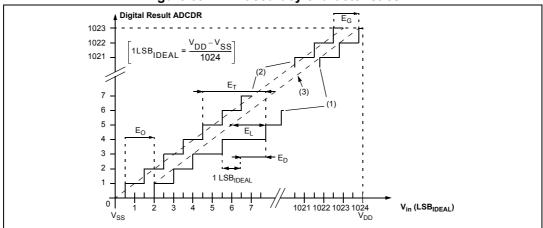
Figure 69. ADC accuracy characteristics
