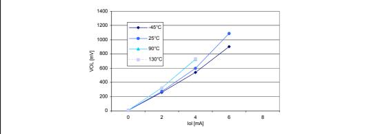
Figure 57. Typical  $V_{OL}$  at  $V_{DD}$  = 5 V (standard pins)
