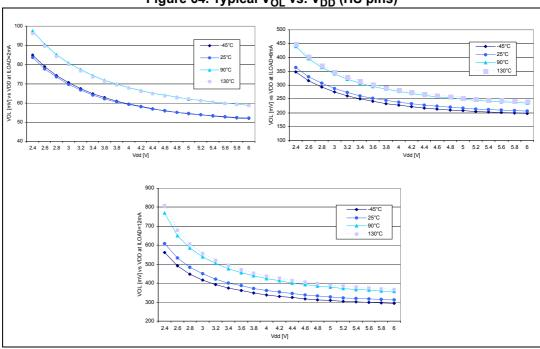
Figure 64. Typical V<sub>OL</sub> vs. V<sub>DD</sub> (HS pins)
