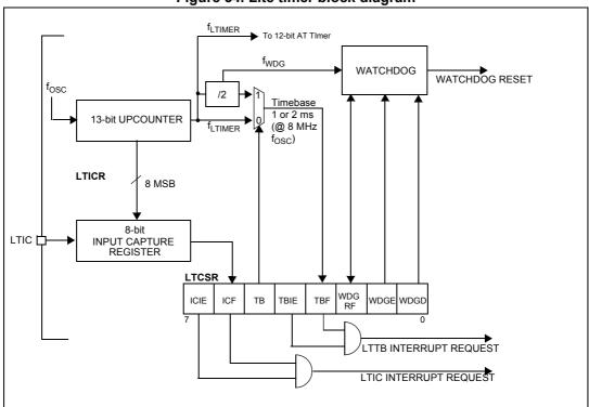
Figure 34. Lite timer block diagram
