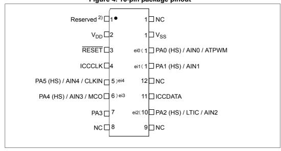
Figure 4. 16-pin package pinout <sup>1</sup>
