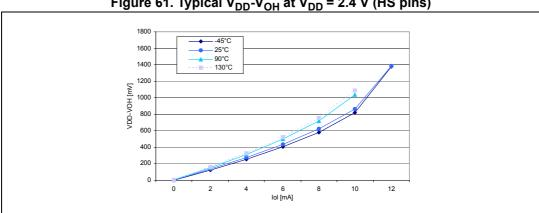
Figure 61. Typical  $V_{DD}$ - $V_{OH}$  at  $V_{DD}$  = 2.4 V (HS pins)
