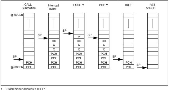
Figure 12. Stack manipulation example
