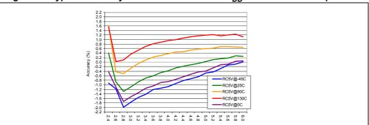
Figure 44. Typical accuracy with RCCR=RCCR0 vs V<sub>DD</sub>= 2.4-6.0 V and temperature
