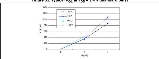
Figure 55. Typical V<sub>OL</sub> at  $v_{DD}$  = 2.4 V (standard pins)
