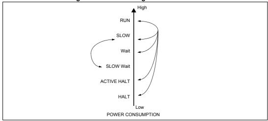
Figure 22. Power saving mode transitions
