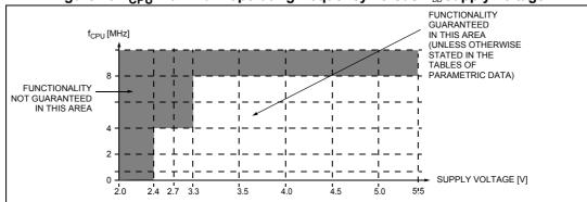
Figure 43. f<sub>CPU</sub> maximum operating frequency versus V<sub>DD</sub> supply voltage
