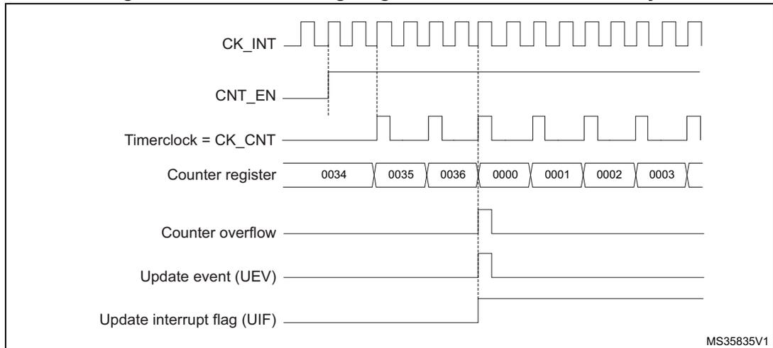
**Figure 159. Counter timing diagram, internal clock divided by 4**
