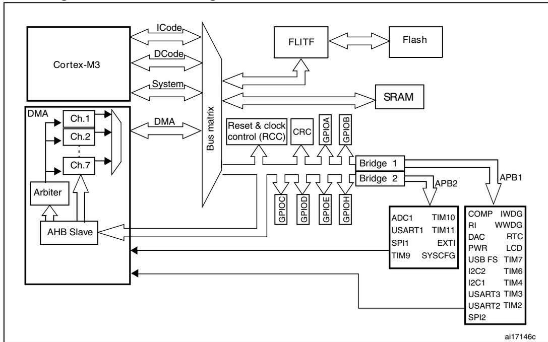
Figure 35. DMA block diagram in Cat.3 STM32L1xxx devices
