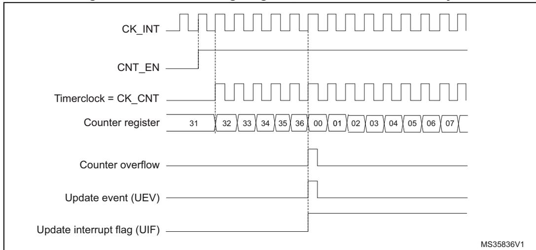
**Figure 88. Counter timing diagram, internal clock divided by 2**
