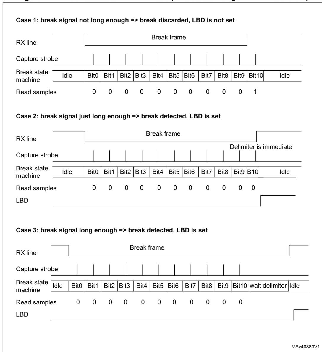
Figure 225. Break detection in LIN mode vs. Framing error detection
