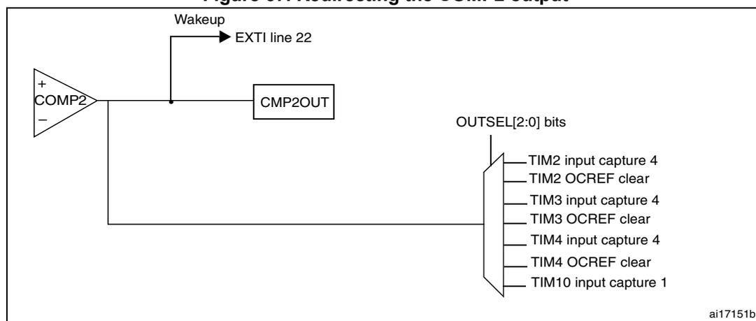
*Note:* For more details about “clearing TIMx OCREF”, refer to [Section 17.3.11: Clearing the OCxREF signal on an external event on page 406](#).
