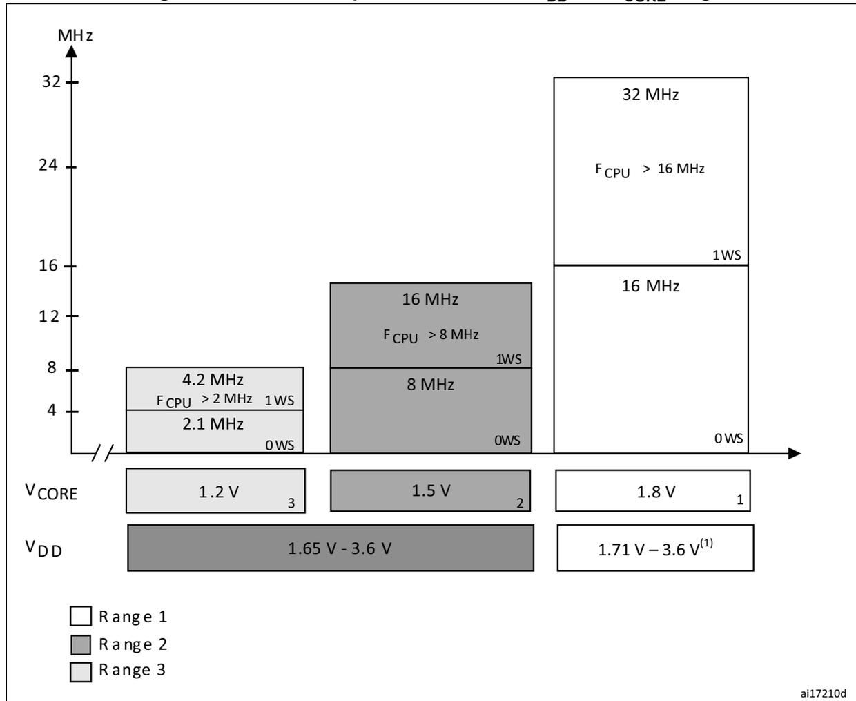
1. Depending on the device, V<sub>DD</sub> range 1 is either 1.71 to 3.6V or 2.0V to 3.6V. Please refer to the specific product datasheet.
