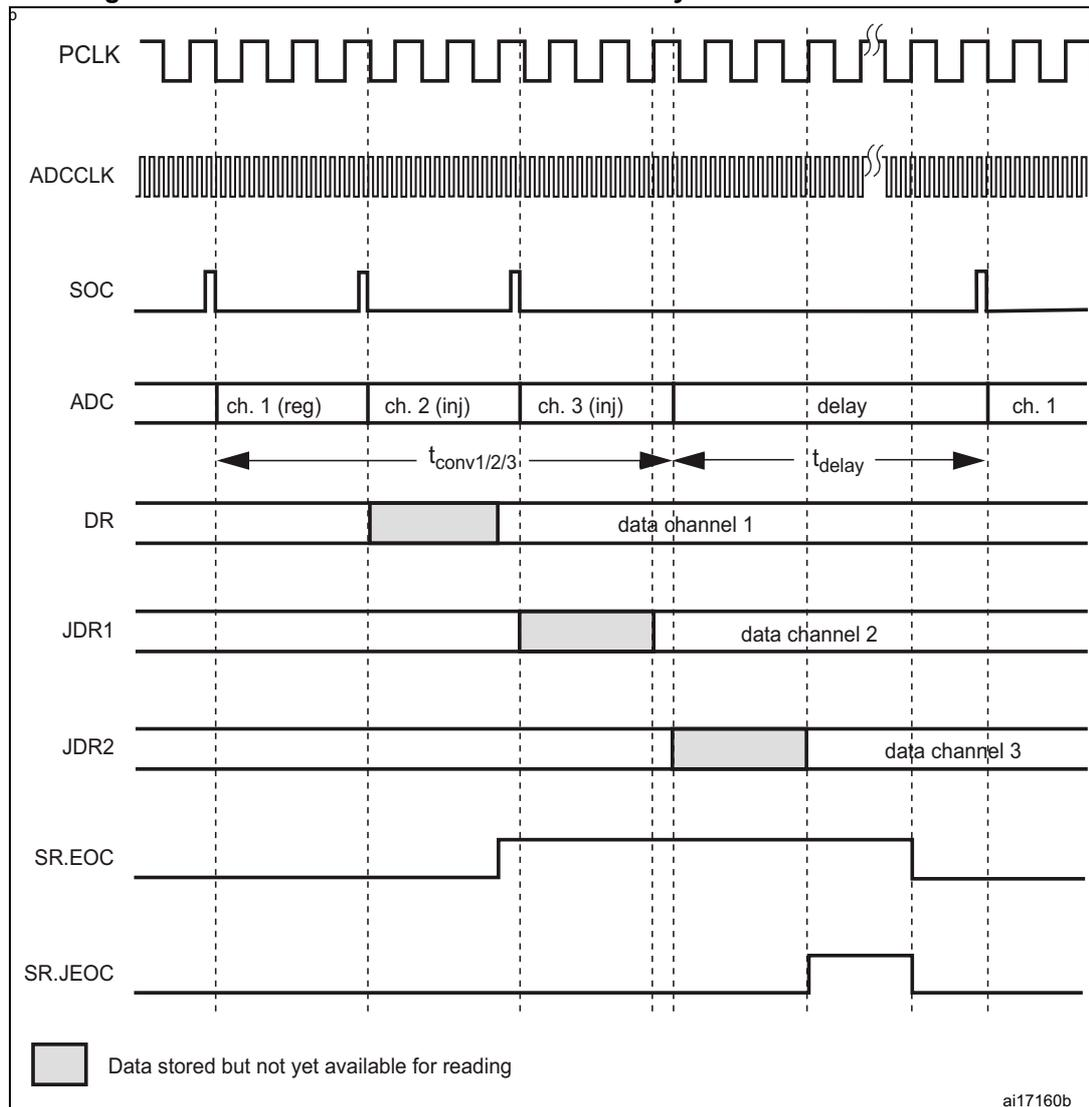
1.  $t_{conv1/2/3}$ : including sampling and conversion times for channels 1, 2 and 3.
