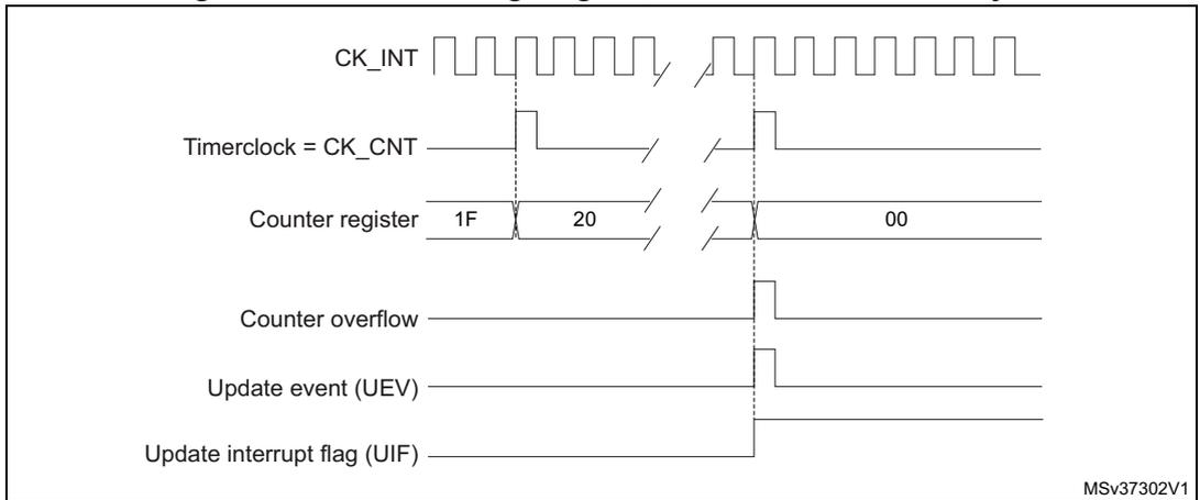
**Figure 91. Counter timing diagram, Update event when ARPE=0 (TIMx\_ARR not preloaded)**
