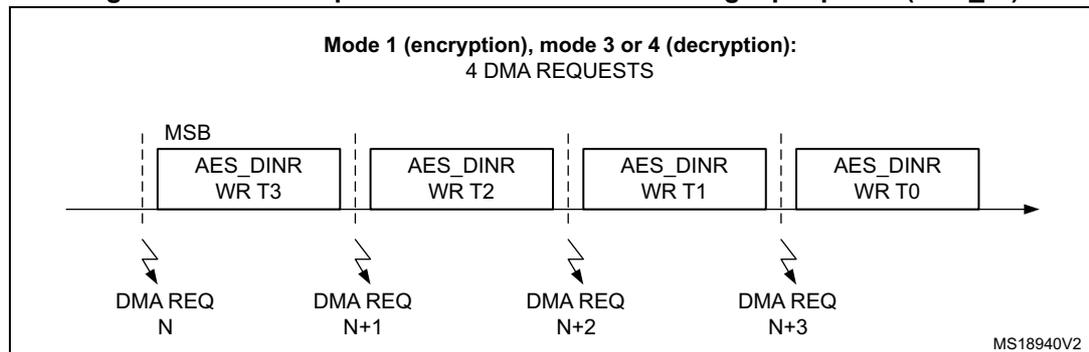
**Figure 185. DMA requests during Output phase (AES\_OUT)**
