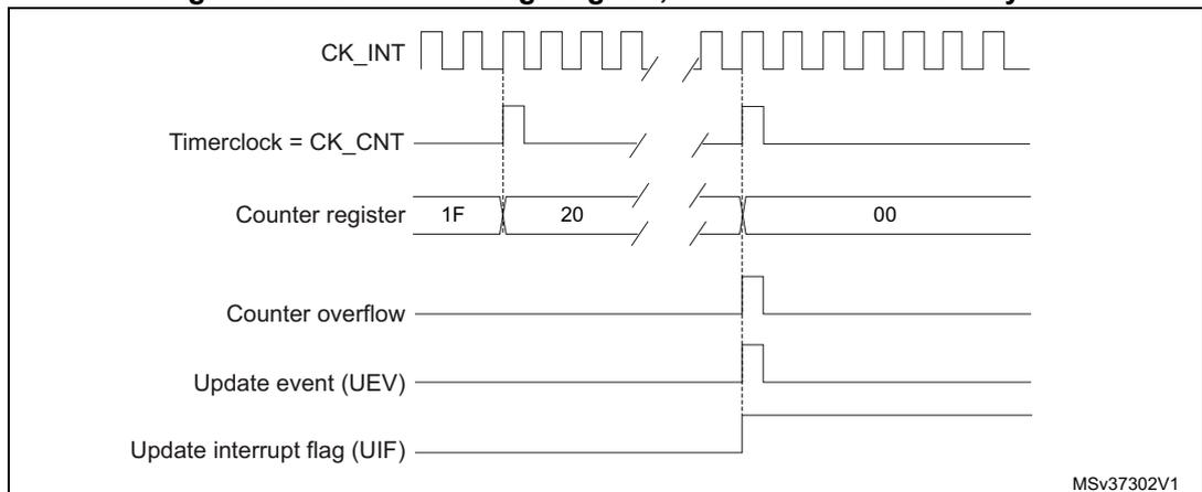
**Figure 161. Counter timing diagram, update event when ARPE=0 (TIMx\_ARR not preloaded)**
