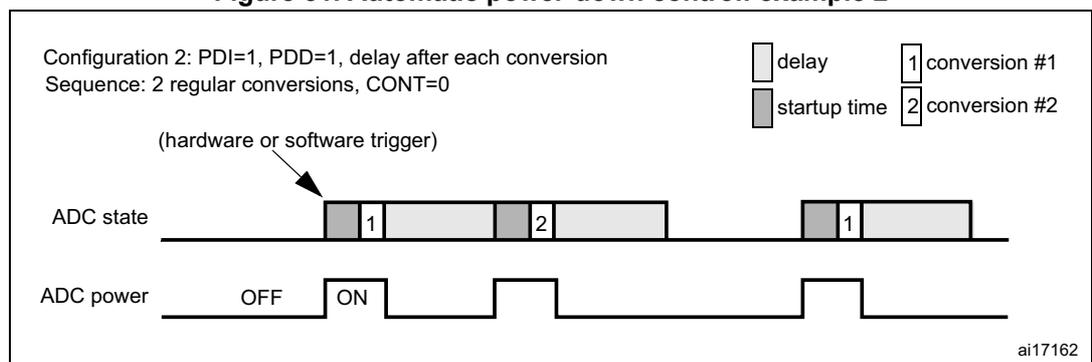
Figure 52. Automatic power-down control: example 3
