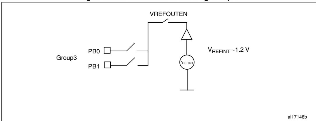
The VREFINT output can be routed to any I/O in group 3 by following this procedure:
