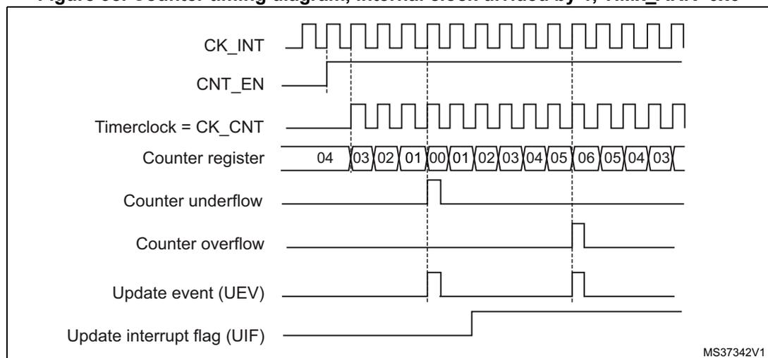
1. Here, center-aligned mode 1 is used, for more details refer to [Section 17.4.1: TIMx control register 1 \(TIMx\\_CR1\)](#).
