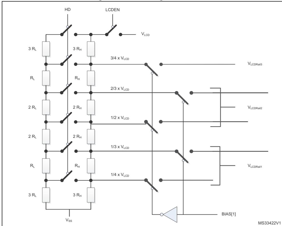
The  $R_L$  divider can be always switched on using the HD bit in the LCD\_FCR configuration register (see [Section 16.5.2](#)). The  $V_{LCD}$  value can be chosen among a wide set of values from  $V_{LCDmin}$  to  $V_{LCDmax}$  by means of CC[2:0] (Contrast Control) bits inside LCD\_FCR (see [Section 16.5.2](#)) register. New values of  $V_{LCD}$  takes effect every beginning of a new frame.
