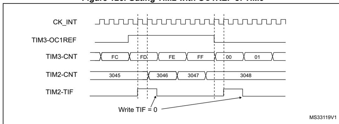
In the example in [Figure 125](#), the TIM2 counter and prescaler are not initialized before being started. So they start counting from their current value. It is possible to start from a given
