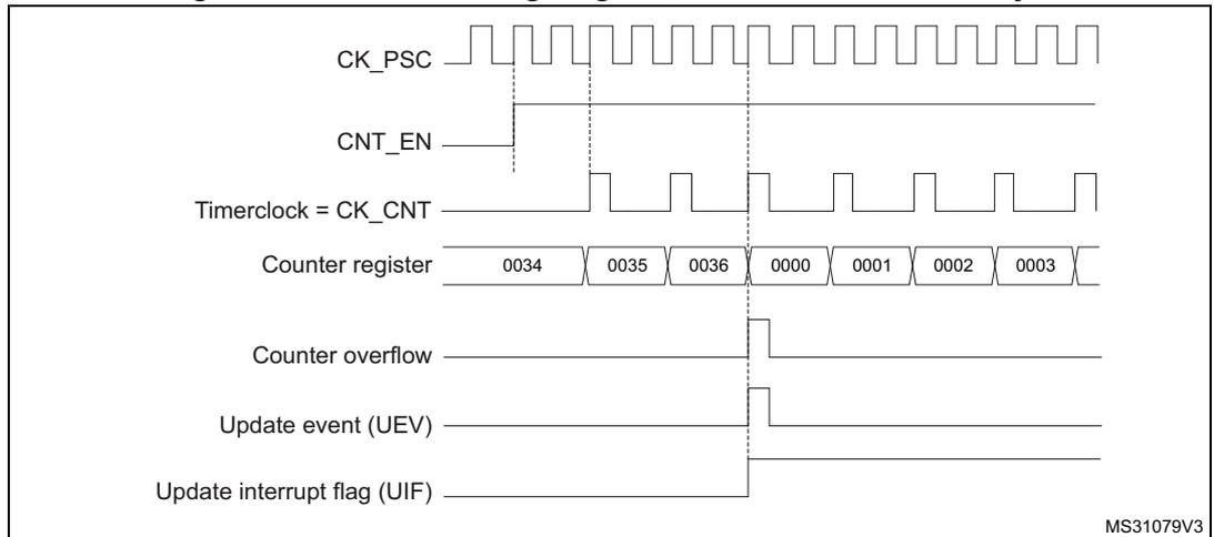
**Figure 137. Counter timing diagram, internal clock divided by 4**
