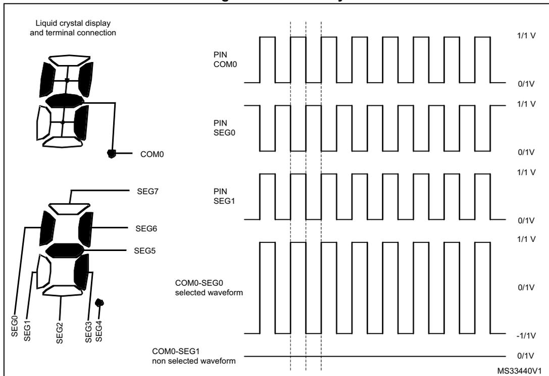
In this mode, the segment terminals are multiplexed and each of them control four pixels. A pixel is activated only when both of its corresponding SEG and COM lines are active in the same phase. In case of 1/4 duty, to deactivate pixel 0 connected to COM[0] the SEG[0] needs to be inactive during the phase 0 when COM[0] is active. To activate pixel44
