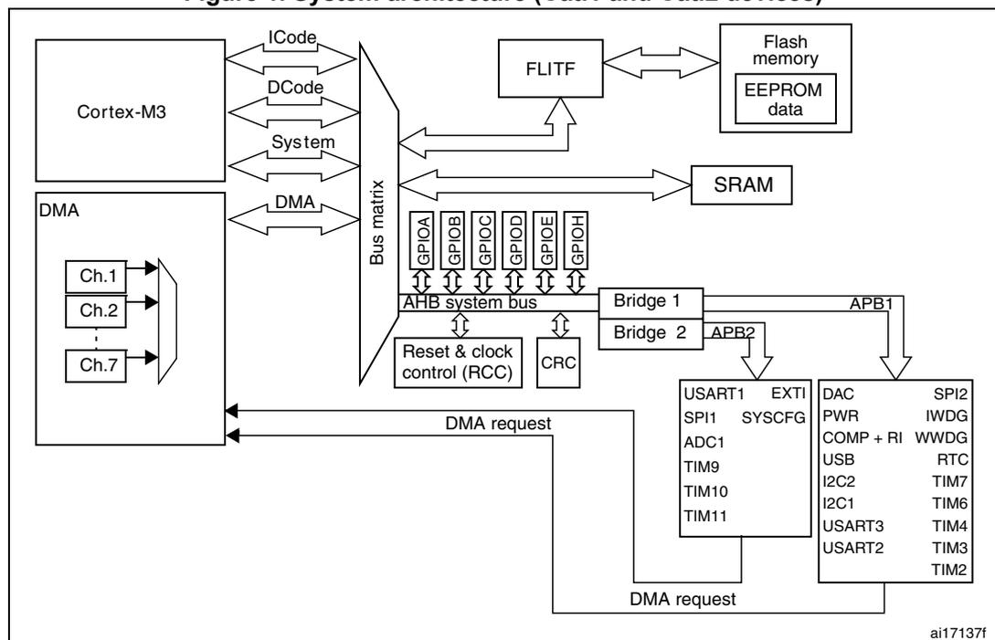
Figure 2. System architecture (Cat.3 devices)
