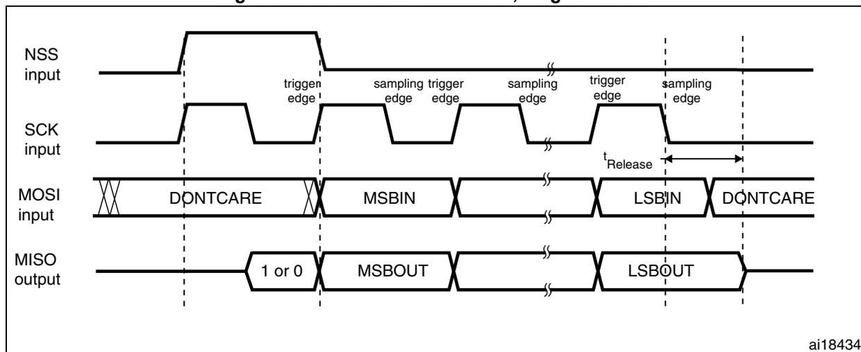
Figure 244. TI mode - Slave mode, continuous transfer
