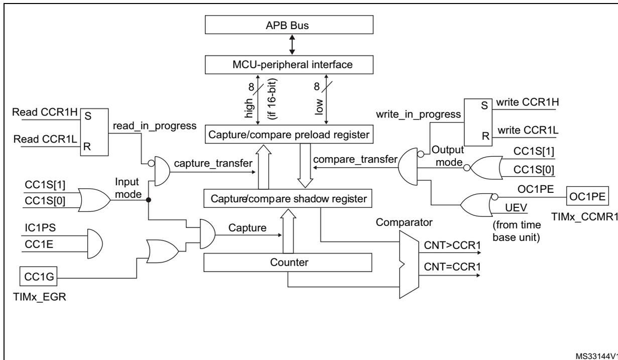
Figure 111. Output stage of capture/compare channel (channel 1)
