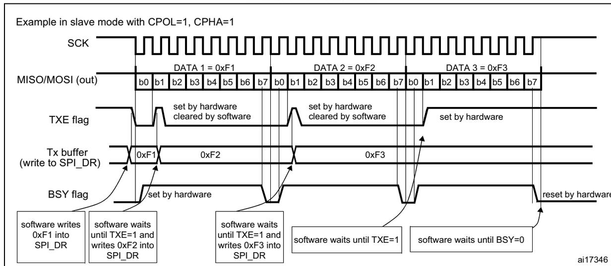
**Bidirectional transmit procedure (BIDIMODE=1 and BIDIOE=1)**
