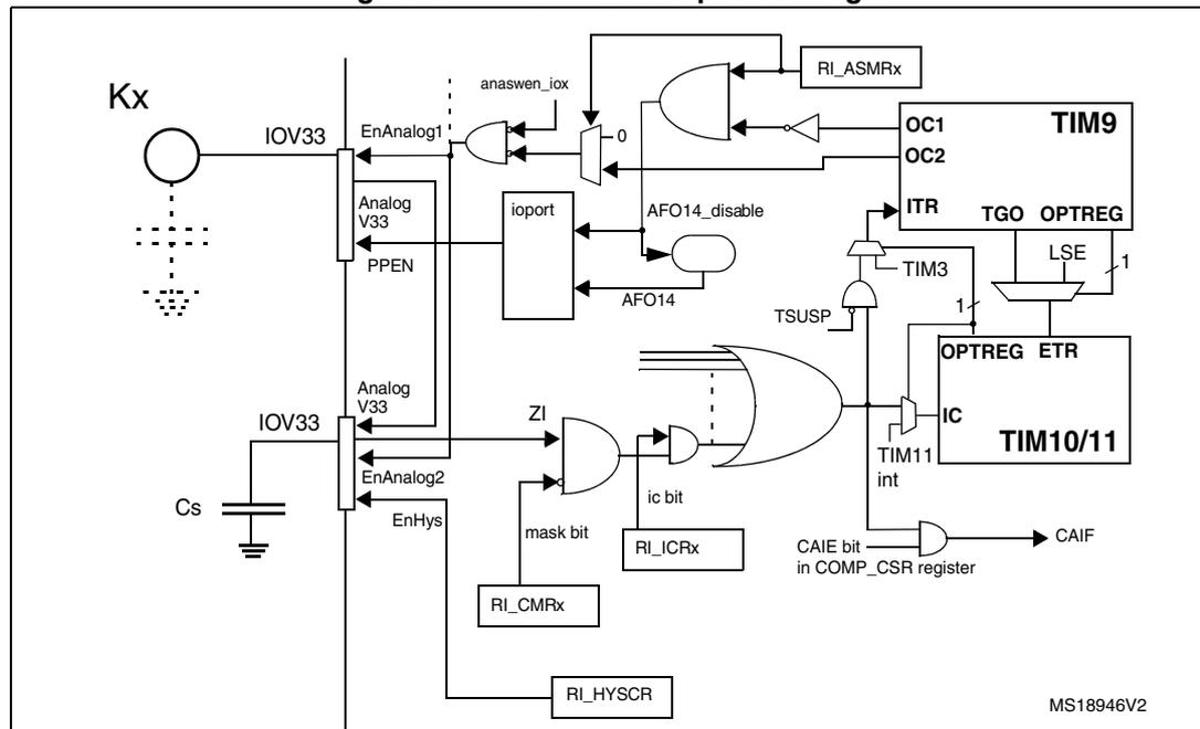
Both timers are used to manage the GPIO port toggling which dramatically reduces the CPU load. TIM9 handles the charge transfer sequence generation by directly controlling the channel and sampling capacitor I/Os. TIM10 or 11 count the number of charge transfer cycles generated before an end of acquisition is detected on one of the enabled analog I/O groups.
