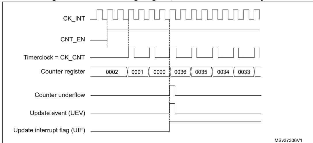
**Figure 95. Counter timing diagram, internal clock divided by 4**
