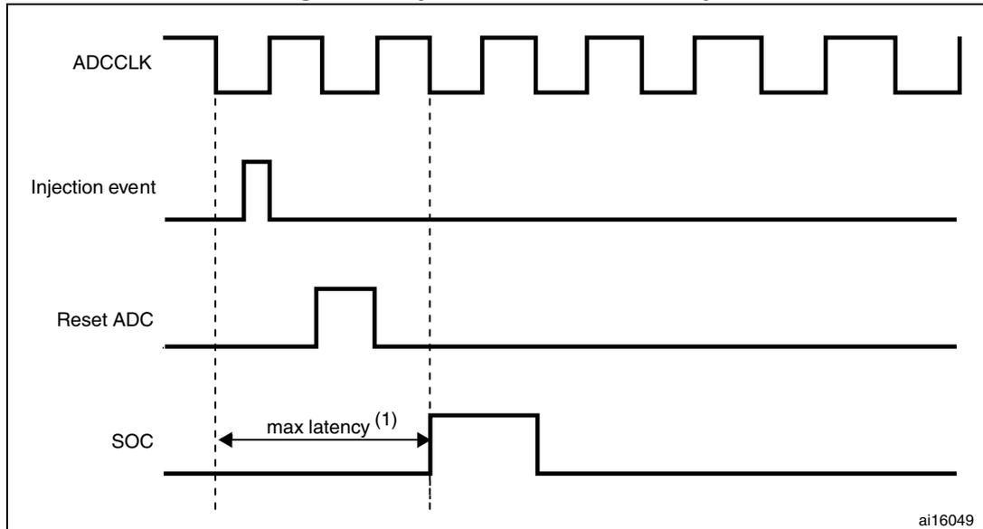
1. The maximum latency value can be found in the electrical characteristics of the STM32L1xxxx datasheet.
