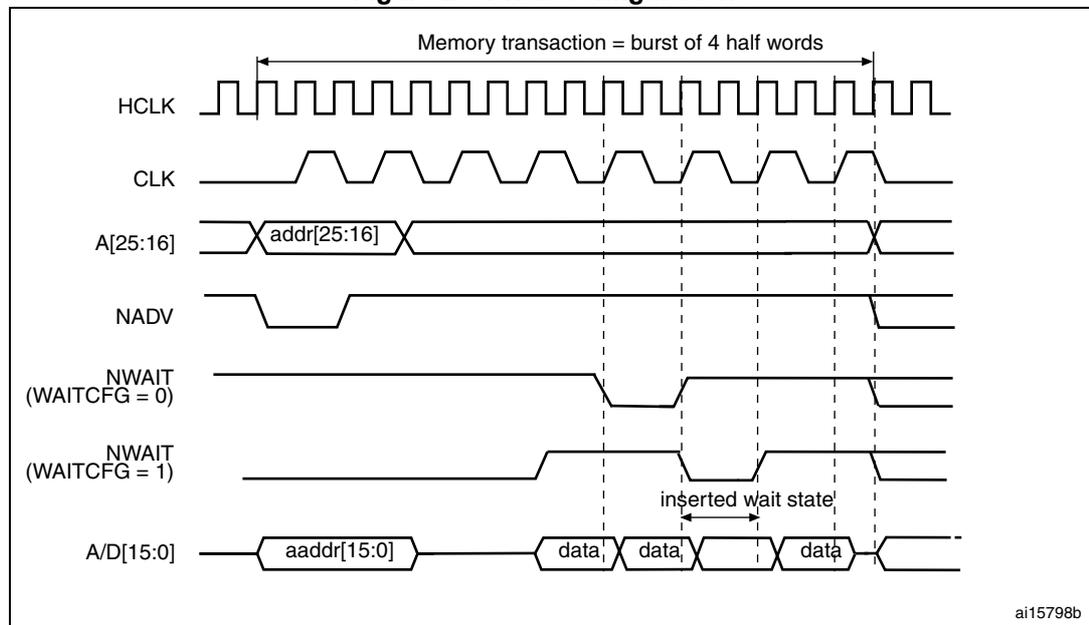
**Figure 206. Synchronous multiplexed read mode - NOR, PSRAM (CRAM)**
