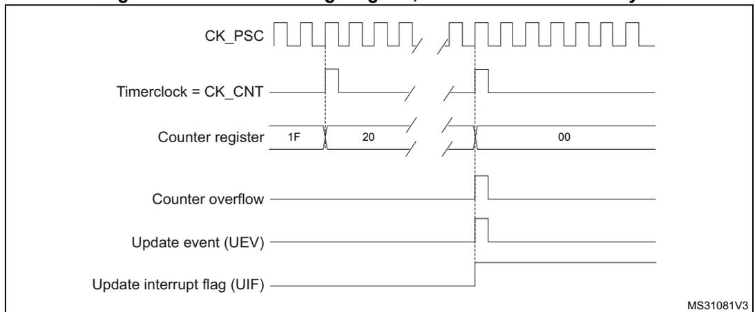
**Figure 139. Counter timing diagram, update event when ARPE=0 (TIMx\_ARR not preloaded)**
