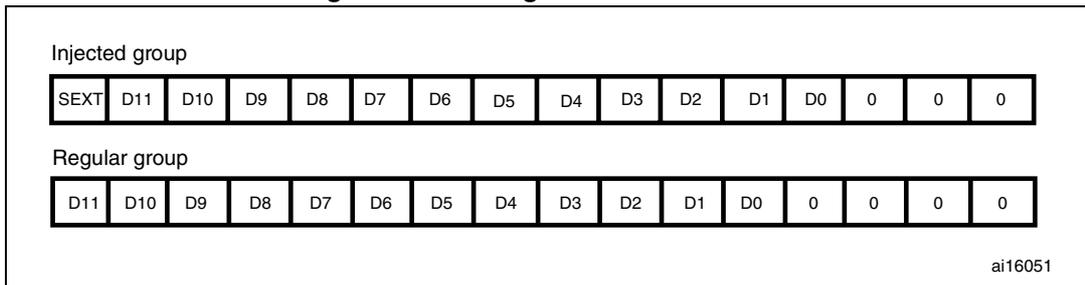
Special case: when left-aligned, the data are aligned on a half-word basis except when the resolution is set to 6-bit. In that case, the data are aligned on a byte basis as shown in [Figure 46](#).
