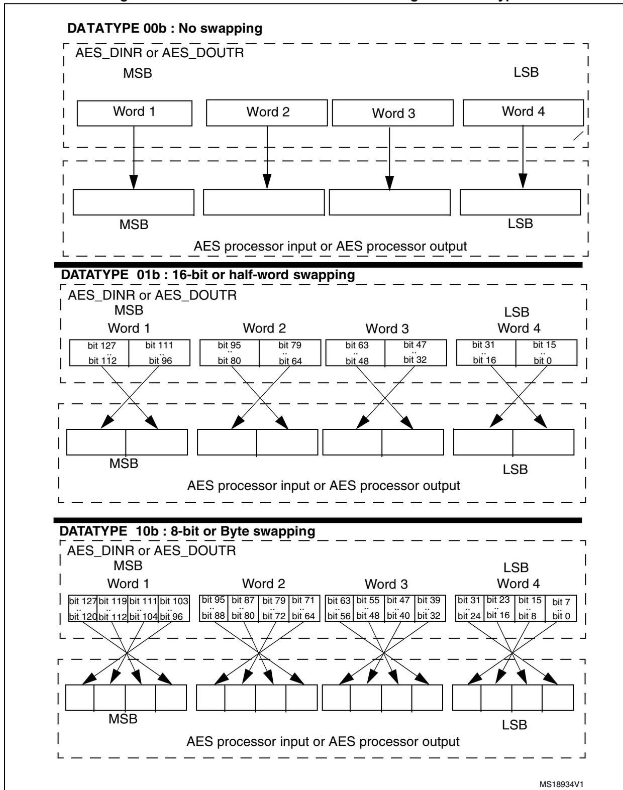
Figure 179. 128-bit block construction according to the data type (continued)
