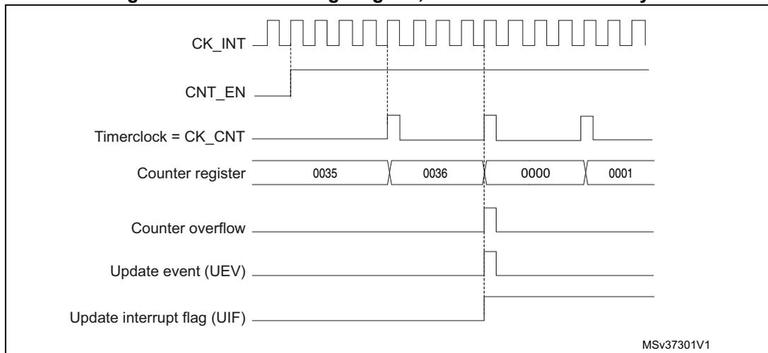
**Figure 90. Counter timing diagram, internal clock divided by N**
