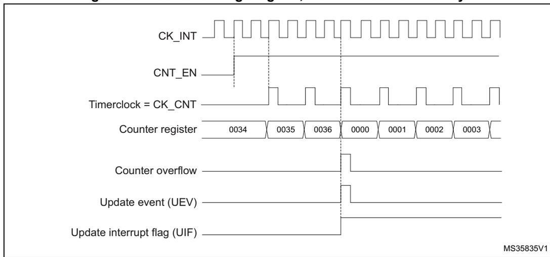
**Figure 89. Counter timing diagram, internal clock divided by 4**
