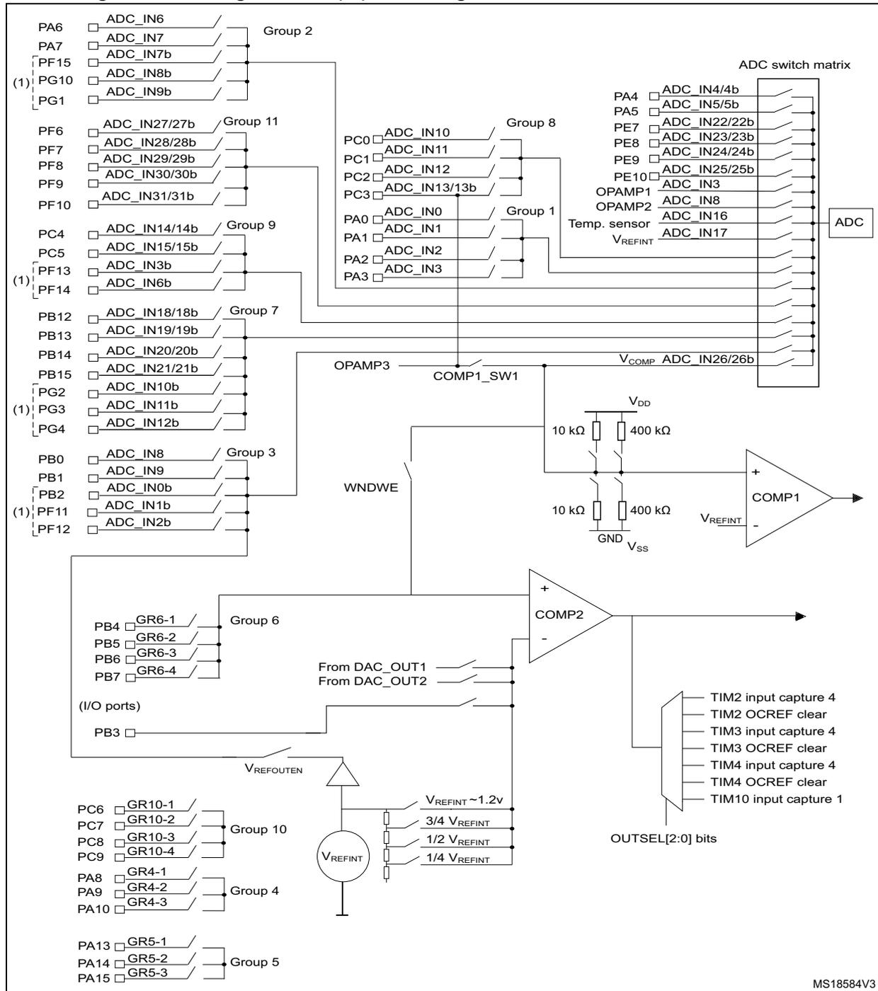
1. These I/O pins cannot be used as COMP1 inputs.
