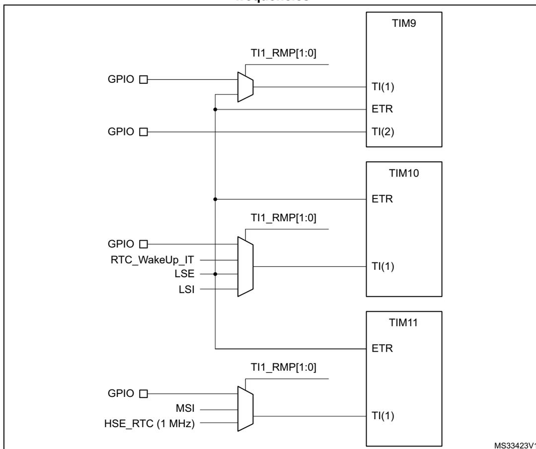
Each timer has an input multiplexer that selects which of the I/O or the internal clock is to trigger the input capture. This selection is performed through the TI1\_RMP [1:0] bits in the TIMx\_OR register.
