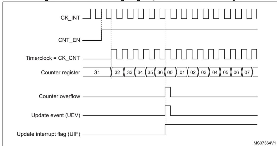
**Figure 158. Counter timing diagram, internal clock divided by 2**
