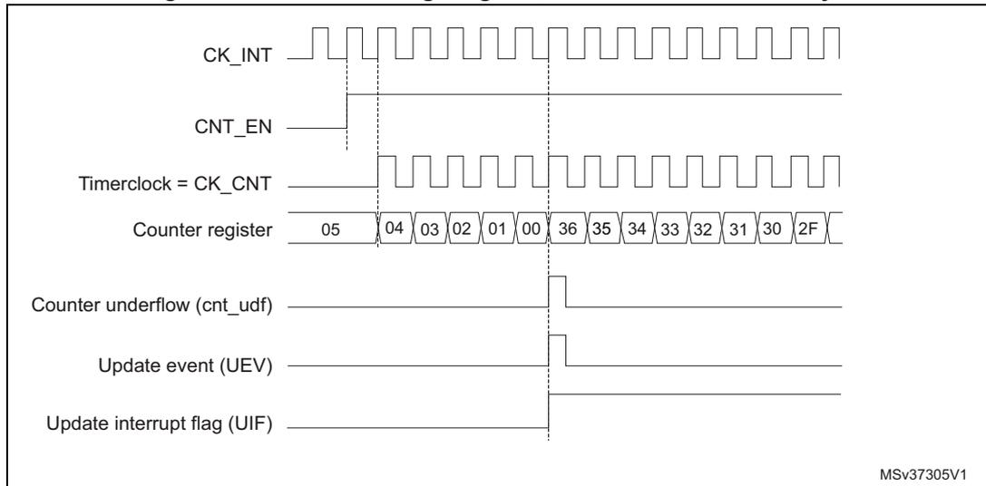
**Figure 94. Counter timing diagram, internal clock divided by 2**
