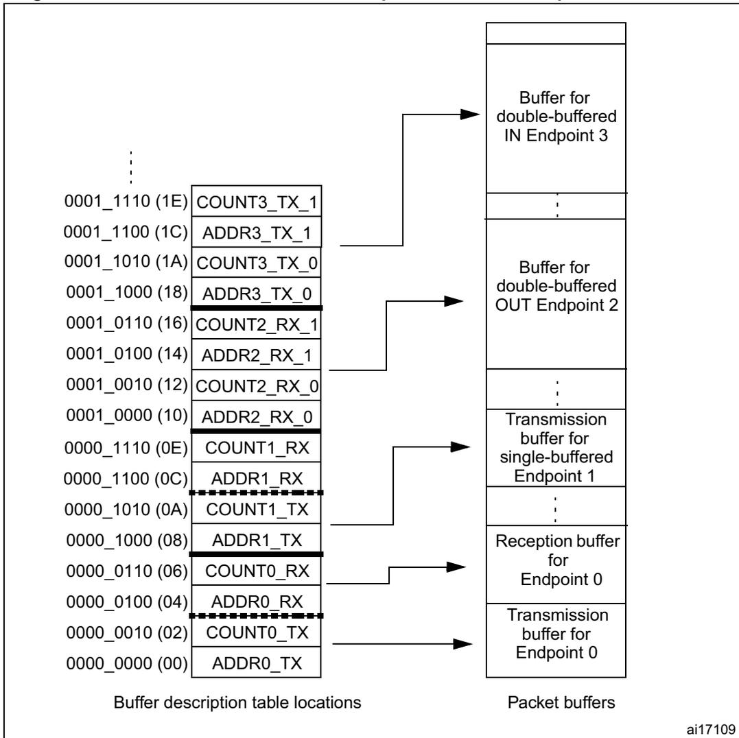
Each packet buffer is used either during reception or transmission starting from the bottom. The USB peripheral will never change the contents of memory locations adjacent to the allocated memory buffers; if a packet bigger than the allocated buffer length is received (buffer overrun condition) the data will be copied to the memory only up to the last available location.
