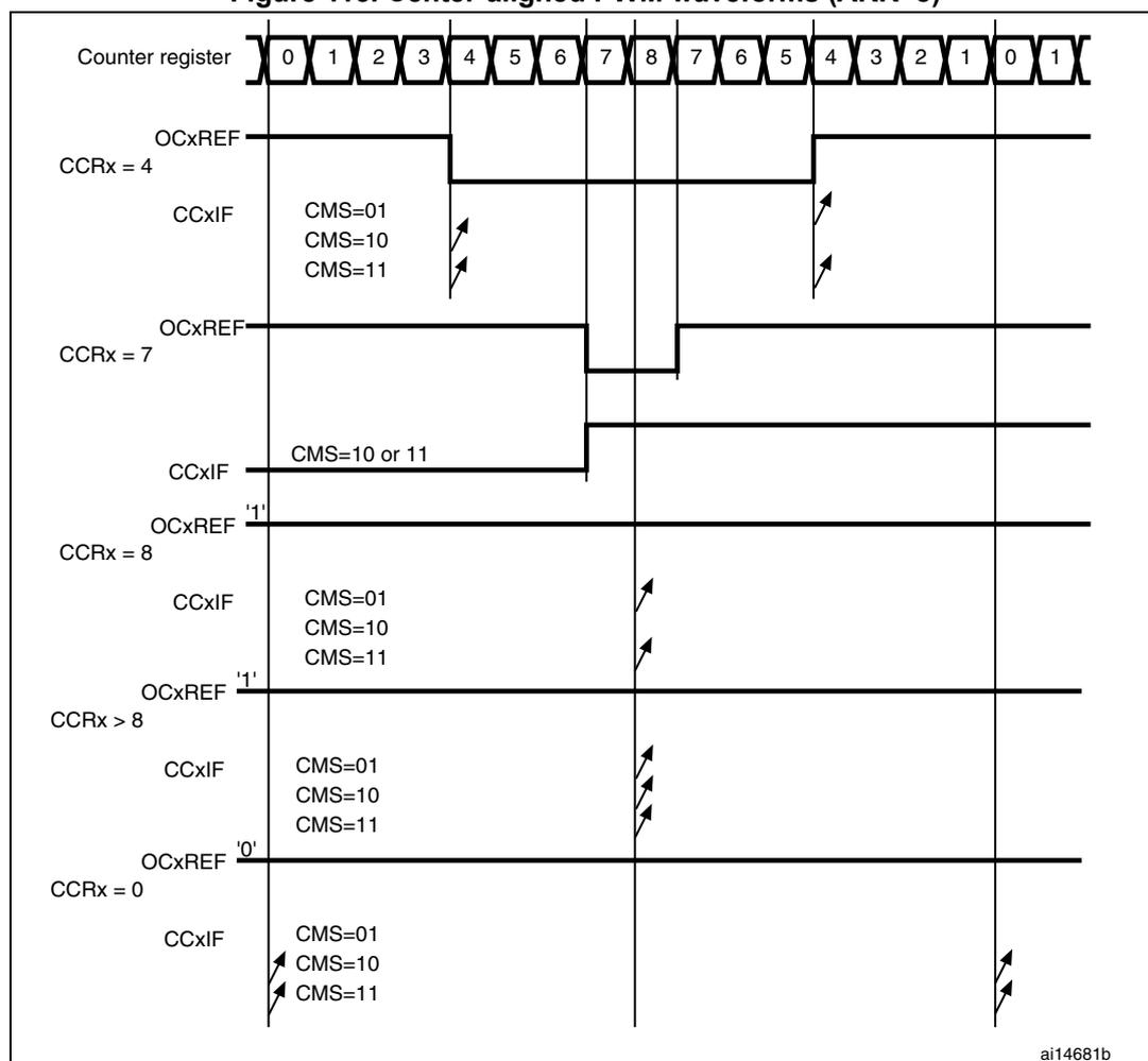
Hints on using center-aligned mode:
