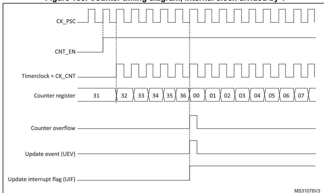
**Figure 136. Counter timing diagram, internal clock divided by 2**
