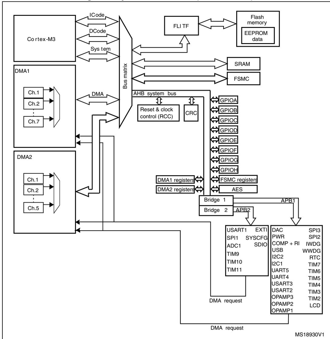
Figure 4. System architecture (Cat.5 and Cat.6 devices)
