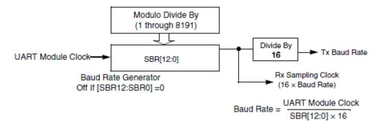
Figure 2. UART baud rate generation
