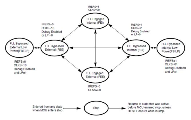
Figure 1. ICS clocking switching modes
