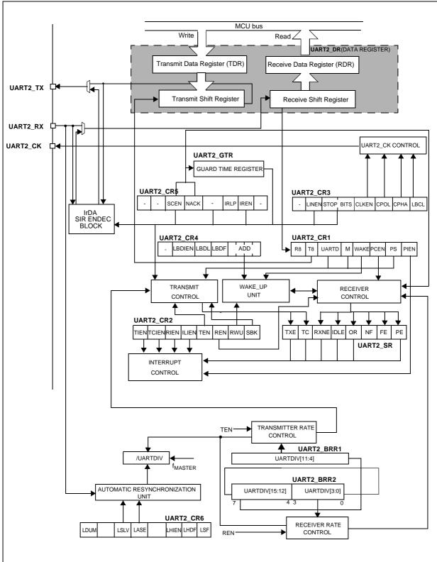
Figure 111. UART2 block diagram
