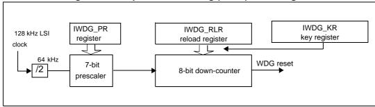
Figure 27. Independent watchdog (IWDG) block diagram
