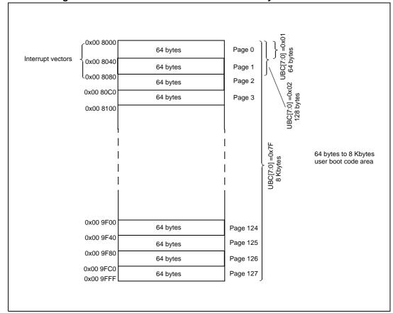
Figure 9. UBC area size definition on low density STM8S devices
