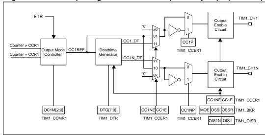
Figure 68. Detailed output stage of channel with complementary output (channel 1)
