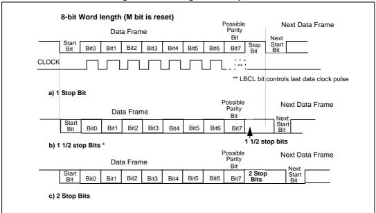
Figure 115. Configurable stop bits
