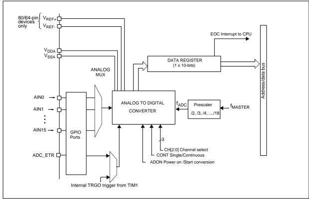
Figure 160. ADC2 block diagram
