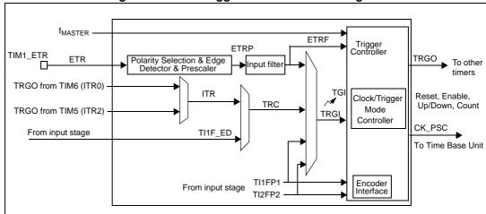
Figure 43. Clock/trigger controller block diagram
