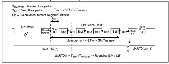
Figure 135. LIN synch field measurement
