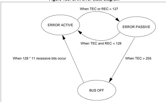
Figure 153. CAN error state diagram
