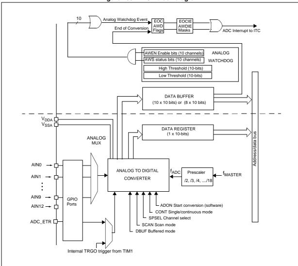
Figure 159. ADC1 block diagram
