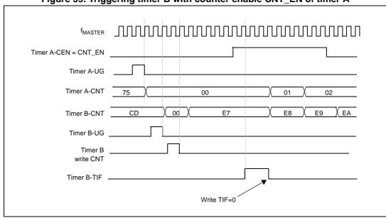
Figure 59. Triggering timer B with counter enable CNT\_EN of timer A
