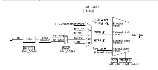
Figure 45. Tl2 external clock connection example
