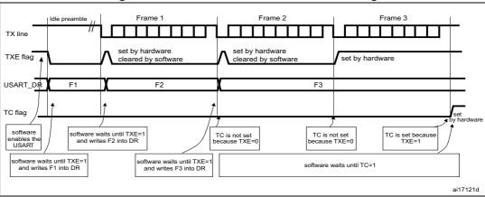
Figure 116. TC/TXE behavior when transmitting
