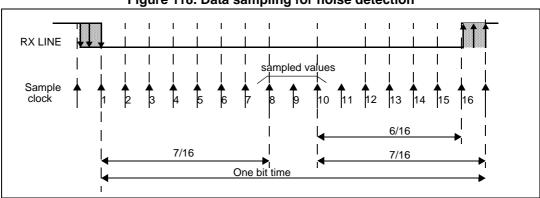
Figure 118. Data sampling for noise detection
