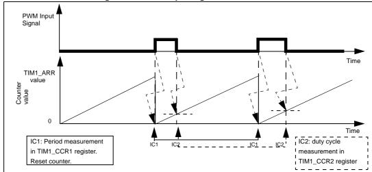
Figure 65. PWM input signal measurement
