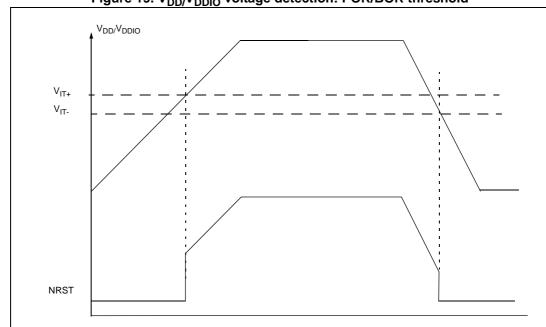
Figure 19. V<sub>DD/</sub>V<sub>DDIO</sub> voltage detection: POR/BOR threshold
