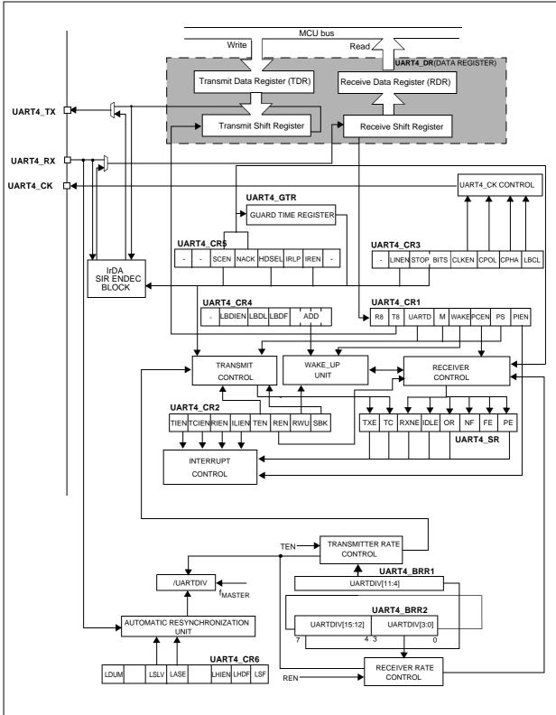
Figure 113. UART4 block diagram
