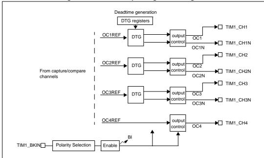
Figure 67. Channel output stage block diagram
