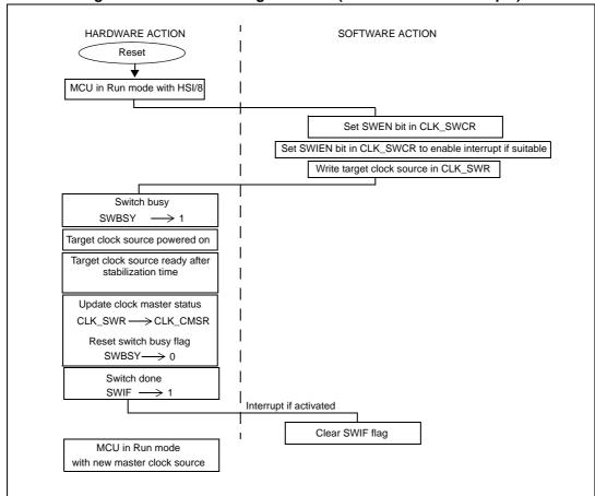
Figure 22. Clock switching flowchart (automatic mode example)
