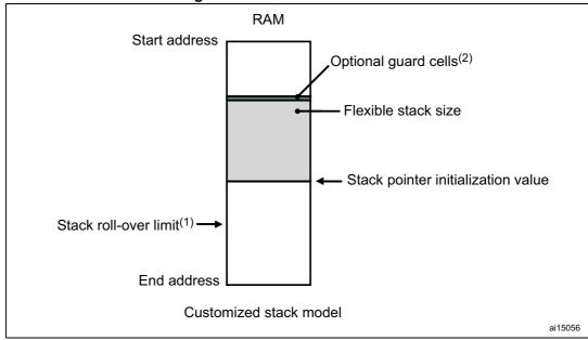
Figure 5. Customized stack model
