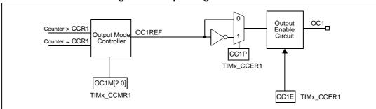
Figure 88. Output stage of channel 1
