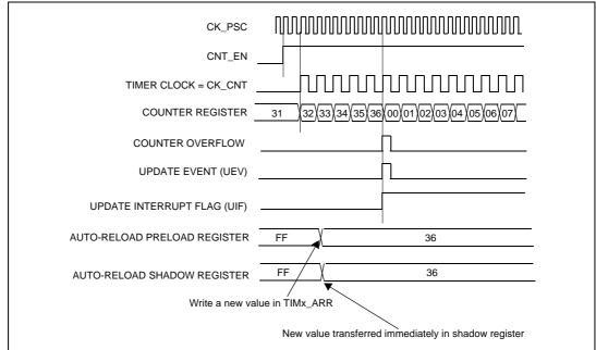
Figure 35. Counter update when ARPE = 0 (ARR not preloaded) with prescaler = 2
