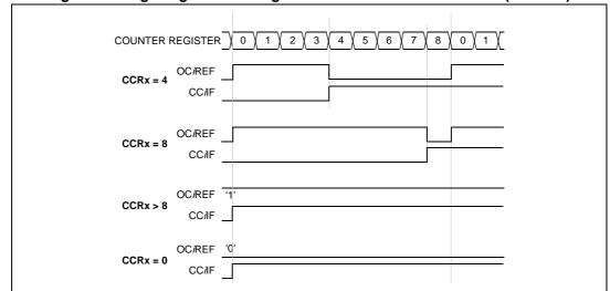
Figure 70. Edge-aligned counting mode PWM mode 1 waveforms (ARR = 8)
