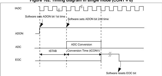
Figure 162. Timing diagram in single mode (CONT = 0)
