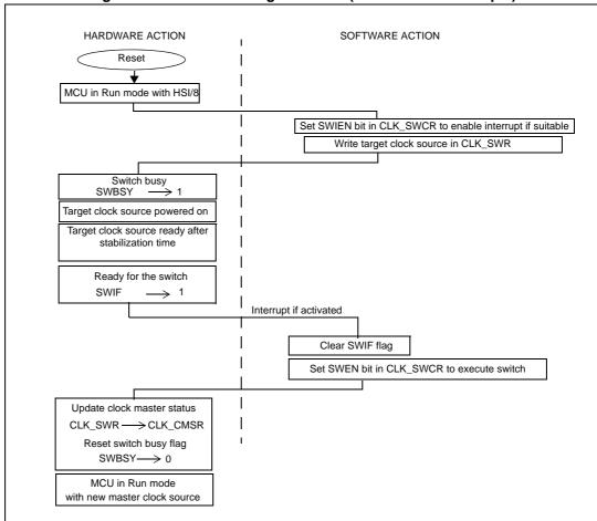
Figure 23. Clock switching flowchart (manual mode example)
