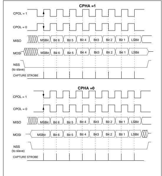
Figure 93. Data clock timing diagram
