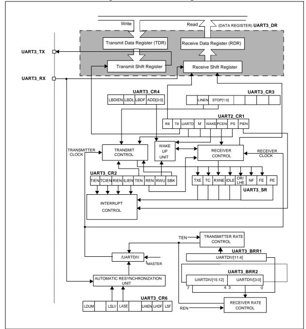
Figure 112. UART3 block diagram
