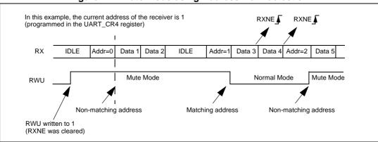
Figure 121. Mute mode using Address mark detection
