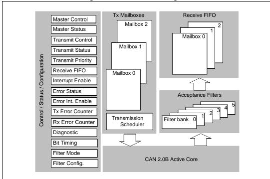
Figure 141. beCAN block diagram
