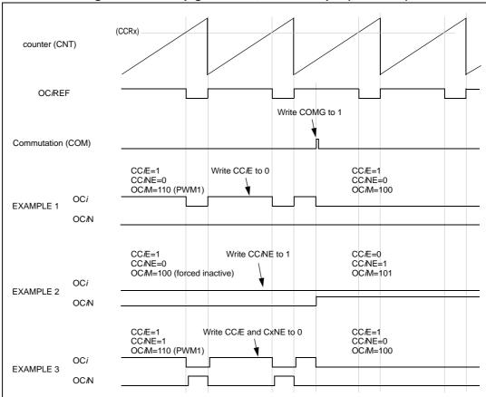
Figure 76. Six-step generation, COM example (OSSR = 1)
