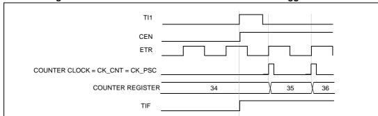
Figure 52. Control circuit in external clock mode 2 + trigger mode
