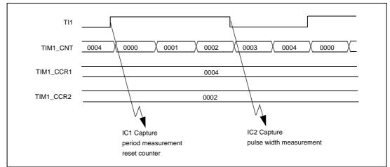
Figure 66. PWM input signal measurement example
