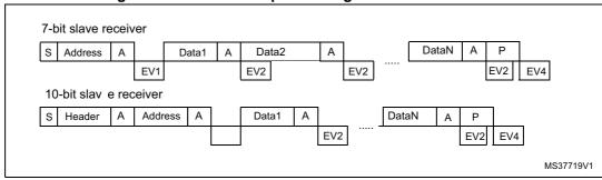
Figure 103. Transfer sequence diagram for slave receiver
