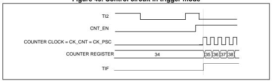
Figure 49. Control circuit in trigger mode
