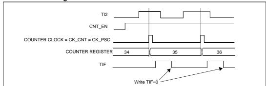
Figure 46. Control circuit in external clock mode 1
