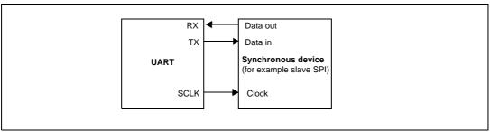
Figure 123. UART data clock timing diagram (M=0)
