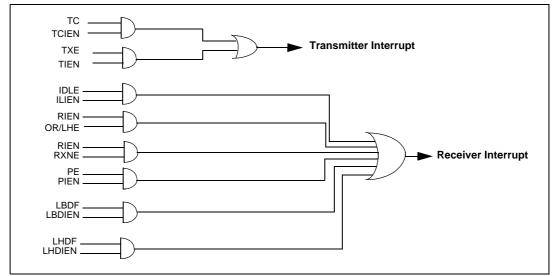
Figure 139. UART interrupt mapping diagram
