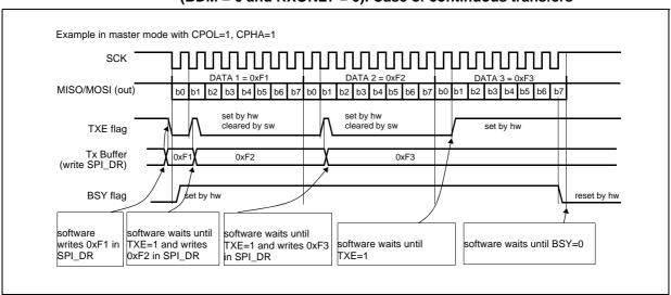
Figure 96. TXE/BSY in master transmit-only mode (BDM = 0 and RXONLY = 0). Case of continuous transfers
