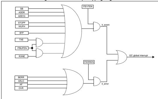
Figure 109. I<sup>2</sup>C interrupt mapping diagram
