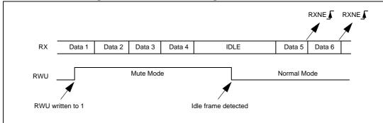
Figure 120. Mute mode using idle line detection
