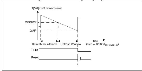
Figure 30. Window watchdog timing diagram
