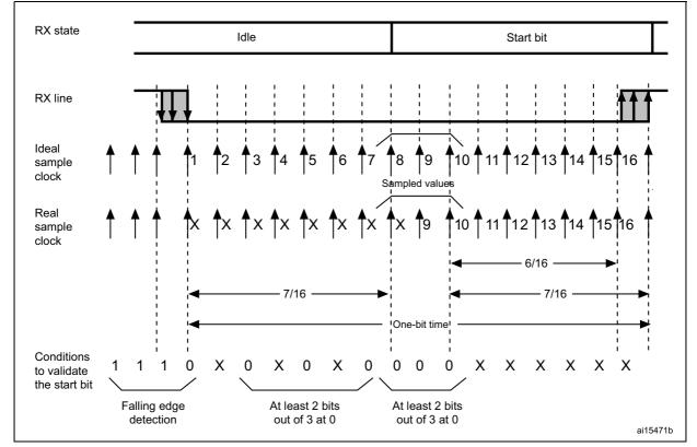
Figure 117. Start bit detection
