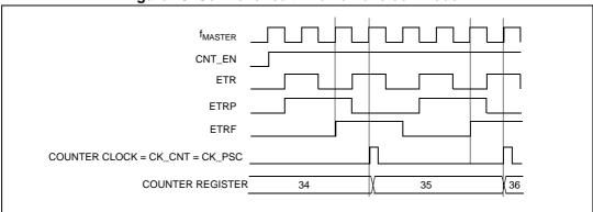
Figure 48. Control circuit in external clock mode 2
