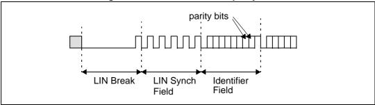
The bits involved are the two MSB positions (7th and 8th bits) of the identifier character. The check is performed as specified by the LIN specification:
