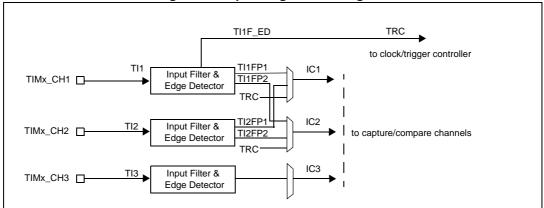
Figure 86. Input stage of TIM 2 channel 1
