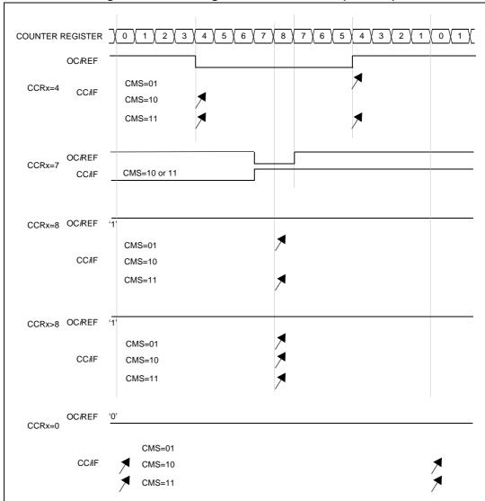
Figure 71. Center-aligned PWM waveforms (ARR = 8)
