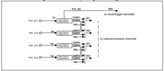
Figure 64 shows how the input stage samples the corresponding TIi input to generate a filtered signal TIiF. Then, an edge detector with polarity selection, generates a signal (TIiFPn) which can be used as trigger input by the clock/trigger controller or as the capture command. The signal is prescaled before entering the capture register (ICiPS).
