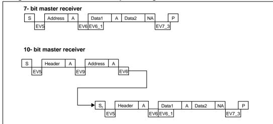
Figure 107. Method 2: transfer sequence diagram for master receiver when N=2
