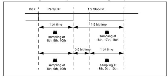
Figure 127. Parity error detection using 1.5 stop bits
