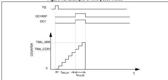
Figure 72. Example of one-pulse mode
