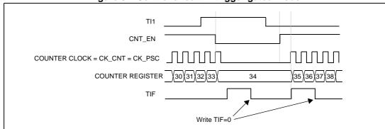
Figure 51. Control circuit in trigger gated mode
