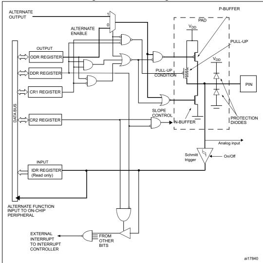
Figure 24. GPIO block diagram
