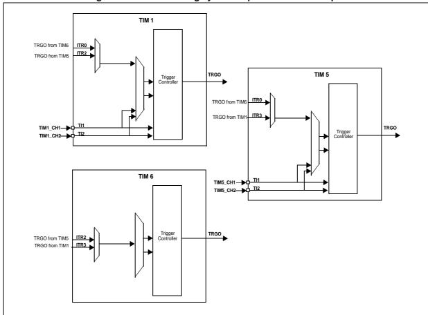
Figure 53. Timer chaining system implementation example
