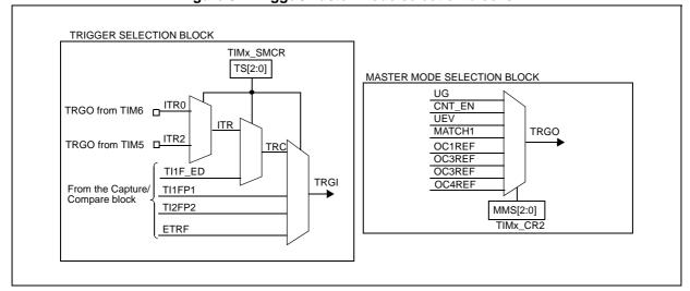
Figure 54. Trigger/master mode selection blocks
