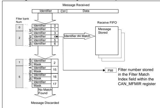
Figure 152. Filter banks configured as in the example in *Table 65*
