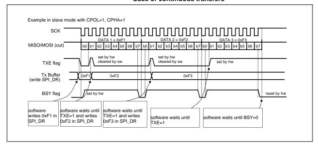
Figure 97. TXE/BSY in slave transmit-only mode (BDM = 0 and RXONLY = 0).
