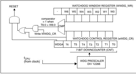
Figure 28. Watchdog block diagram
