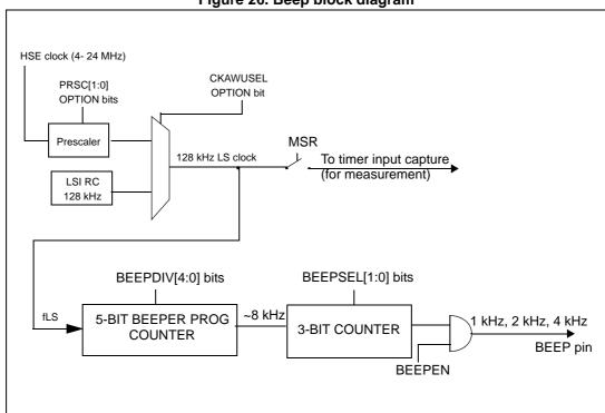
Figure 26. Beep block diagram
