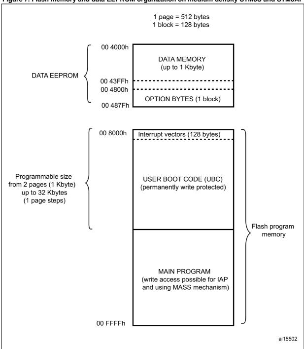
The memory mapping is given for the STM8AF devices featuring 32 Kbytes of Flash program memory and 1 Kbytes of SRAM.
