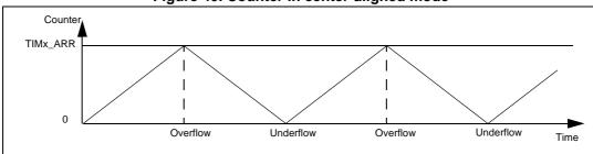
Figure 40. Counter in center-aligned mode
