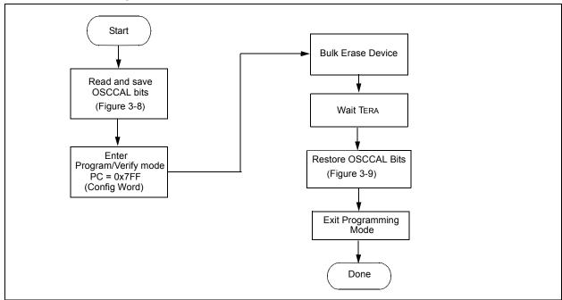
FIGURE 3-13: PROGRAM FLOWCHART – ERASE PROGRAM MEMORY, CONFIGURATION WORD AND USER ID
