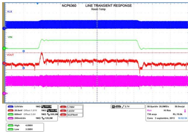
Figure 31. Line Transient Response < 20\ \text{mV} Peak, PV_{IN} = 3.6\text{ V to }4.1\text{ V} , R_L = 8\ \Omega , V_{OUT} = 1.8\text{ V}
