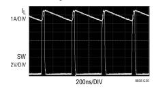
$36V_{IN}$  TO  $3.3V_{OUT}$  AT 1A 2MHz
