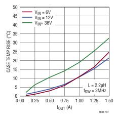
Figure 7. Case Temperature Rise vs Load Current
