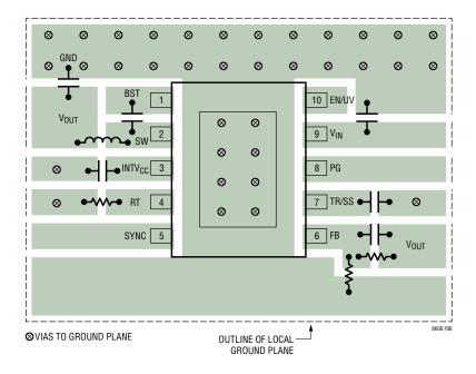
Figure 6. PCB Layout (Not to Scale)
