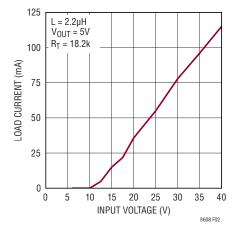
Figure 2. Full Switching Frequency Minimum Load vs V<sub>IN</sub> in Pulse Skipping Mode
