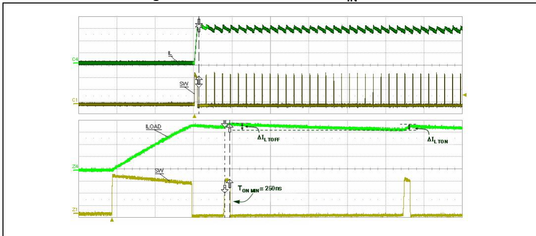
Figure 20. Short-circuit current V_{IN} = 24\text{ V}
