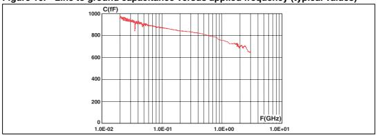
Figure 10. Line to ground capacitance versus applied frequency (typical values)
