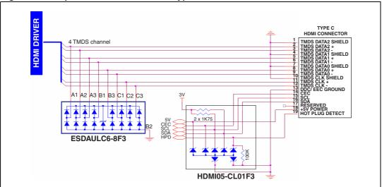
Figure 11. Implementation with HDMI type C connector
