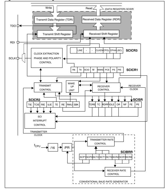
Figure 88. SCI block diagram
