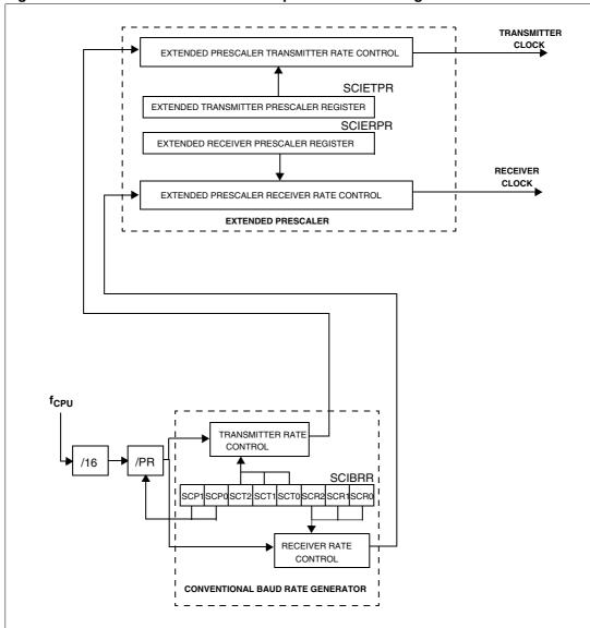
Figure 90. SCI baud rate and extended prescaler block diagram
