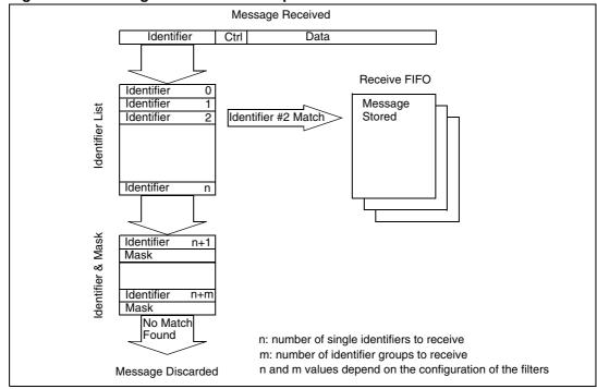
Figure 103. Filtering mechanism - example
