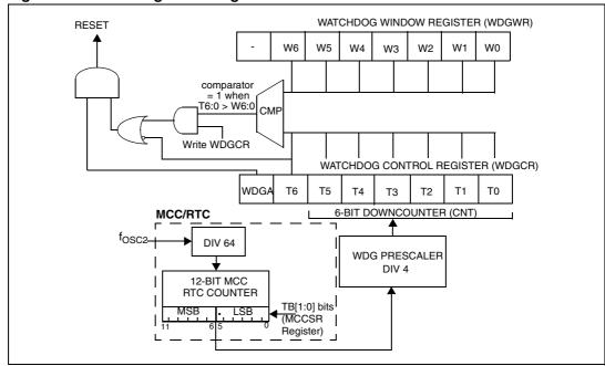
Figure 34. Watchdog block diagram
