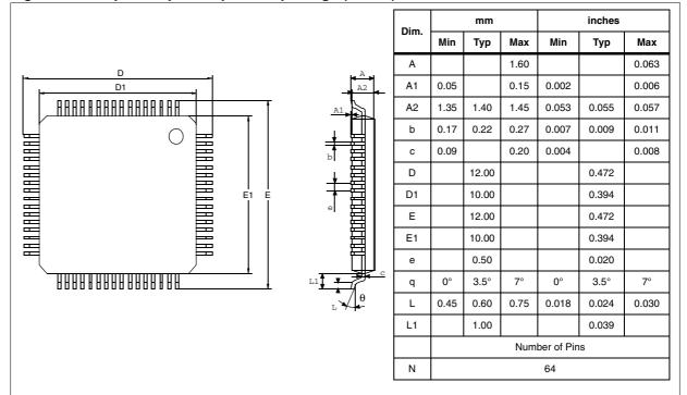
Figure 150. 64-pin low profile quad flat package (10 x10)
