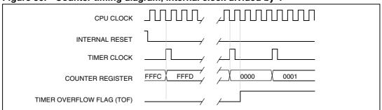
Figure 51. Counter timing diagram, internal clock divided by 8
