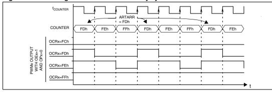
Figure 42. PWM signal from 0% to 100% duty cycle
