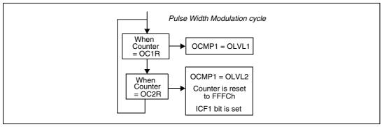
If OLVL1 = 1 and OLVL2 = 0 the length of the positive pulse is the difference between the OC2R and OC1R registers.
