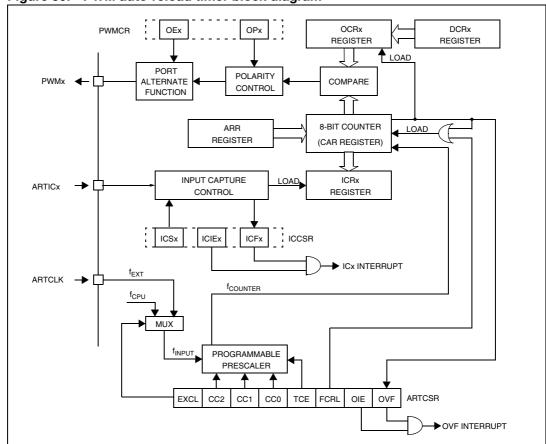
Figure 39. PWM auto-reload timer block diagram
