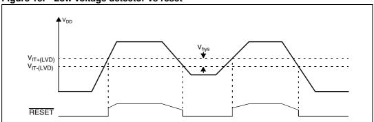
Figure 15. Low voltage detector vs reset
