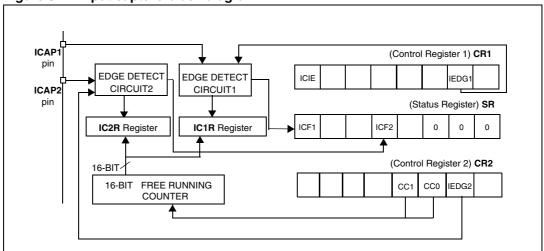
Figure 52. Input capture block diagram
