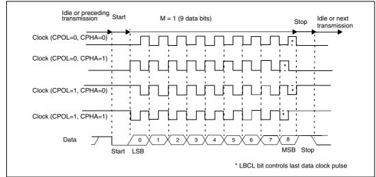
Figure 93. SCI data clock timing diagram (M = 1)
