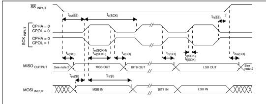
Figure 139. SPI slave timing diagram with CPHA = 0
