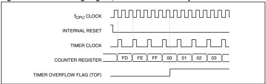
Figure 61. Counter timing diagram, internal clock divided by 4
