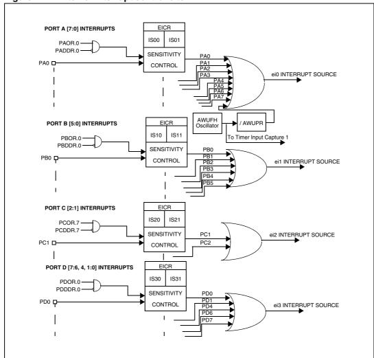
Figure 21. External interrupt control bits
