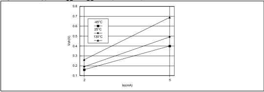
Figure 130. Typical  $V_{OL}$  at  $V_{DD} = 5V$  (high-sink)
