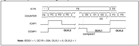
Figure 69. Pulse width modulation mode timing example
