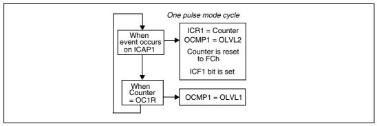
Then, on a valid event on the ICAP1 pin, the counter is initialized to FCh and OLVL2 bit is loaded on the OCMP1 pin, the ICF1 bit is set and the value FFFDh is loaded in the IC1R register.
