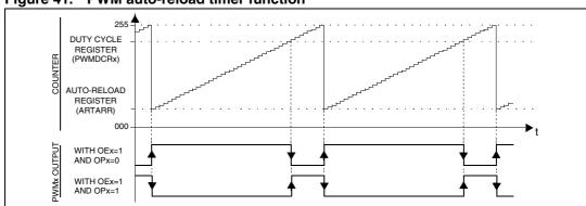
Figure 41. PWM auto-reload timer function
