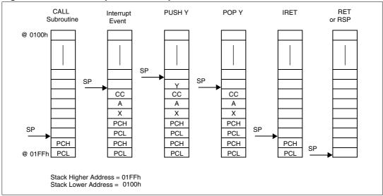
Figure 9. Stack manipulation example
