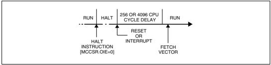
Figure 26. HALT mode flow-chart
