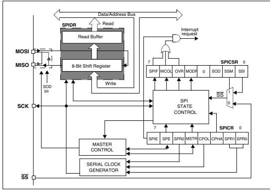
Figure 70. Serial peripheral interface block diagram
