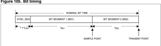
Figure 105. Bit timing
