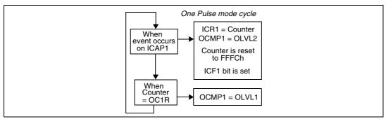
Then, on a valid event on the ICAP1 pin, the counter is initialized to FFFCh and OLVL2 bit is loaded on the OCMP1 pin, the ICF1 bit is set and the value FFFDh is loaded in the IC1R register.
