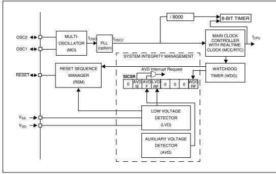
Figure 11. Clock, reset and supply block diagram
