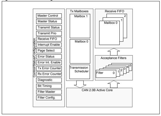
Figure 95. CAN block diagram
