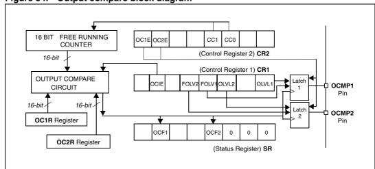
Figure 54. Output compare block diagram
