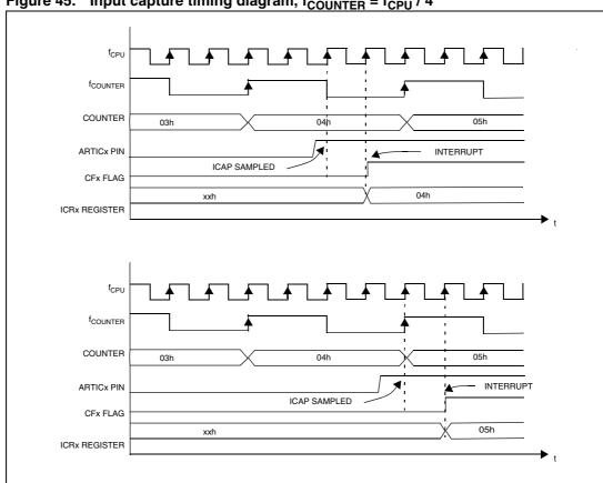
Figure 45. Input capture timing diagram, f<sub>COUNTER</sub> = f<sub>CPU</sub> / 4
