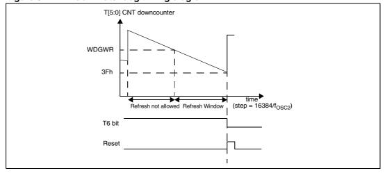
Figure 37. Window watchdog timing diagram
