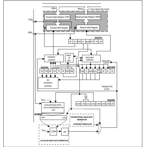
Figure 81. SCI block diagram in LIN slave mode
