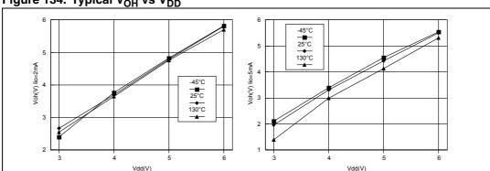
Figure 134. Typical  $V_{OH}$  vs  $V_{DD}$
