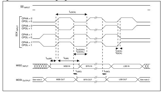
Figure 141. SPI master timing diagram
