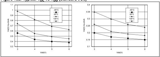
Figure 133. Typical  $V_{OL}$  vs  $V_{DD}$  (high-sink I/Os)
