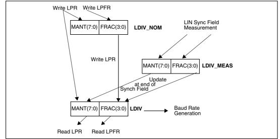
Figure 84. LDIV read / write operations when LDUM = 0
