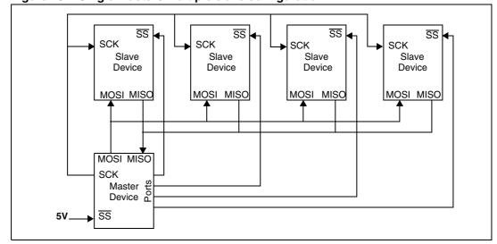
Figure 76. Single master / multiple slave configuration
