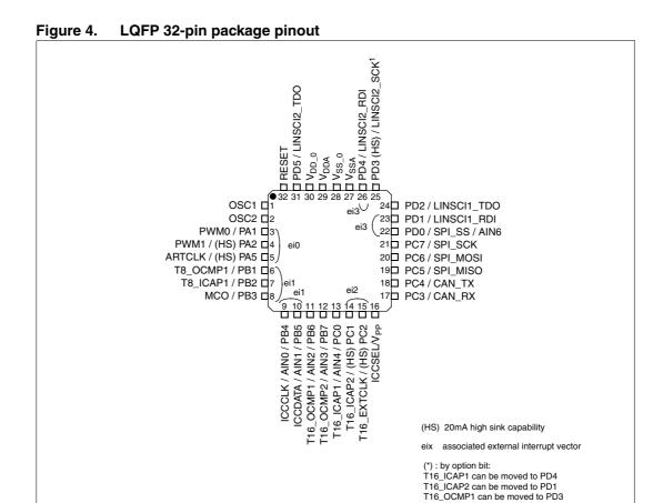
For external pin connection guidelines, refer to Chapter 20: Electrical characteristics.
