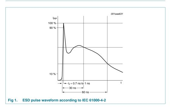
Ultra low capacitance double rail-to-rail ESD protection
