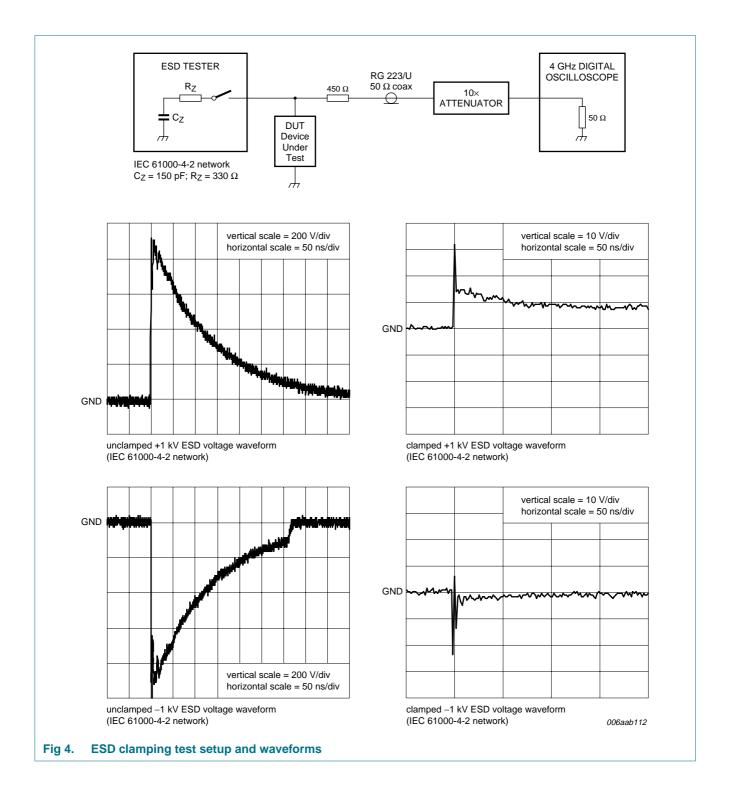
Ultra low capacitance double rail-to-rail ESD protection
