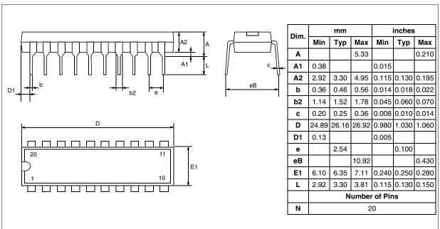
Figure 75. 20-Pin Ceramic Side-Brazed Dual In-Line Package
