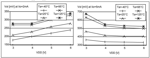
Figure 67. Typical V<sub>OL</sub> vs V<sub>DD</sub> (high-sink I/Os)
