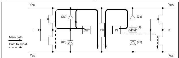
Figure 60. Negative Stress on a Standard Pad vs. V<sub>DD</sub>
