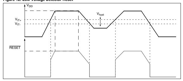
Figure 12. Low Voltage Detector Reset
