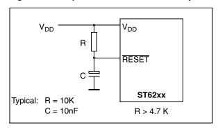
Figure 16. Reset Processing
