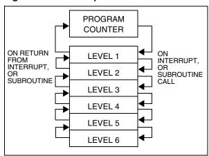
Since the accumulator, in common with all other data space registers, is not stored in this stack, management of these registers should be performed within the subroutine.
