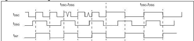
Figure 11. LFAO Oscillator Function
