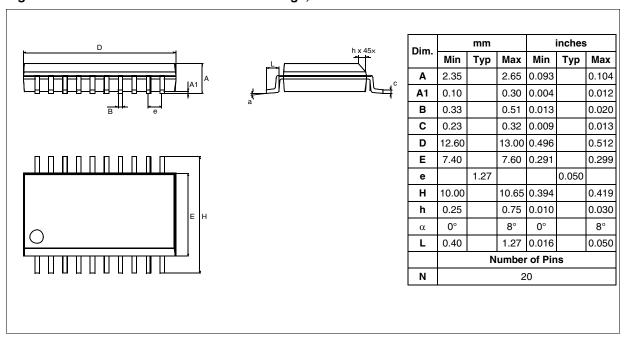
Figure 77. 20-Pin Plastic Shrink Small Outline Package
