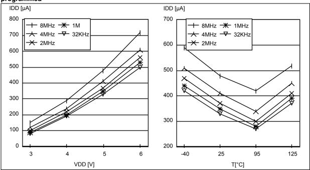
Figure 45. Typical  $I_{\text{DD}}$  in WAIT vs  $f_{\text{CPU}}$  and Temperature for OTP devices with option bytes programmed to 00H
