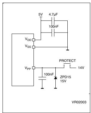
Note: ZPD15 is used for overvoltage protection
