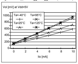
Figure 64. Typical  $V_{OL}$  at  $V_{DD} = 5V$  (high-sink)
