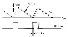
Figure 5—Jitter in PWM Mode
