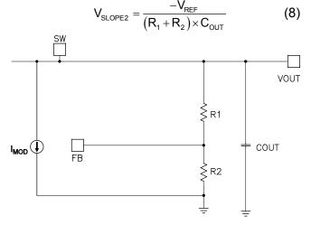
Figure 9—Simplified Circuit in Skip Mode
