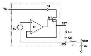
Figure 3: Internal Bootstrap Charging Circuit
