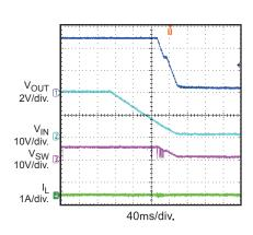
**Enable Startup**  $V_{IN} = 19V, V_{OLIT} = 5V, I_{O} = 2A$
