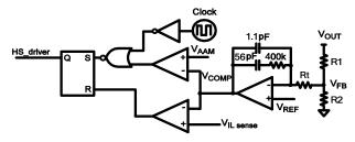
Figure 2: Simplified AAM Control Logic
