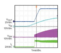
Power up  $V_{IN} = 19V, V_{OUT} = 5V, I_O = 0A$
