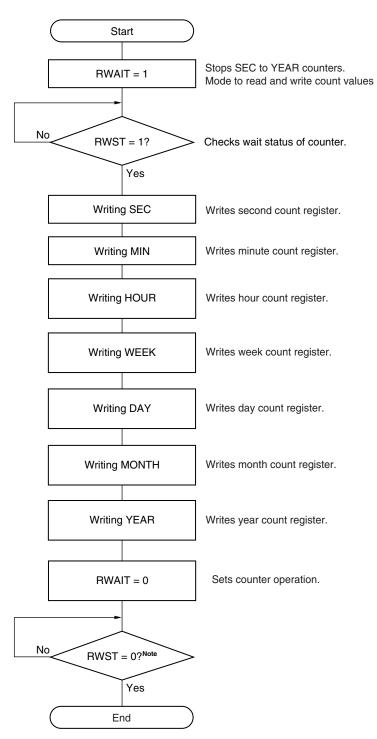
Figure 9-20. Procedure for Writing Real-Time Counter
