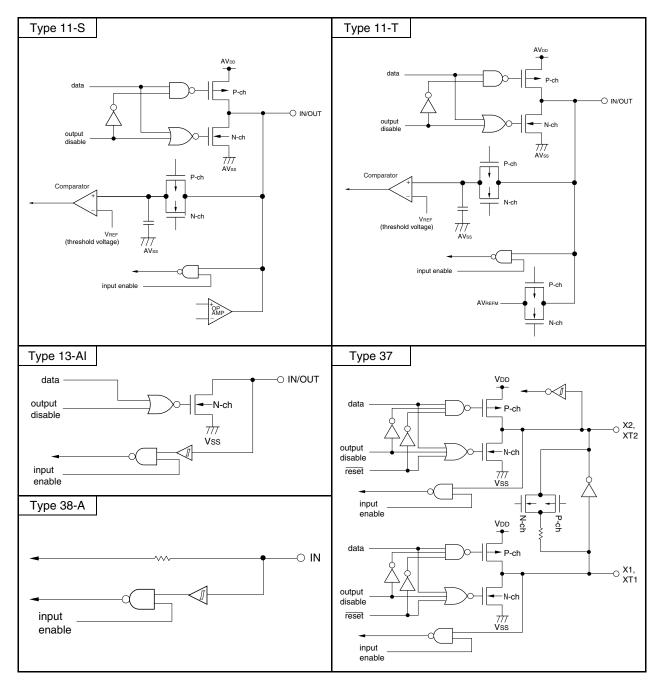
Figure 2-1. Pin I/O Circuit List (2/2)
