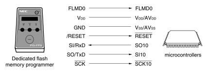
Caution: Only the P60/SCLA0/SCK10 and P61/SDAA0/SI10 pins (when used as the CSI10 pins SCK10 and SI10) can be used for communicating with the dedicated flash memory programmer. The P31/INTP5/OCD1A(/SCK10) and P32/INTP4/OCD1B(/SI10) pins cannot be used for communicating with the dedicated flash memory programmer.
