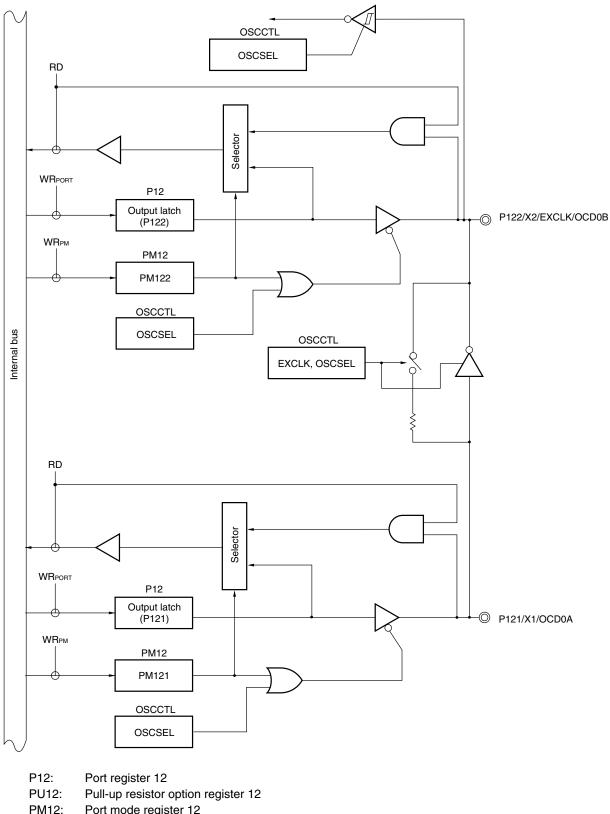
Figure 4-23. Block Diagram of P121 and P122
