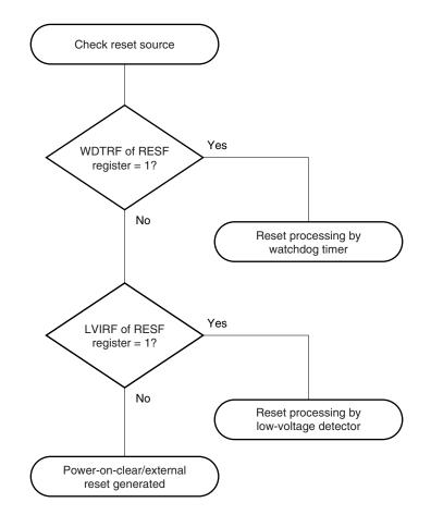
Figure 22-3. Example of Software Processing After Reset Release (2/2)
