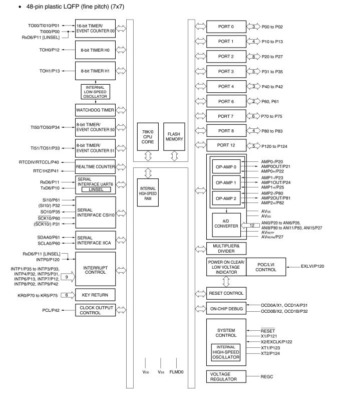
**Remark** The functions of pins whose names are in parentheses can be used by setting bit 2 (ISC2) of the input switch control register (ISC) to 1. If ISC2 is 0, serial interface CSI10 can only be used to send and received data as a slave.
