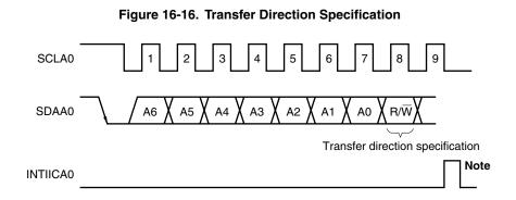
Note INTIICA0 is not issued if data other than a local address or extension code is received during slave device operation.
