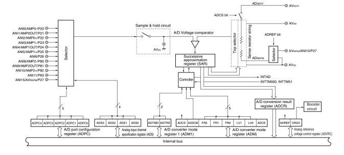
Figure 12-1. Block Diagram of A/D Converter
