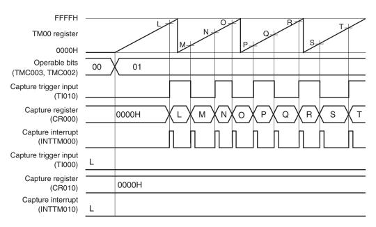
Figure 6-38. Timing Example of Free-Running Timer Mode (CR000: Capture Register, CR010: Capture Register) (2/2)
