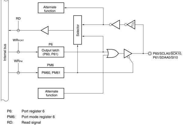
Figure 4-16. Block Diagram of P60 and P61
