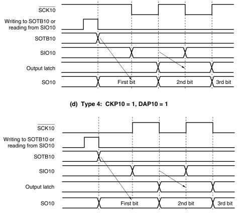
Figure 15-10. Output Operation of First Bit (2/2)
