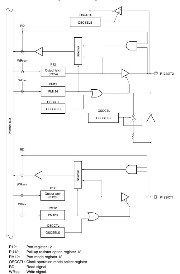
Figure 4-24. Block Diagram of P123 and P124
