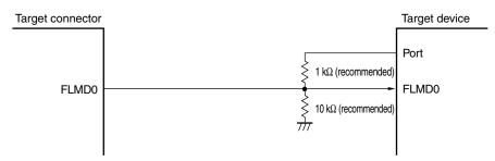
Caution When using the port that controls the FLMD0 pin, make sure that it satisfies the values of the highlevel output current and FLMD0 supply voltage (minimum value: 0.8VDD) stated in CHAPTER 28 ELECTRICAL SPECIFICATIONS.
