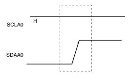
A stop condition is generated when bit 0 (SPT0) of IICA control register 0 (IICACTL0) is set to 1. When the stop condition is detected, bit 0 (SPD0) of the IICA status register 0 (IICAS0) is set to 1 and INTIICA0 is generated when bit 4 (SPIE0) of IICACTL0 is set to 1.
