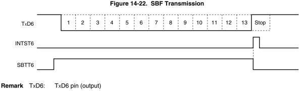
INTST6: Transmission completion interrupt request
