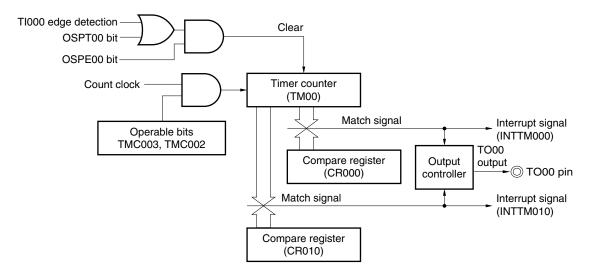
Figure 6-44. Block Diagram of One-Shot Pulse Output Operation
