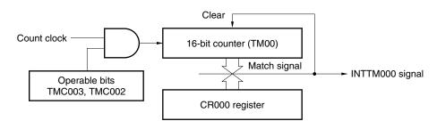
Figure 6-12. Block Diagram of Interval Timer Operation
