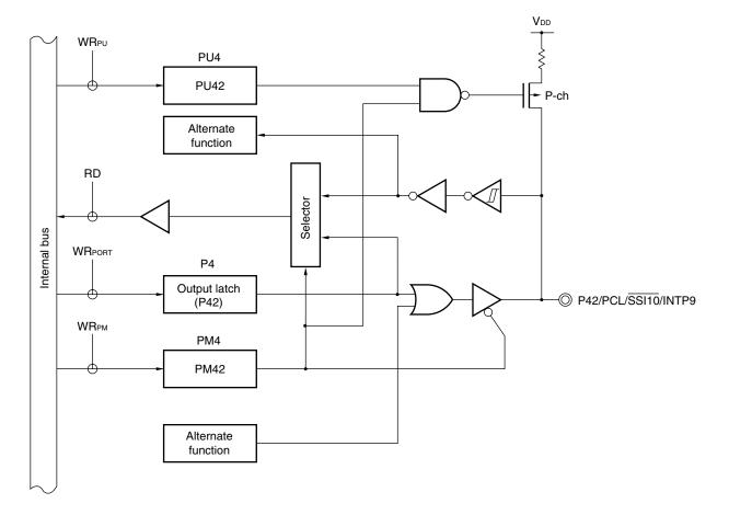
Figure 4-15. Block Diagram of P42
