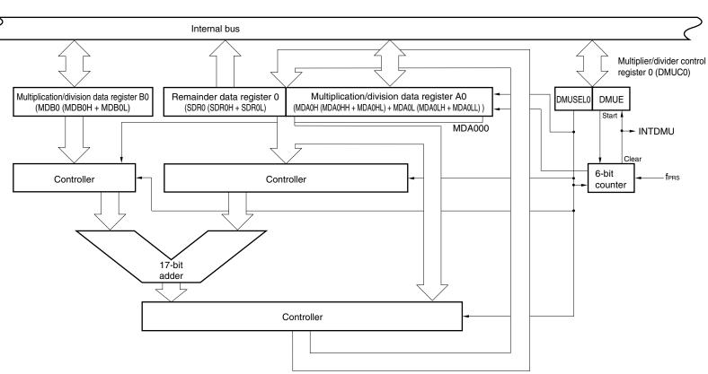
Figure 17-1. Block Diagram of Multiplier/Divider
