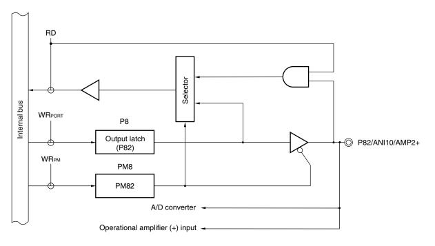
Figure 4-20. Block Diagram of P82
