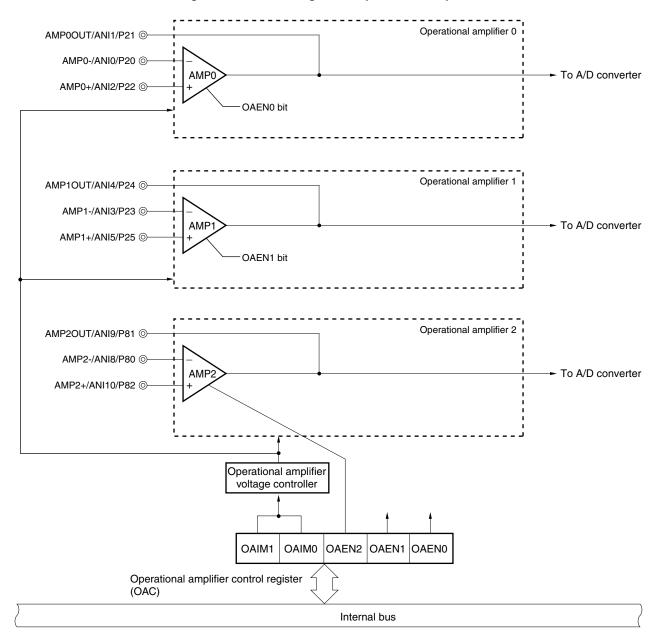
Figure 13-1. Block Diagram of Operational Amplifier
