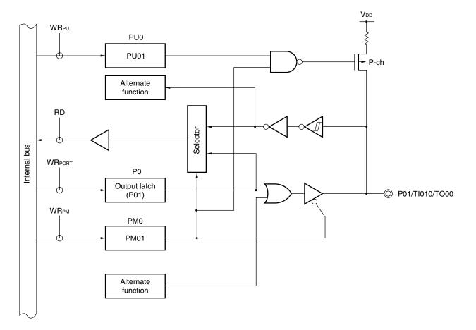
Figure 4-2. Block Diagram of P01
