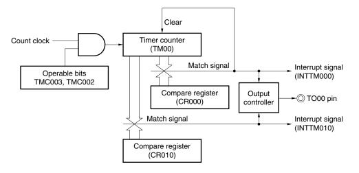
Figure 6-41. Block Diagram of PPG Output Operation
