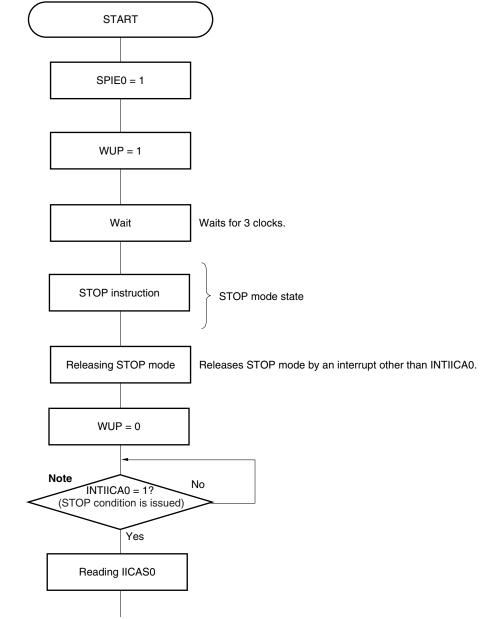
Executes processing corresponding to the operation to be executed after checking the operation state of serial interface IICA.
