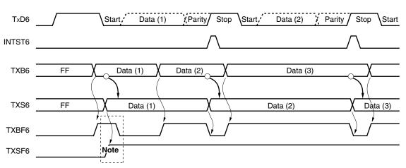
Figure 14-17. Timing of Starting Continuous Transmission
