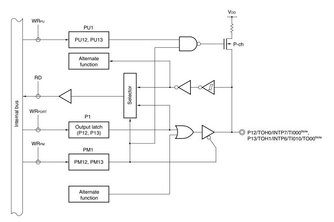
Figure 4-5. Block Diagram of P12 and P13
