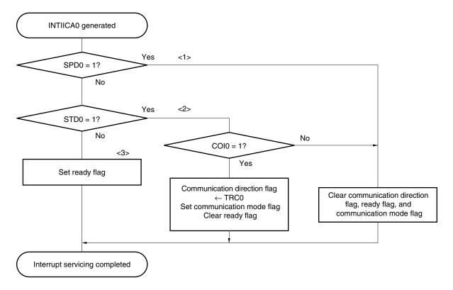
Figure 16-31. Slave Operation Flowchart (2)
