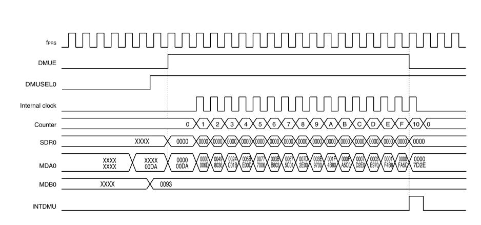
Figure 17-6. Timing Chart of Multiplication Operation (00DAH × 0093H)
