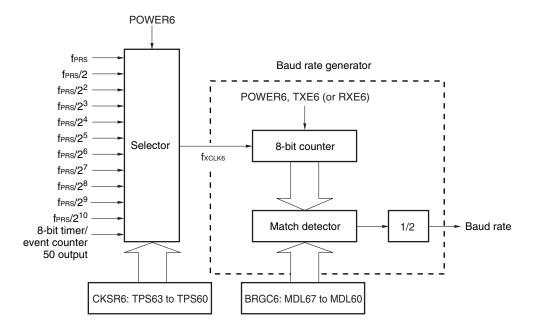
Figure 14-24. Configuration of Baud Rate Generator
