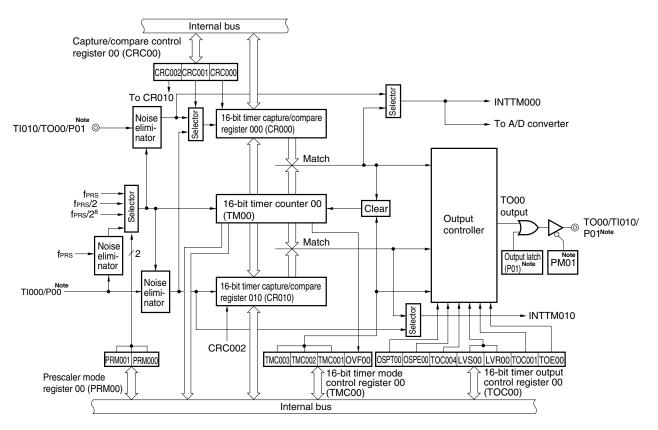
Figure 6-1. Block Diagram of 16-Bit Timer/Event Counter 00
