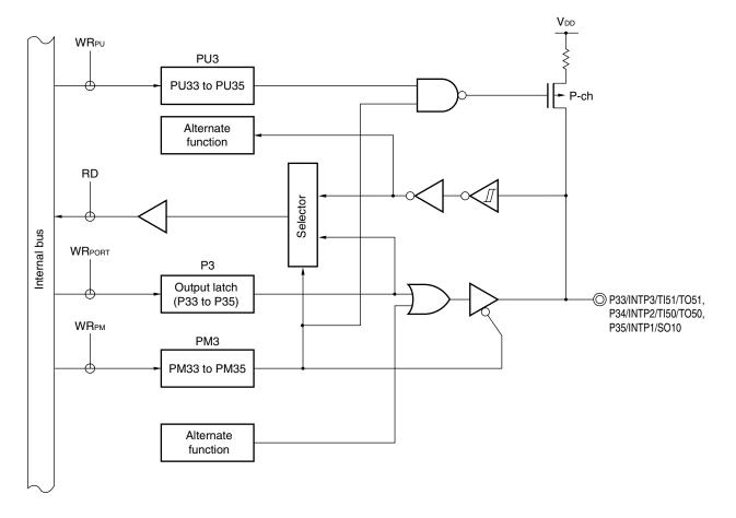
Figure 4-13. Block Diagram of P33 to P35
