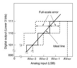
Figure 12-24. Differential Linearity Error
