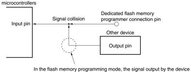
In the flash memory programming mode, the signal output by the device collides with the signal sent from the dedicated flash programmer. Therefore, isolate the signal of the other device.
