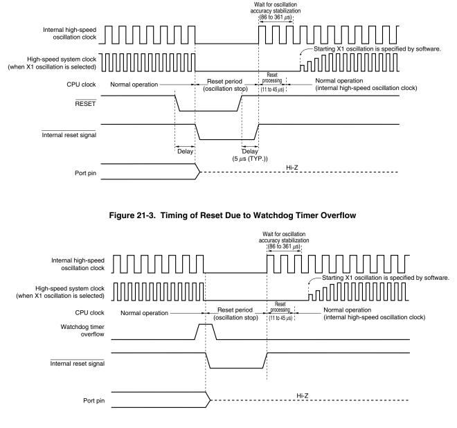
Figure 21-2. Timing of Reset by RESET Input
