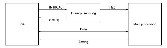
Therefore, data communication processing is performed by preparing the following three flags and passing them to the main processing instead of INTIICA0.
