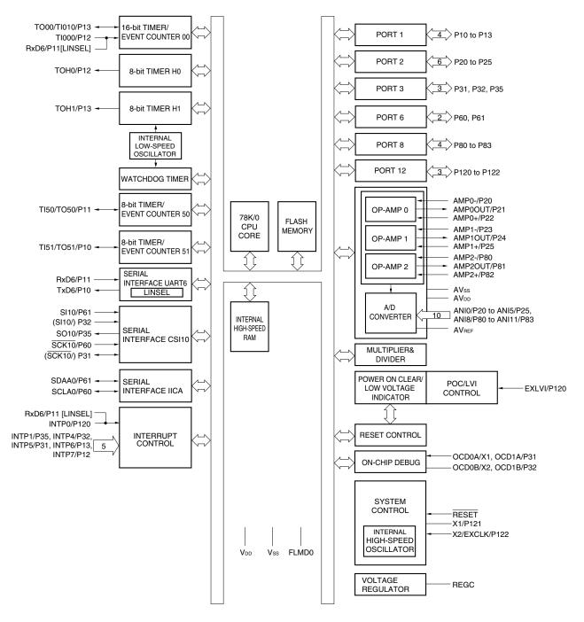
**Remark** The functions of pins whose names are in parentheses can be used by setting bit 2 (ISC2) of the input switch control register (ISC) to 1. If ISC2 is 0, serial interface CSI10 can only be used to send and received data as a slave.
