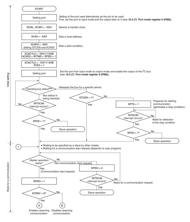
**Note** Confirm that the bus is released (CLD0 bit = 1, DAD0 bit = 1) for a specific period (for example, for a period of one frame). If the SDAA0 pin is constantly at low level, decide whether to release the l<sup>2</sup>C bus (SCLA0 and SDAA0 pins = high level) in conformance with the specifications of the product that is communicating.
