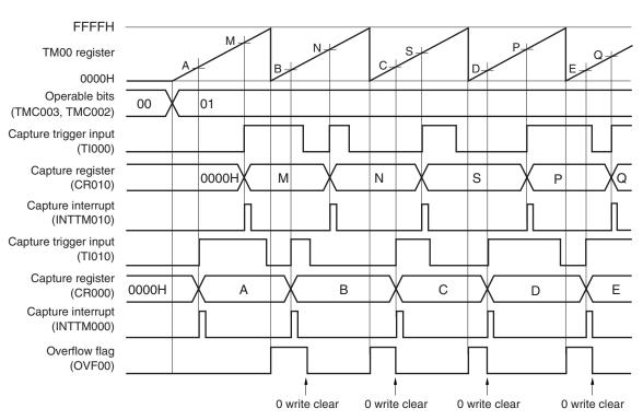
Figure 6-38. Timing Example of Free-Running Timer Mode (CR000: Capture Register, CR010: Capture Register) (1/2)
