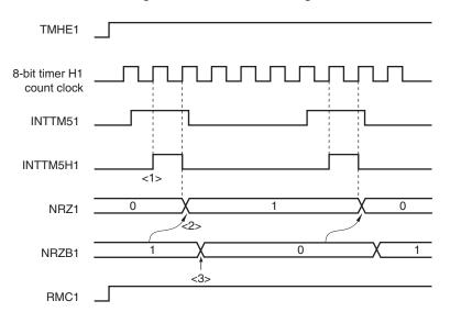
Figure 8-13. Transfer Timing
