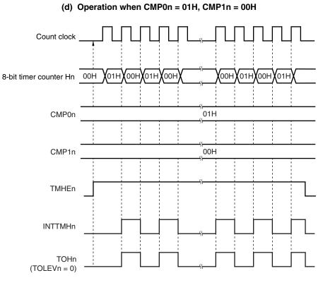
Figure 8-12. Operation Timing in PWM Output Mode (3/4)
