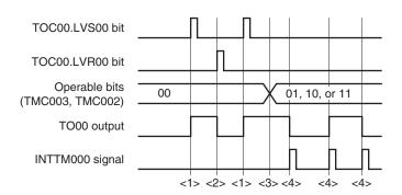
Figure 6-55. Timing Example of LVR00 and LVS00
