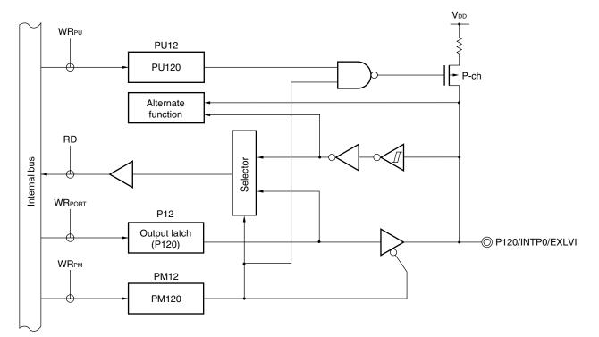
Figure 4-22. Block Diagram of P120
