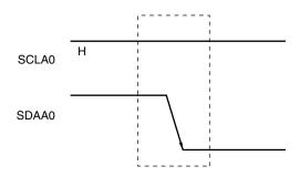
A start condition is output when bit 1 (STT0) of IICA control register 0 (IICACTL0) is set (1) after a stop condition has been detected (SPD0: Bit 0 of the IICA status register 0 (IICAS0) = 1). When a start condition is detected, bit 1 (STD0) of IICAS0 is set (1).
