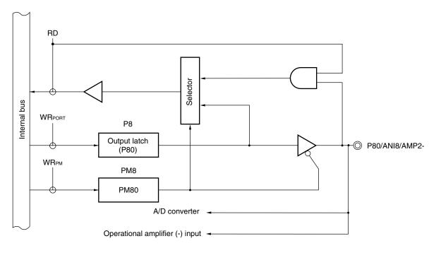
Figure 4-18. Block Diagram of P80
