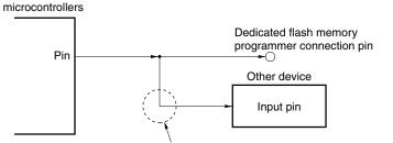
If the signal output by microcontrollers in the flash memory programming mode affects the other device, isolate the signal of the other device.
