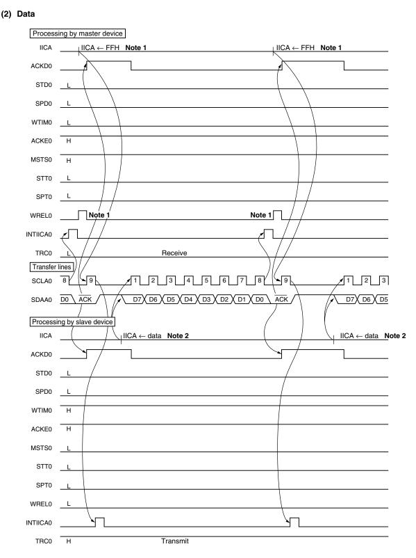
Figure 16-33. Example of Slave to Master Communication (When 8-Clock Wait Is Selected for Master, 9-Clock Wait Is Selected for Slave) (2/3)
