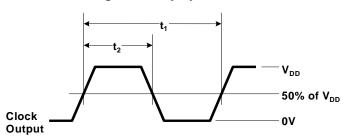
Figure 6. Rise Time =  $T_{RF}$ , Fall Time =  $T_{RF}$
