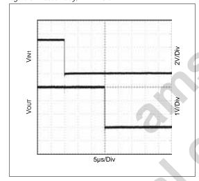
Figure 9. Reset Active Timeout Periode; VIN2 = 3.0V
