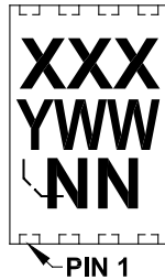
8-Lead DFN (3x3x0.9 mm) (MCP662)
