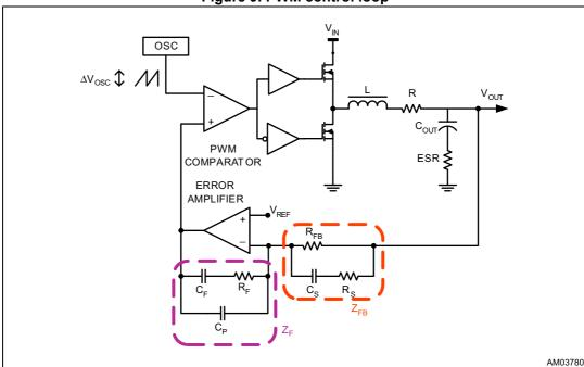
Figure 9. PWM control loop
