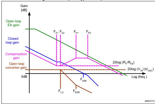
Figure 10. Example of type III compensation
