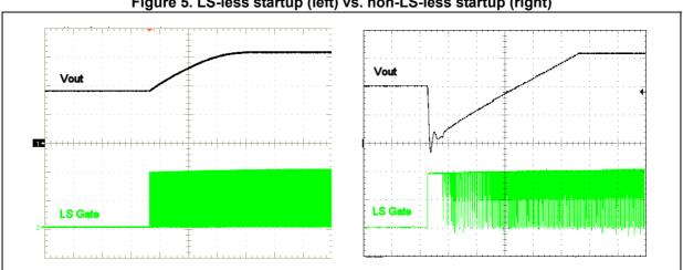
Figure 5. LS-less startup (left) vs. non-LS-less startup (right)
