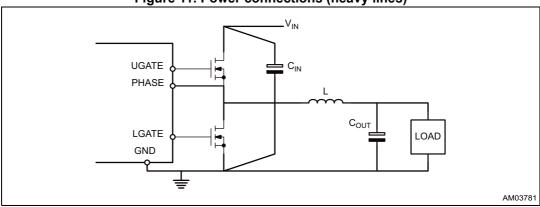
Figure 11. Power connections (heavy lines)
