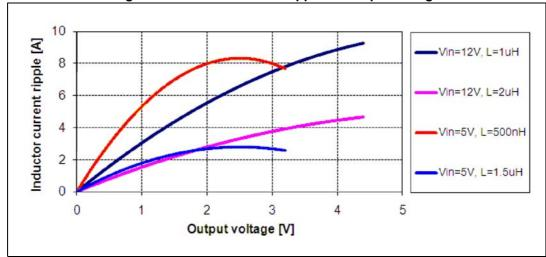
Figure 13. Inductor current ripple vs. output voltage
