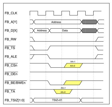
Figure 30-30. Single Byte-Write Transfer
