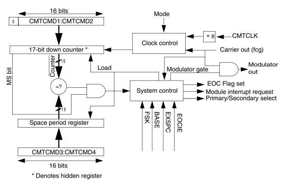
Figure 41-16. Modulator block diagram
