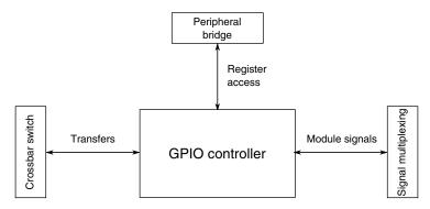
Figure 3-55. GPIO configuration
