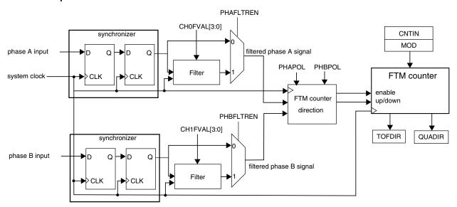
Figure 38-250. Quadrature Decoder block diagram
