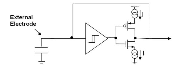
Figure 50-33. TSI electrode oscillator circuit
