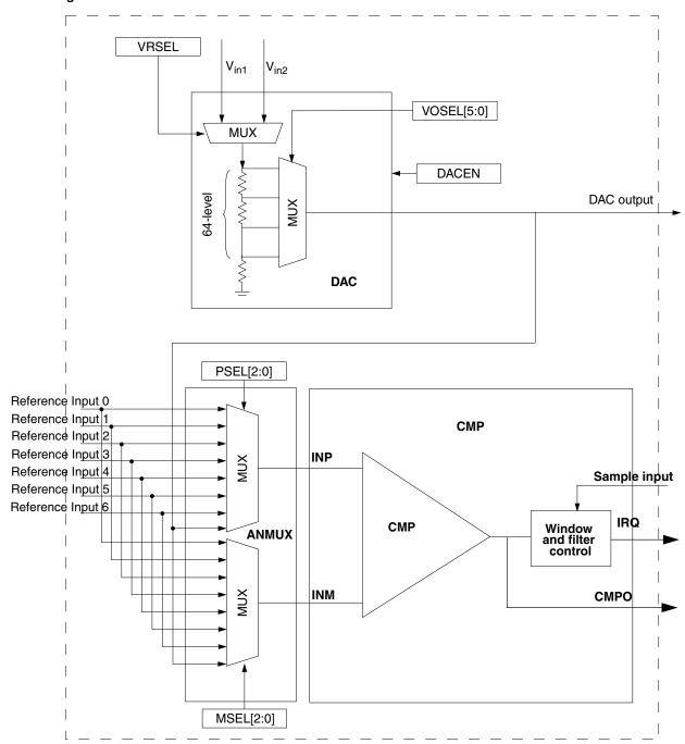
Figure 34-1. CMP, DAC and ANMUX block diagram
