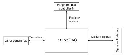
Figure 3-38. 12-bit DAC configuration
