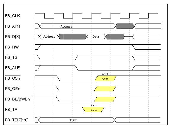
Figure 30-44. Read-Bus Cycle with CSCRn[EXTS] = 1 (One Wait State)
