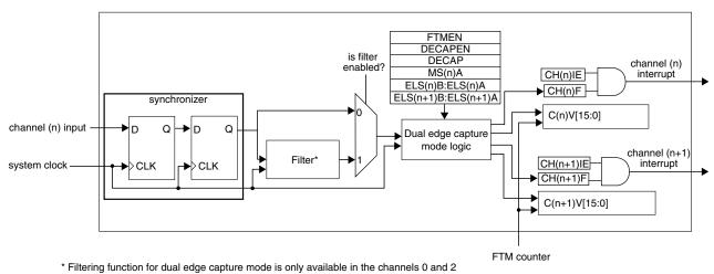
Figure 38-244. Dual Edge Capture mode block diagram
