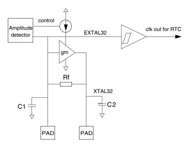
Figure 27-1. RTC Oscillator Block Diagram
