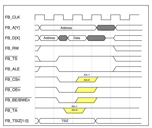
Figure 30-26. Basic Read-Bus Cycle
