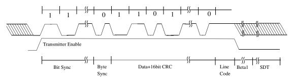
Figure 46-337. Frame format with differential manchester encoding
