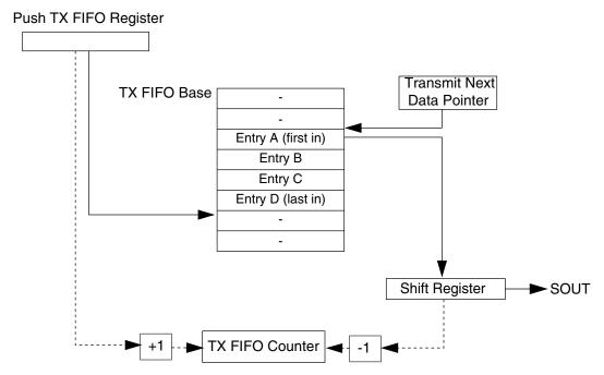
Figure 44-99. TX FIFO pointers and counter
