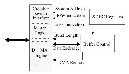
Figure 47-31. DMA crossbar switch interface block
