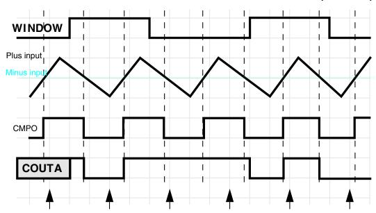
Figure 34-32. Windowed mode operation
