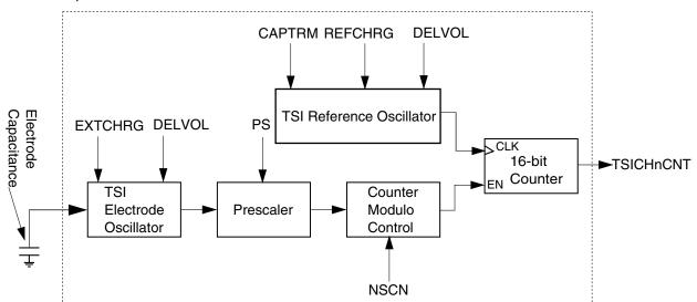
Figure 50-2. TSI capacitance measurement unit block diagram
