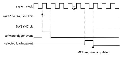
Figure 38-213. MOD synchronization with (SYNCMODE = 0) and (PWMSYNC = 1)
