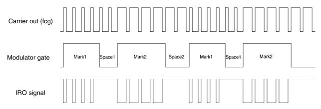
Figure 41-18. Example: CMT output in FSK mode
