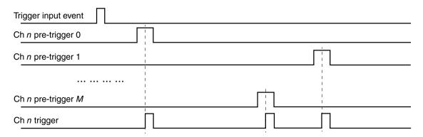
Figure 37-56. Pre-trigger and trigger outputs
