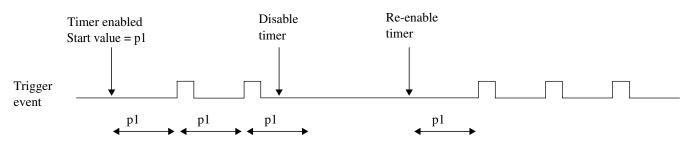
Figure 39-23. Stopping and starting a timer
