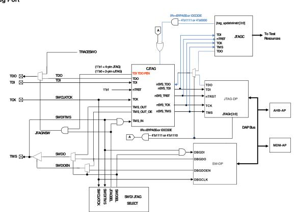
Figure 9-2. Modified Debug Port
