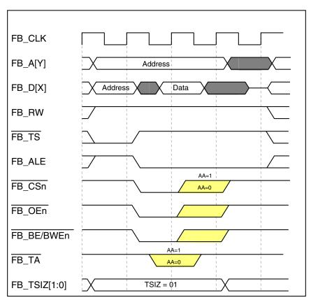
Figure 30-29. Single Byte-Read Transfer
