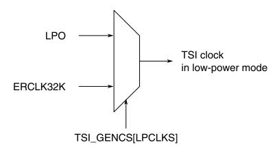
Figure 5-10. TSI low-power clock generation
