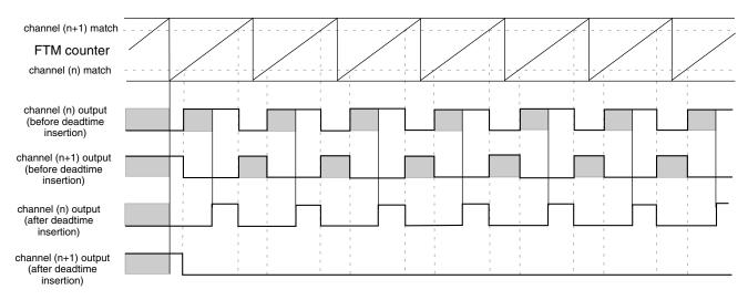
Figure 38-230. Example of the deadtime insertion (ELSnB:ELSnA = 1:0, POL(n) = 0, and POL(n+1) = 0) when the deadtime delay is comparable to channel (n+1) duty cycle
