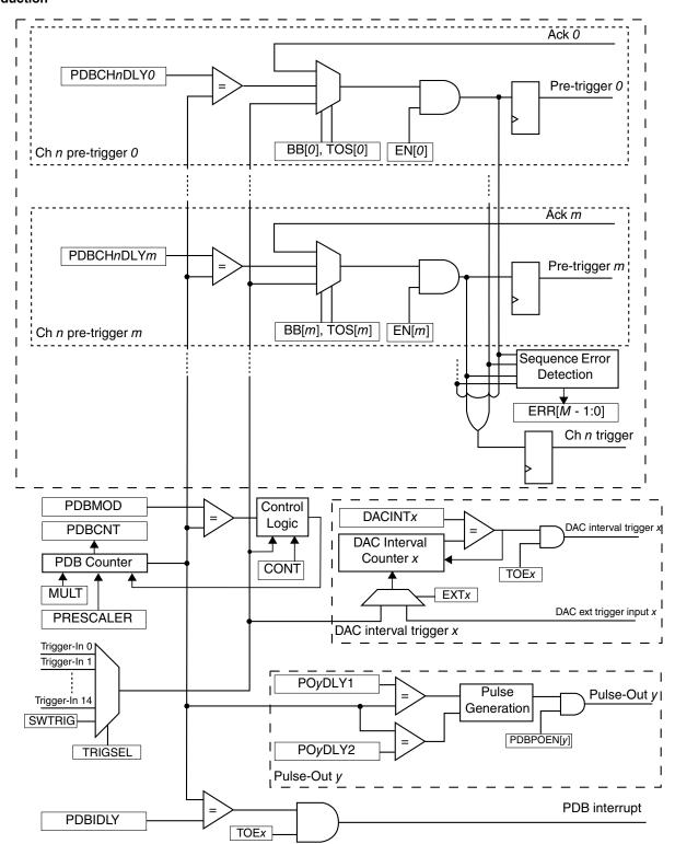
Figure 37-1. PDB block diagram
