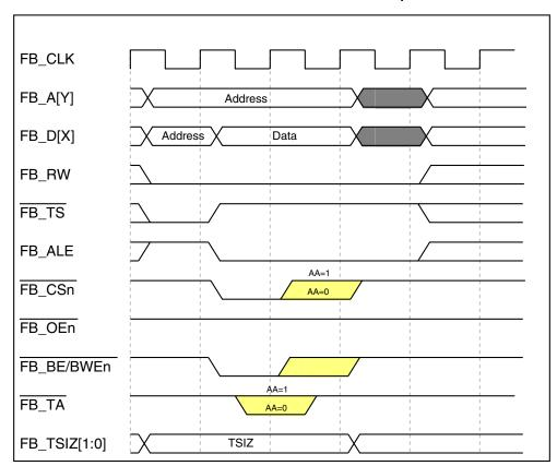
Figure 30-36. Basic Write-Bus Cycle (No Wait States)
