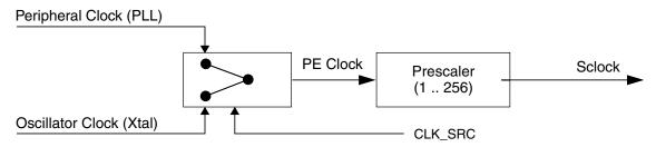
Figure 43-98. CAN engine clocking scheme
