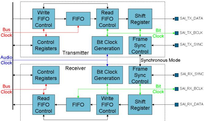
Figure 48-1. I<sup>2</sup>S/SAI block diagram
