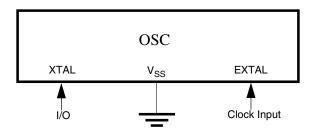
Figure 26-5. External Clock Connections
