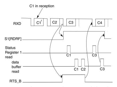
Figure 46-345. Receiver hardware flow control timing diagram
