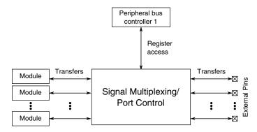
Figure 10-1. Signal multiplexing integration
