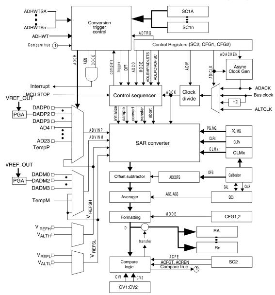
Figure 33-1. ADC block diagram
