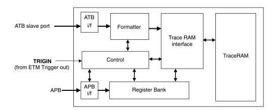
Figure 9-5. ETB Block Diagram
