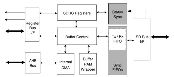
Figure 47-27. SDHC buffer scheme
