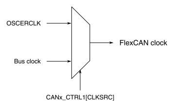
Figure 5-6. FlexCAN clock generation
