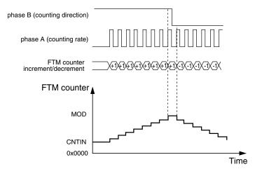
Figure 38-251. Quadrature Decoder – Count and Direction Encoding mode
