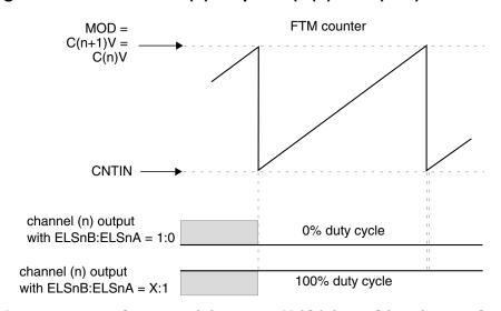
Figure 38-196. Channel (n) output if (C(n)V = C(n+1)V = MOD)
