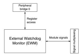
Figure 3-15. External Watchdog Monitor configuration
