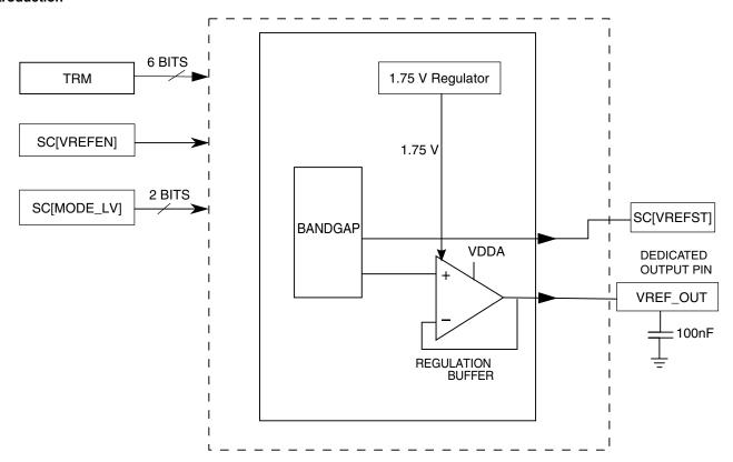
Figure 36-1. Voltage reference block diagram
