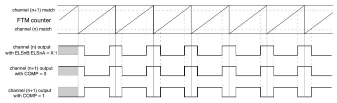
Figure 38-204. Channel (n+1) output in Complementary mode with (ELSnB:ELSnA = X:1)
