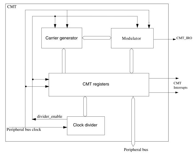
Figure 41-1. CMT module block diagram
