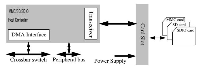
Figure 47-1. System connection of the SDHC
