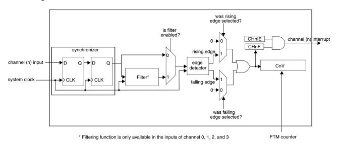
Figure 38-175. Input Capture mode
