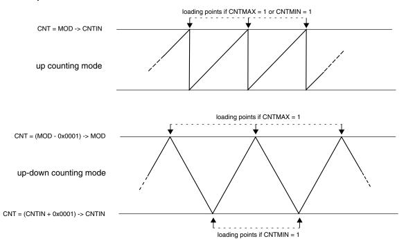
Figure 38-207. Boundary cycles and loading points
