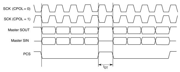
Figure 44-97. Continuous SCK Timing Diagram (CONT=0)
