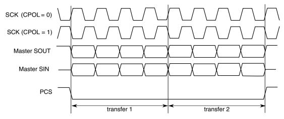
Figure 44-98. Continuous SCK timing diagram (CONT=1)
