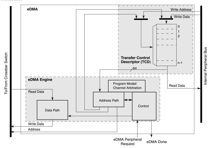
Figure 22-1. eDMA block diagram
