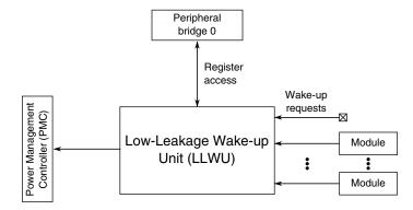
Figure 3-8. Low-Leakage Wake-up Unit configuration
