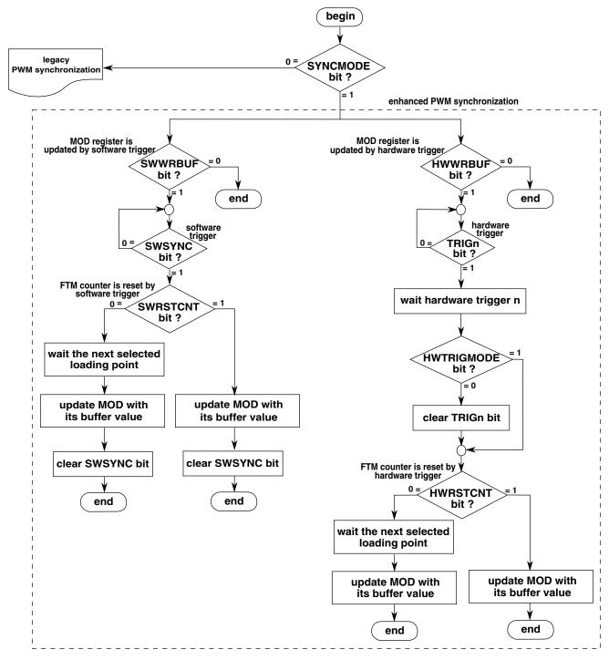
Figure 38-208. MOD register synchronization flowchart
