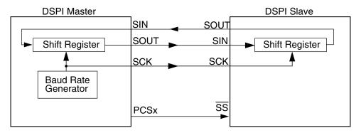
Figure 44-91. SPI serial protocol overview
