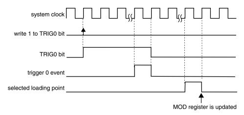
Figure 38-210. MOD synchronization with (SYNCMODE = 0), (HWTRIGMODE = 0), (PWMSYNC = 0), (REINIT = 0), and a hardware trigger was used
