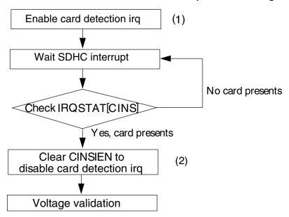
Figure 47-39. Flow diagram for card detection
