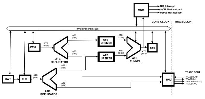
Figure 9-4. Core Trace Connectivity
