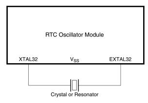
Figure 27-2. Crystal Connections
