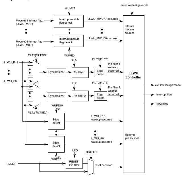
Figure 16-1. LLWU block diagram
