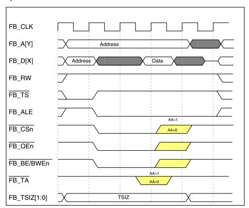
Figure 30-37. Read-Bus Cycle (One Wait State)
