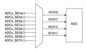
Figure 3-34. ADCx\_SEn channels a and b selection
