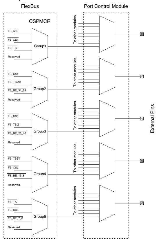
Figure 3-31. FlexBus control signal multiplexing
