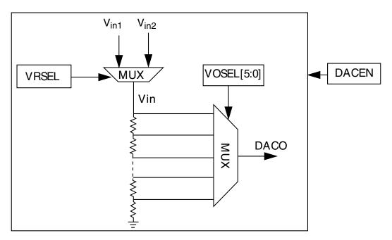
Figure 34-36. 6-bit DAC block diagram
