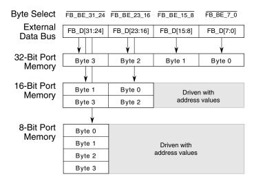
Figure 30-23. Connections for external memory port sizes (CSCRn[BLS] = 0)
