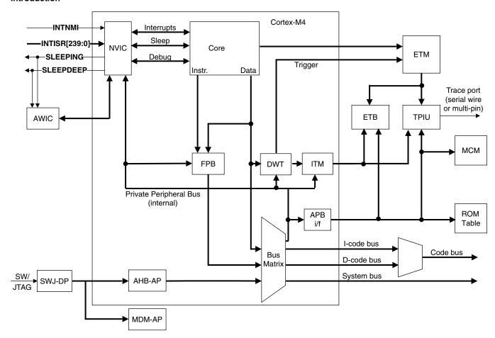
Figure 9-1. Cortex-M4 Debug Topology
