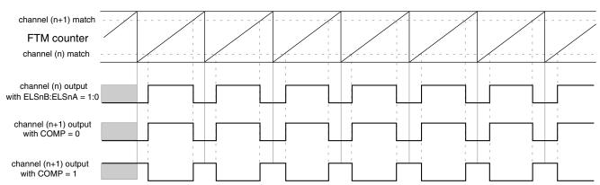
Figure 38-203. Channel (n+1) output in Complementary mode with (ELSnB:ELSnA = 1:0)
