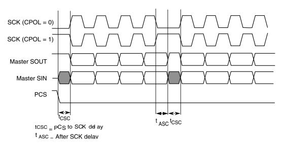
Figure 44-96. Example of continuous transfer (CPHA=1, CONT=1)
