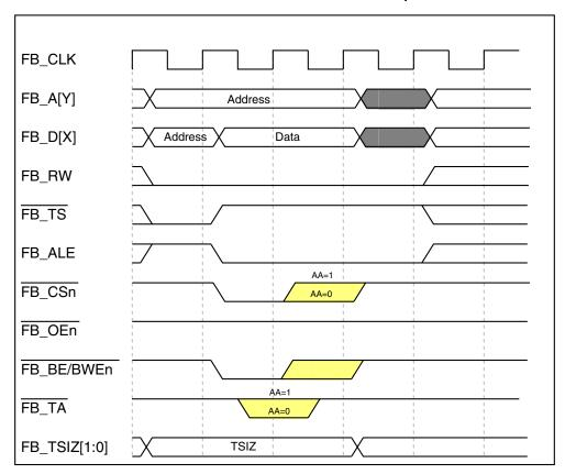
Figure 30-28. Basic Write-Bus Cycle
