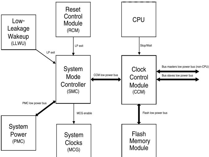
Figure 14-6. Low-power system components and connections
