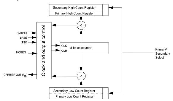
Figure 41-15. Carrier generator block diagram
