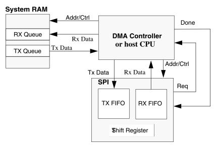
Figure 44-2. SPI with queues and DMA
