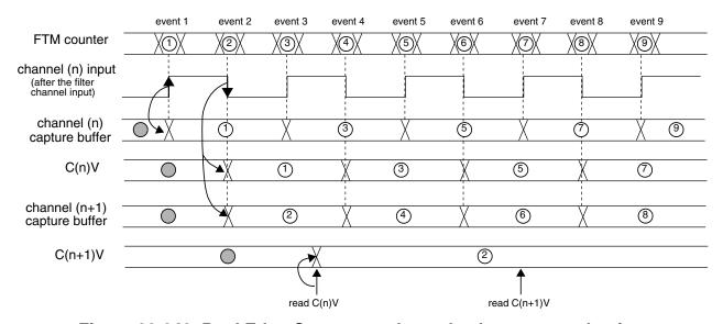
Figure 38-249. Dual Edge Capture mode read coherency mechanism
