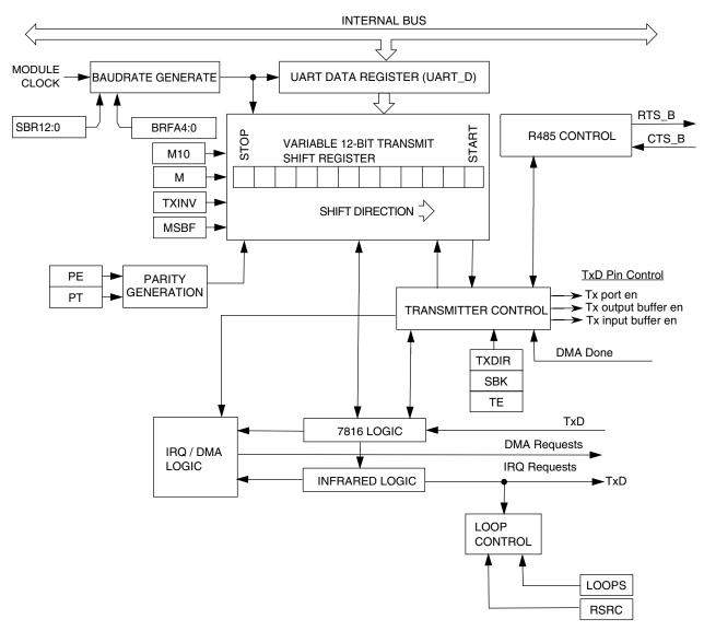
Figure 46-342. Transmitter Block Diagram
