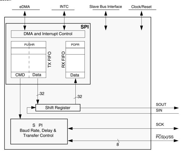
Figure 44-1. SPI Block Diagram
