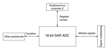
Figure 3-33. 16-bit SAR ADC with PGA configuration
