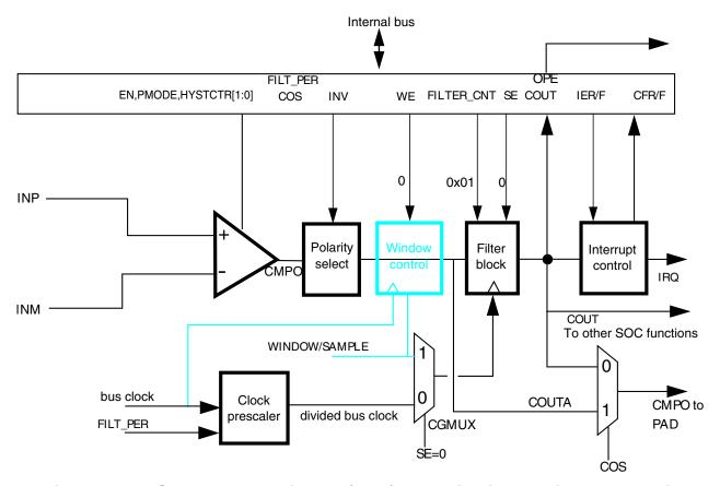
Figure 34-29. Sampled, Non-Filtered (# 3B): sampling interval internally derived
