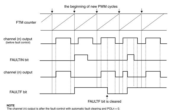
Figure 38-235. Fault control with automatic fault clearing
