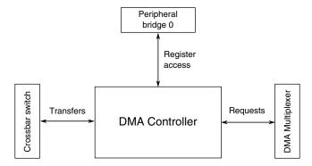
Figure 3-14. DMA Controller configuration
