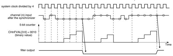
Figure 38-177. Channel input filter example
