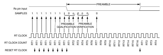
Figure 46-340. Receiver data sampling
