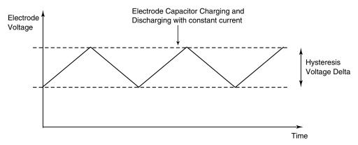
Figure 50-34. TSI electrode oscillator chart
