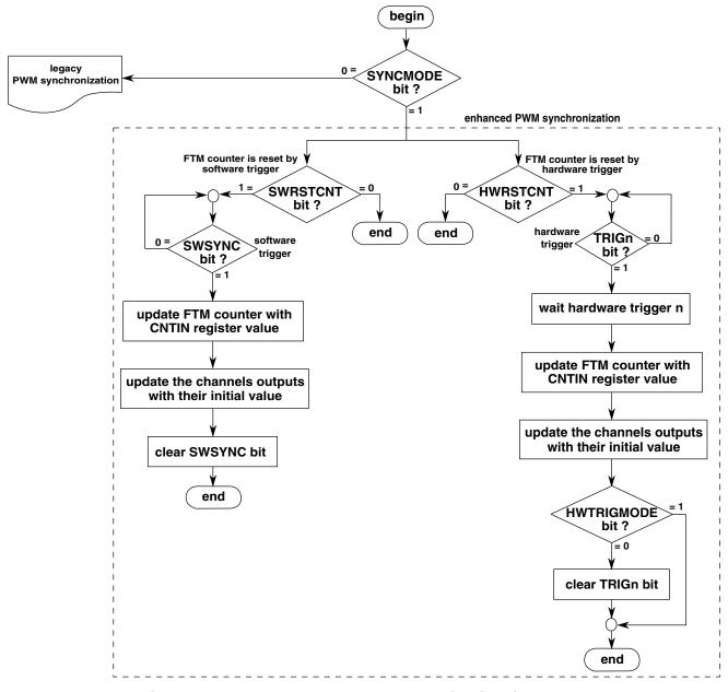
Figure 38-221. FTM counter synchronization flowchart
