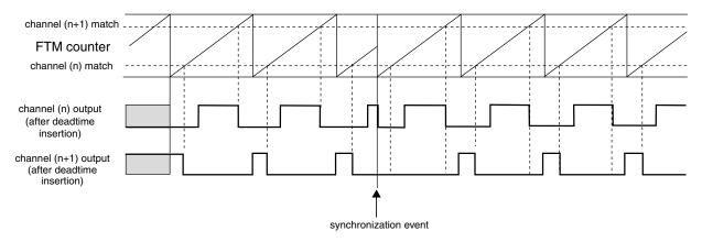
Figure 38-220. FTM counter synchronization
