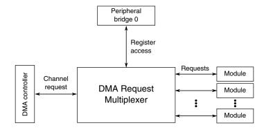
Figure 3-13. DMA request multiplexer configuration
