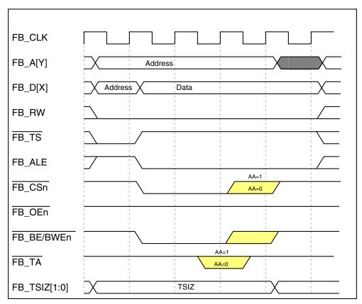
Figure 30-38. Write-Bus Cycle (One Wait State)
