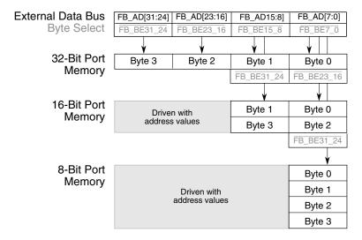
Figure 30-24. Connections for external memory port sizes (CSCRn[BLS] = 1)
