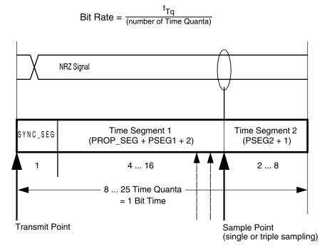
Figure 43-99. Segments within the bit time
