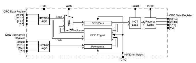
Figure 32-1. Programmable cyclic redundancy check (CRC) block diagram
