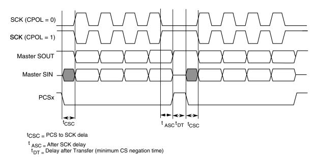
Figure 44-95. Example of non-continuous format (CPHA=1, CONT=0)
