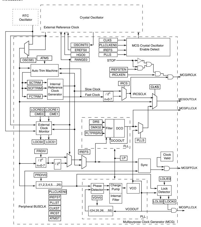
Figure 25-1. Multipurpose Clock Generator (MCG) block diagram
