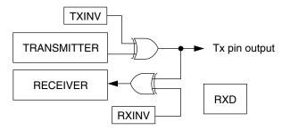
Figure 46-359. Loop operation (C1[LOOPS] = 1, C1[RSRC] = 0)
