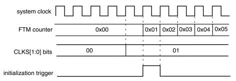
Figure 38-242. Initialization trigger is generated if (CNT = CNTIN), (CLKS[1:0] = 0:0), and a value different from zero is written to CLKS[1:0] bits
