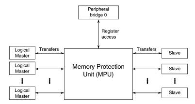
Figure 3-11. Memory Protection Unit configuration
