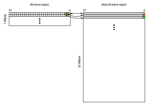
Figure 4-1. Alias bit-band mapping
