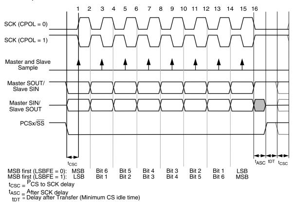
Figure 44-93. Module transfer timing diagram (MTFE=0, CPHA=0, FMSZ=8)
