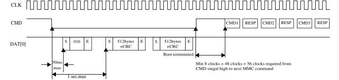
Figure 47-37. Multimediacard state diagram in Normal Boot mode
