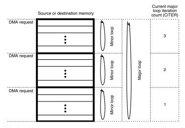
Figure 22-292. Example of multiple loop iterations
