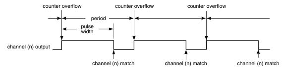
Figure 38-181. EPWM period and pulse width with ELSnB:ELSnA = 1:0
