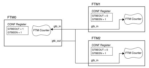
Figure 3-43. FTM Global Time Base Configuration
