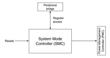
Figure 3-6. System Mode Controller configuration
