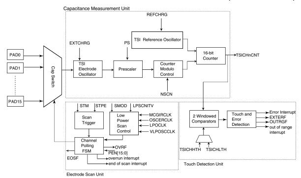
Figure 50-3. TSI block diagram
