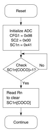
Figure 33-97. Initialization flowchart example
