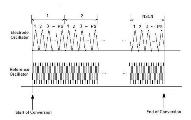
Figure 50-32. Dual electrode capacitance measurement
