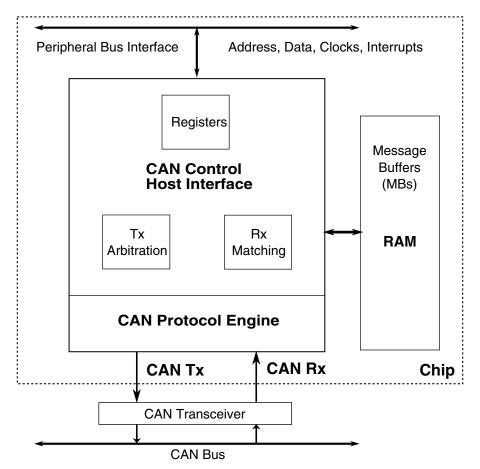
Figure 43-1. FlexCAN block diagram
