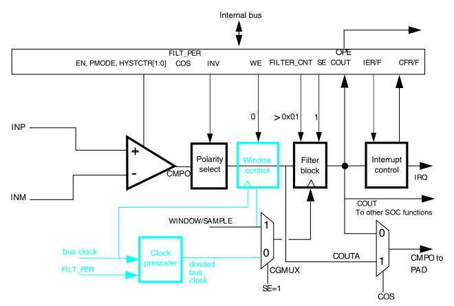
Figure 34-30. Sampled, Filtered (# 4A): sampling point externally driven
