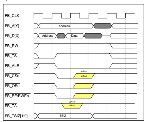
Figure 30-35. Basic Read-Bus Cycle (No Wait States)
