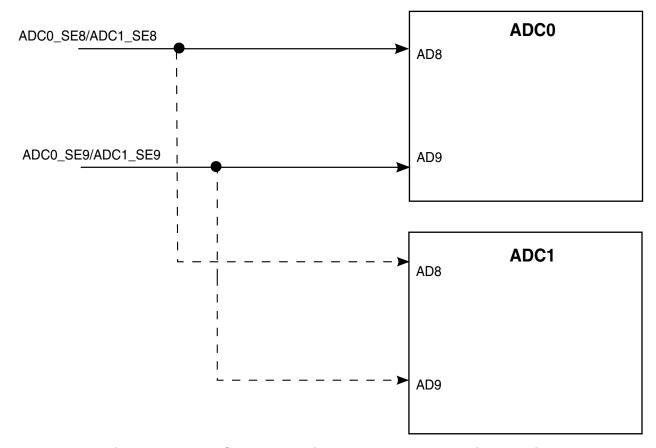
Figure 3-35. ADC hardware interleaved channels integration
