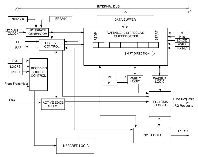
Figure 46-344. UART receiver block diagram
