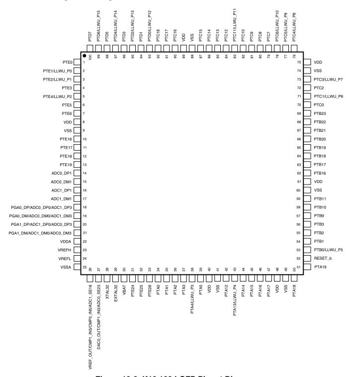
Figure 10-2. K10 100 LQFP Pinout Diagram
