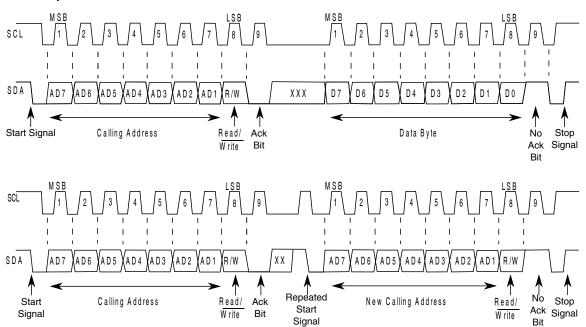
Figure 45-38. I2C bus transmission signals
