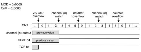
Figure 38-179. Example of the Output Compare mode when the match clears the channel output
