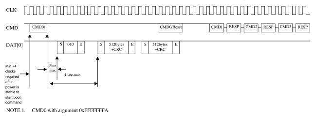
Figure 47-38. MultiMediaCard state diagram in Alternative Boot mode
