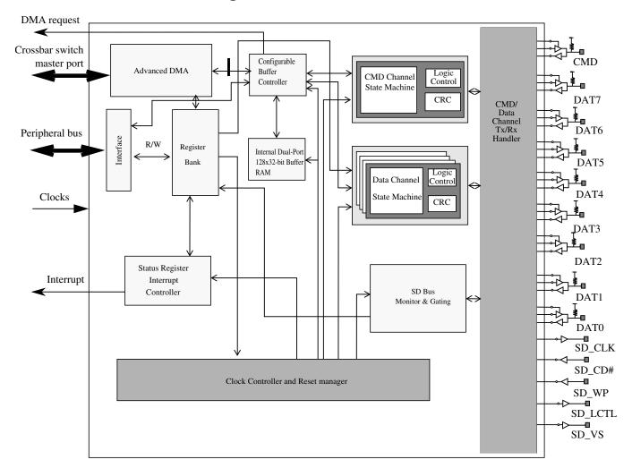
Figure 47-2. Enhanced secure digital host controller block diagram
