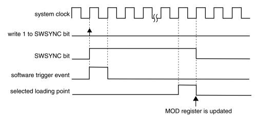
Figure 38-209. MOD synchronization with (SYNCMODE = 0), (PWMSYNC = 0), (REINIT = 0), and software trigger was used
