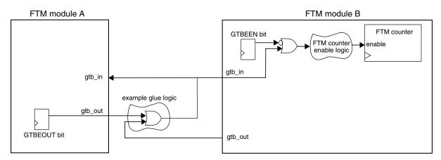
Figure 38-258. Global time base (GTB) block diagram
