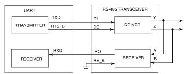
Figure 46-363. Transceiver driver enable using RTS
