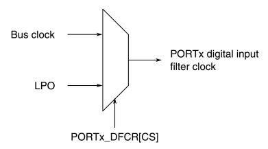
Figure 5-4. PORTx digital input filter clock generation
