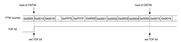
Figure 38-170. Example of up counting when the value of CNTIN is greater than the value of MOD
