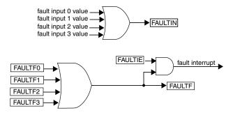
Figure 38-234. FAULTF and FAULTIN bits and fault interrupt
