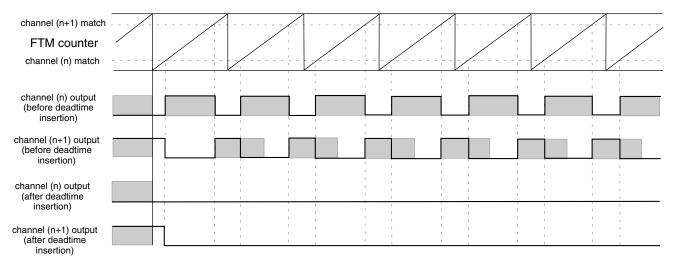
Figure 38-231. Example of the deadtime insertion (ELSnB:ELSnA = 1:0, POL(n) = 0, and POL(n+1) = 0) when the deadtime delay is comparable to channels (n) and (n+1) duty cycle
