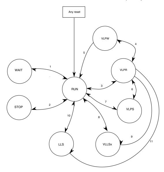
Figure 14-5. Power mode state diagram
