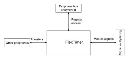
Figure 3-42. FlexTimer configuration
