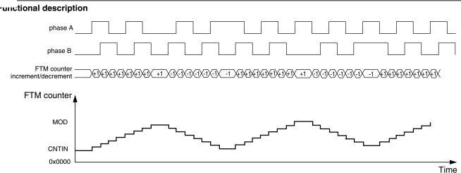
Figure 38-252. Quadrature Decoder – Phase A and Phase B Encoding mode
