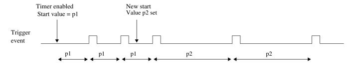
Figure 39-25. Dynamically setting a new load value
