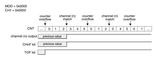
Figure 38-180. Example of the Output Compare mode when the match sets the channel output
