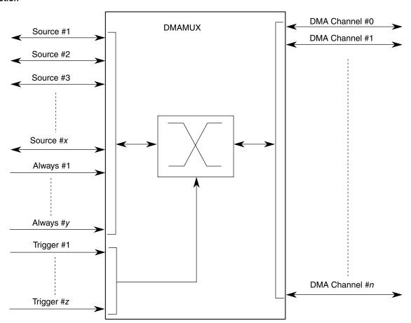
Figure 21-1. DMAMUX block diagram
