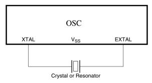
Figure 26-2. Crystal/Ceramic Resonator Connections - Connection 1
