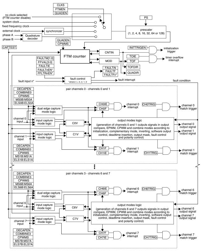
Figure 38-1. FTM block diagram
