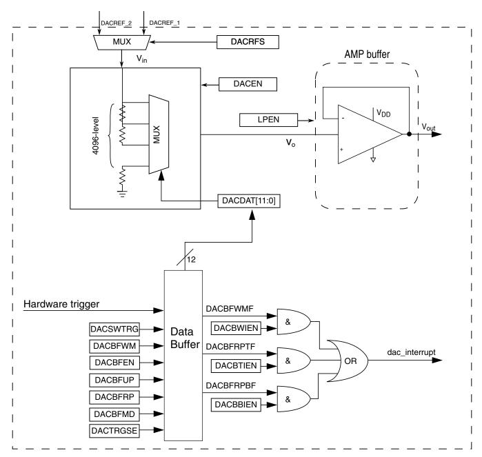
Figure 35-1. DAC block diagram
