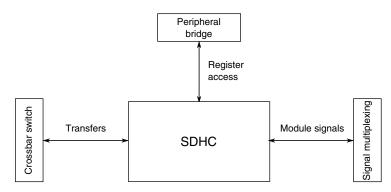
Figure 3-53. SDHC configuration
