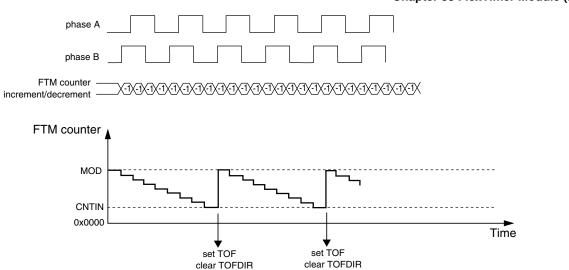
Figure 38-254. FTM counter overflow in down counting for Quadrature Decoder mode
