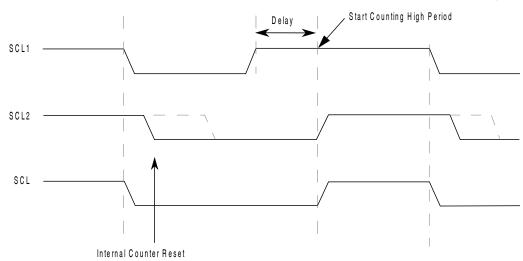
Figure 45-39. I2C clock synchronization
