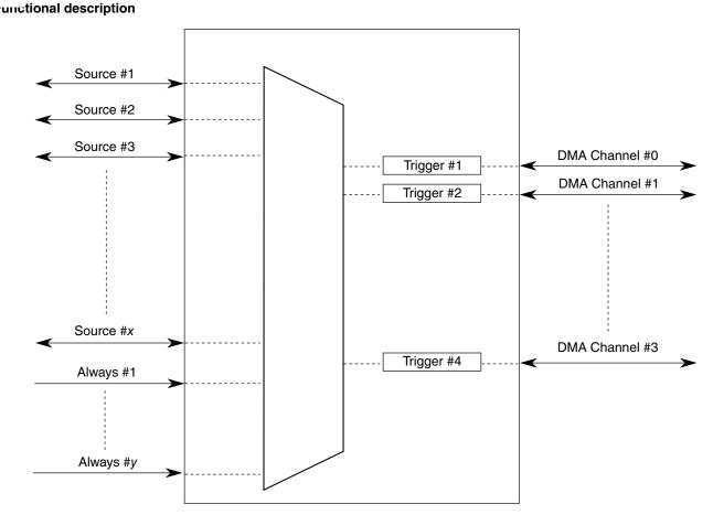
Figure 21-19. DMA MUX triggered channels
