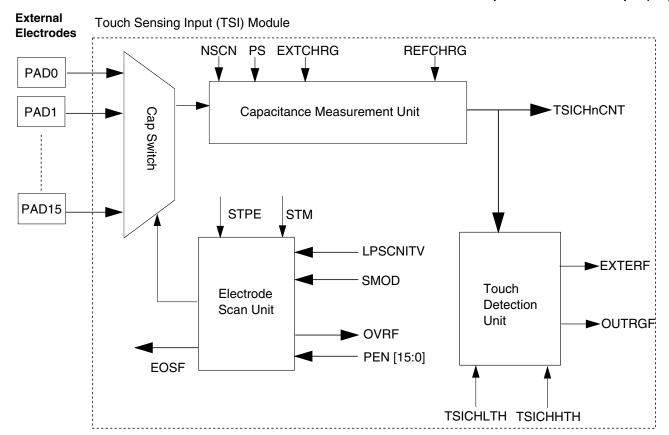
Figure 50-1. TSI block diagram
