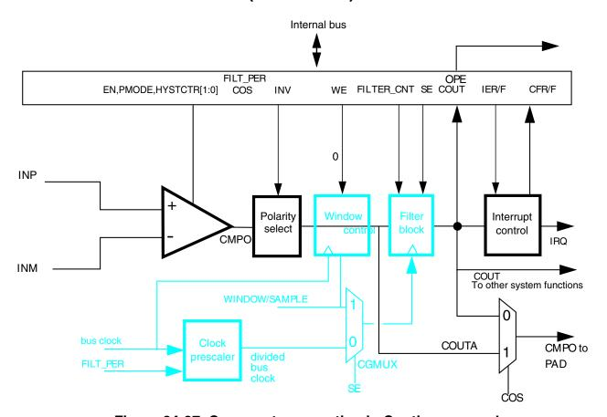
Figure 34-27. Comparator operation in Continuous mode
