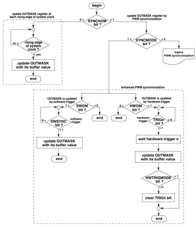
Figure 38-214. OUTMASK register synchronization flowchart
