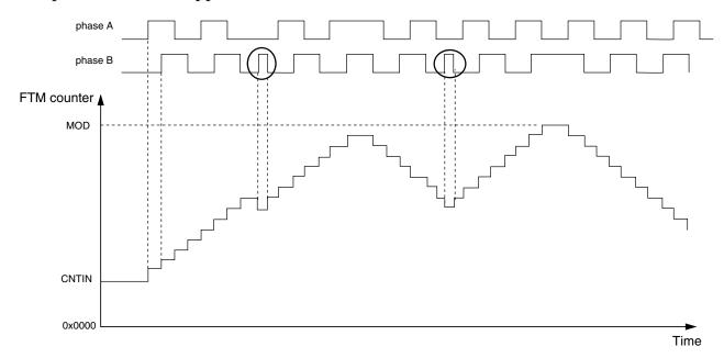
Figure 38-255. Motor position jittering in a mid count value
