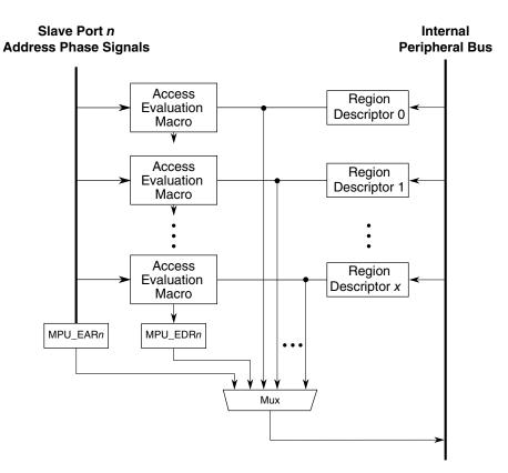
Figure 19-1. MPU block diagram
