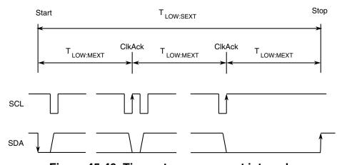
Figure 45-40. Timeout measurement intervals
