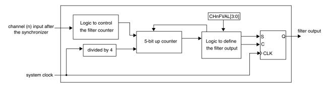
Figure 38-176. Channel input filter
