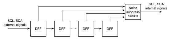
Figure 45-41. Programmable input glitch filter diagram
