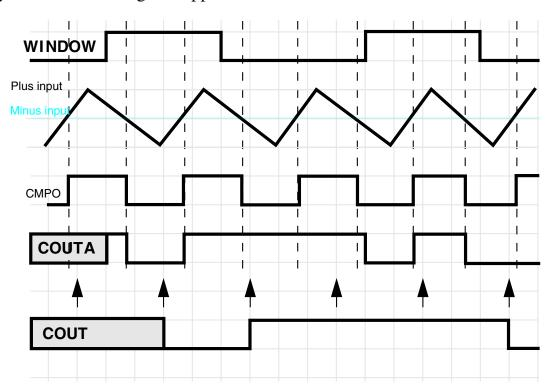
Figure 34-34. Windowed/resampled mode operation
