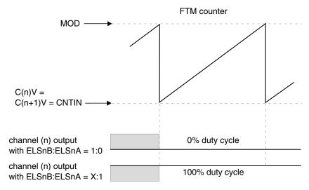
Figure 38-195. Channel (n) output if (C(n)V = C(n+1)V = CNTIN)
