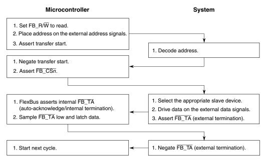
Figure 30-25. Read Cycle Flowchart
