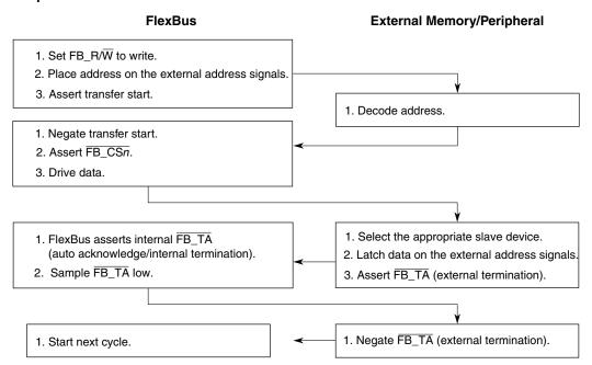
Figure 30-27. Write-Cycle Flowchart
