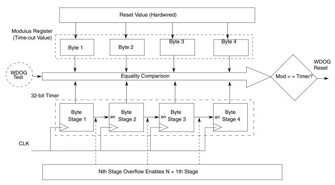
Figure 24-2. Watchdog timer byte splitting
