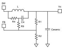
Figure11—Simplified Circuit of Ceramic Capacitor
