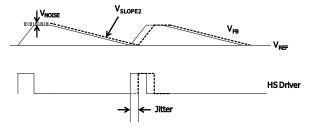
Figure 5—Jitter in Skip Mode
