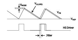
Figure 4—Jitter in PWM Mode
