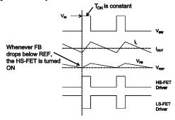
Figure 2—Heavy Load Operation
