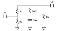
Figure 8—Simplified Circuit in skip Mode
