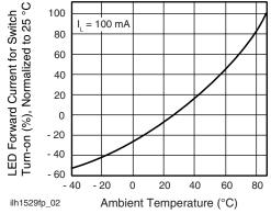
Fig. 2 - LED Current for Switch Turn-on vs. Temperature
