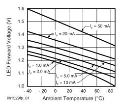
Fig. 1 - LED Voltage vs. Temperature
