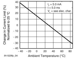
Fig. 4 - Current Limit vs. Temperature
