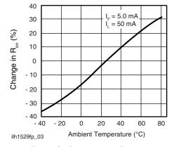
Fig. 3 - On-Resistance vs. Temperature
