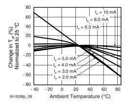
Fig. 9 - Turn-off Time vs. Temperature
