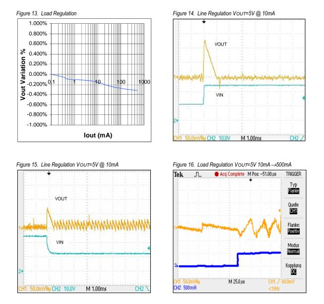
Note: All measurements taken at VIN=24V, VOUT=3.3V, and TAMB=25°C using the typical application circuit specified in Figure 17, unless otherwise specified.
