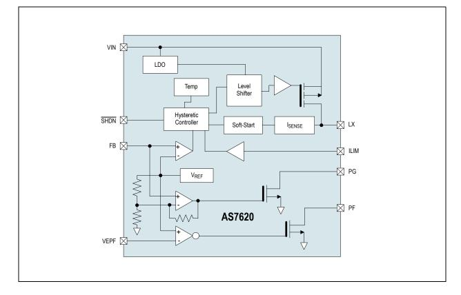
Figure 1. AS7620 - Block Diagram
