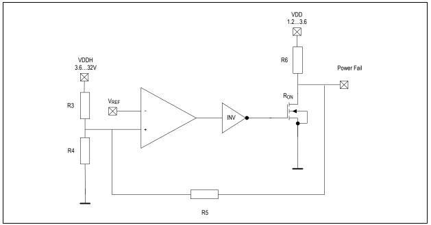
Table 5 provides the resistors values covering all the standard input BUS. The resistors values are 1% commercial values. It is mandatory to use the correct resistors values to guarantee the respect of maximum absolute voltages at EPF and PF pin. VDD has been considered 3.3V. Otherwise EPF pin should be shorted to GND and PF left floating.
