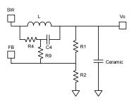
Figure11—Simplified Circuit of Ceramic Capacitor
