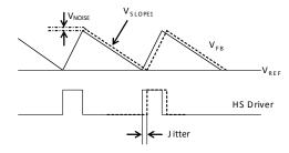
Figure 4—Jitter in PWM Mode
