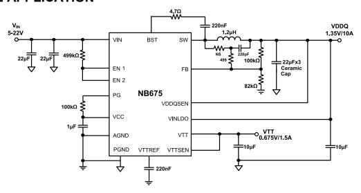
Figure 14 — Typical Application Circuit with Low ESR Ceramic Output Capacitor  $V_{\text{IN}}$ =5-22V,  $V_{\text{OUT}}$ =1.35V,  $I_{\text{OUT}}$ =10A
