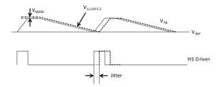
Figure 5—Jitter in Skip Mode
