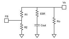
Figure 8—Simplified Circuit in skip Mode
