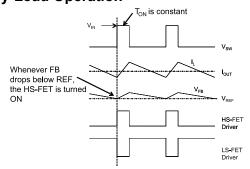
Figure 2—Heavy Load Operation
