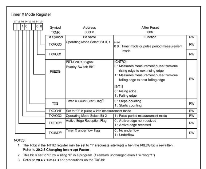
Figure 13.9 TXMR Register in Pulse Period Measurement Mode
