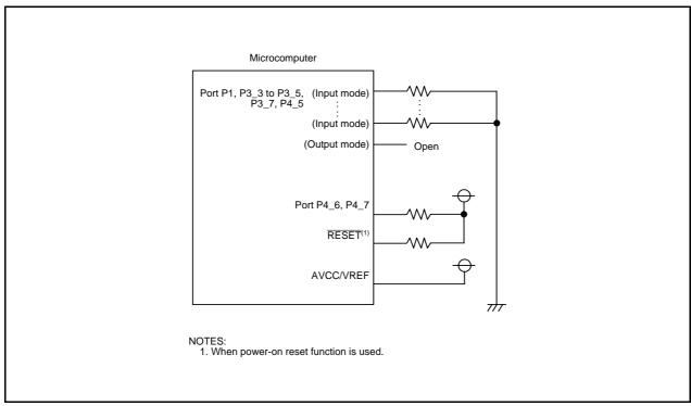
Figure 17.9 Unassigned Pin Handling
