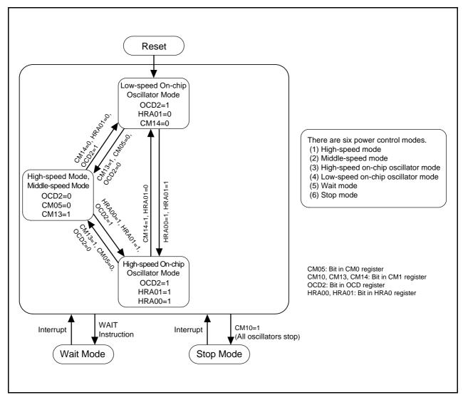
Figure 9.8 State Transition of Power Control
