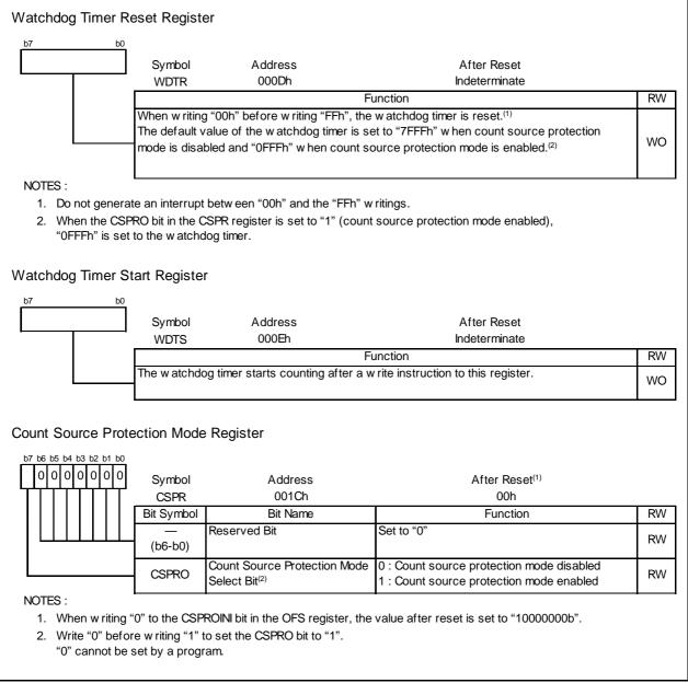
Figure 12.3 WDTR, WDTS and CSPR Registers
