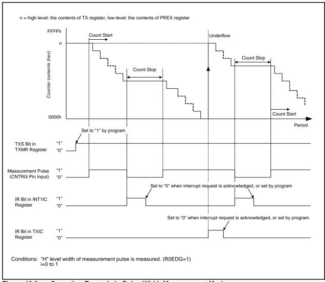
Figure 13.8 Operating Example in Pulse Width Measurement Mode
