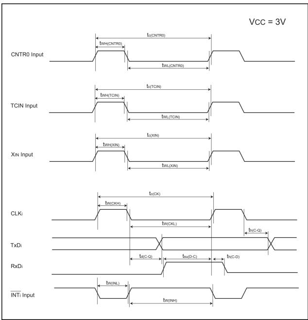
Figure 19.8 Timing Diagram When Vcc = 3V
