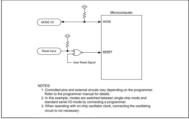
Figure 18.17 Pin Process in Standard Serial I/O Mode 3
