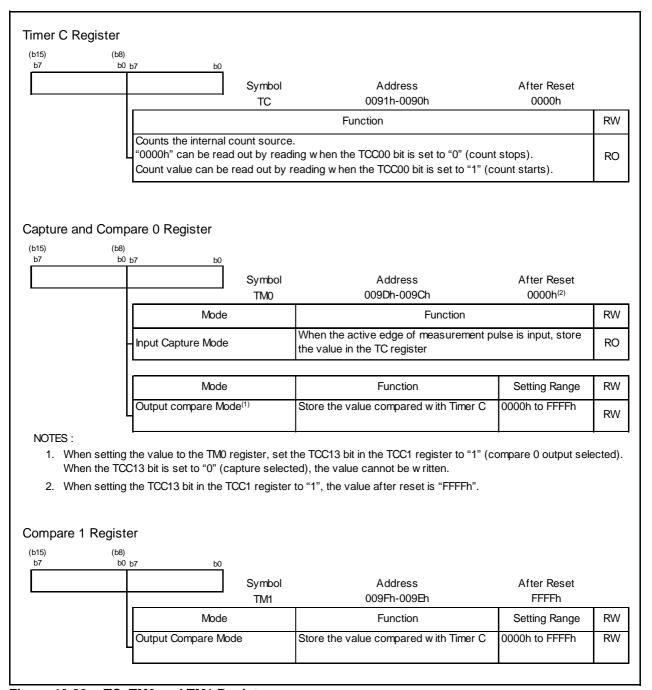
Figure 13.26 TC, TM0 and TM1 Registers
