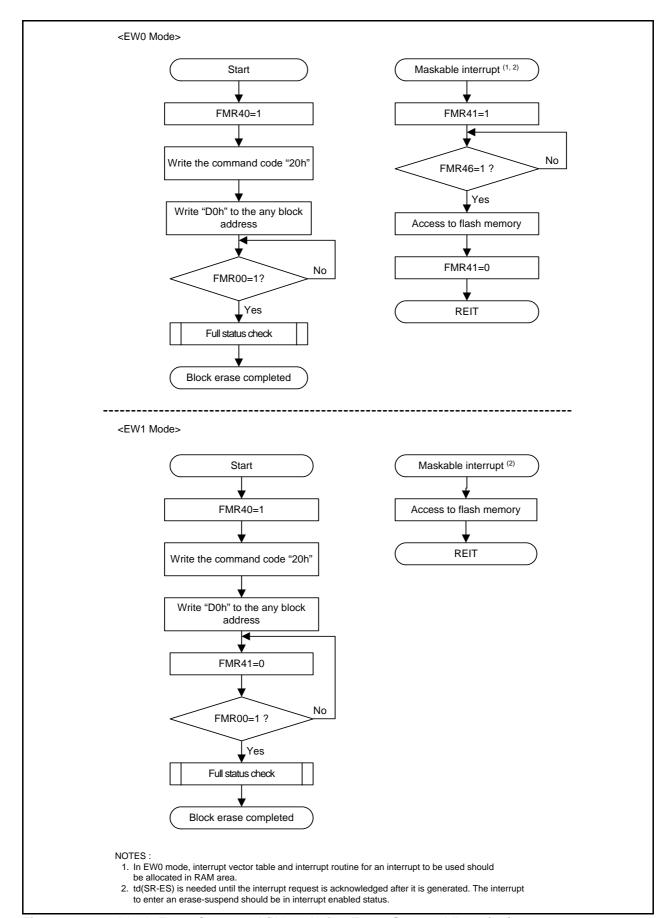
Figure 18.13 Block Erase Command (When Using Erase-Suspend Function)
