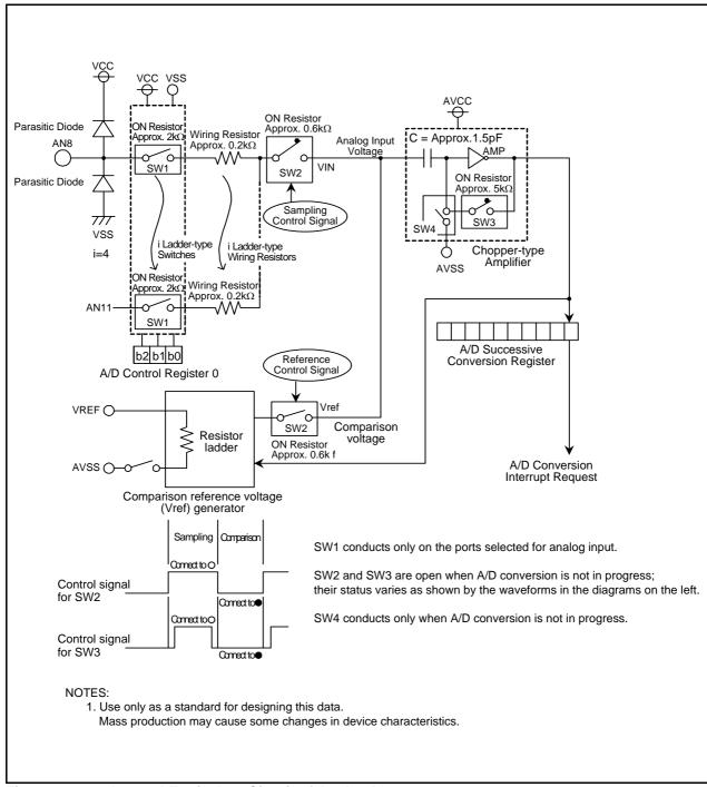
Figure 16.8 Internal Equivalent Circuit of Analog Input
