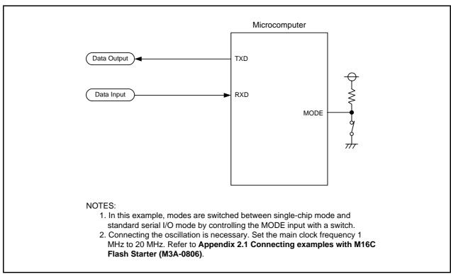
Figure 18.16 Pin Process in Standard Serial I/O Mode 2
