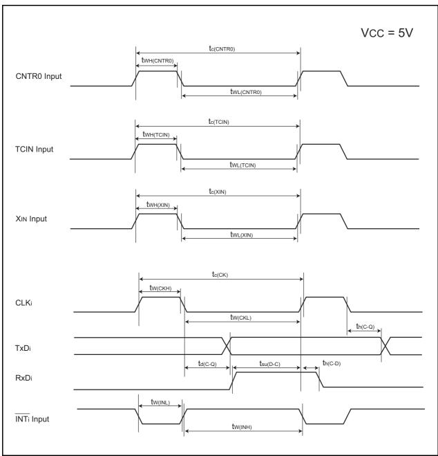
Figure 19.7 Timing Diagram When Vcc = 5V
