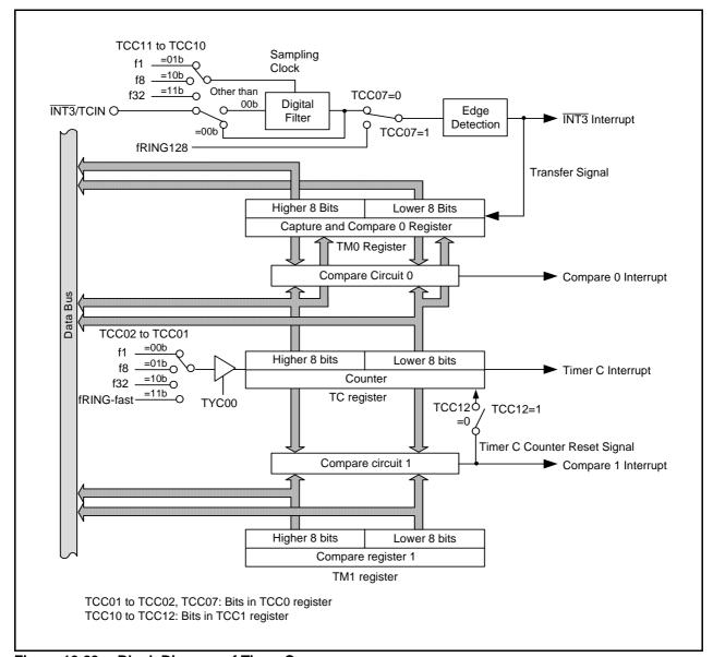
Figure 13.23 Block Diagram of Timer C
