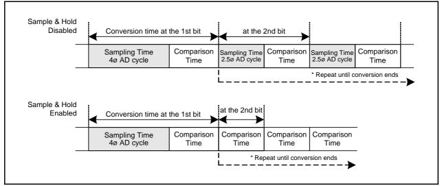
Figure 16.6 Timing Diagram of A/D Conversion
