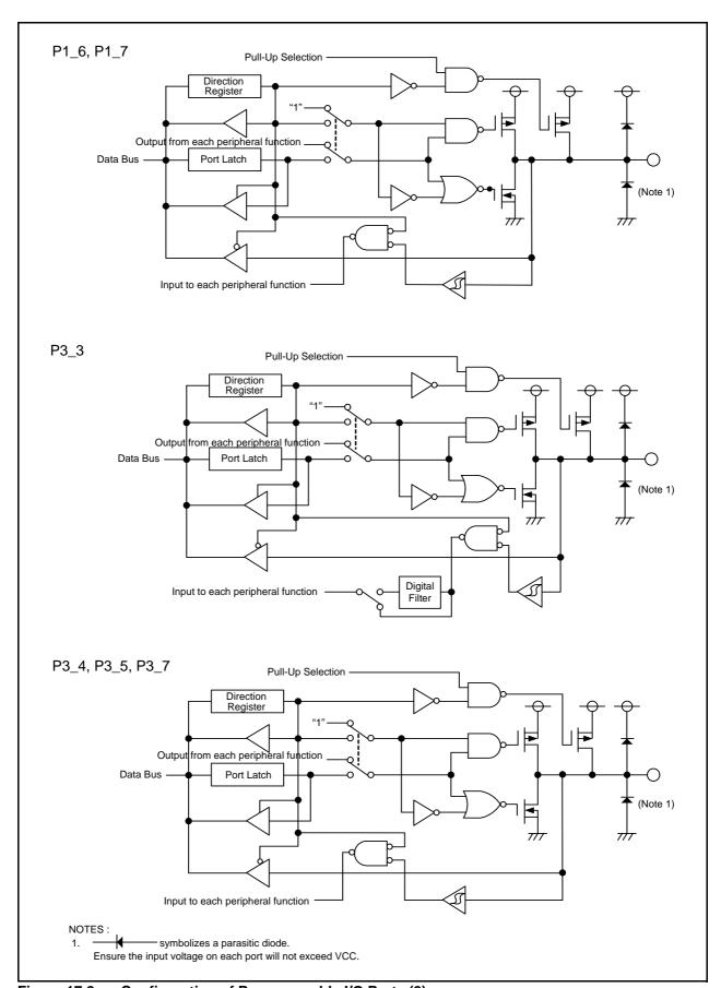
Figure 17.2 Configuration of Programmable I/O Ports (2)
