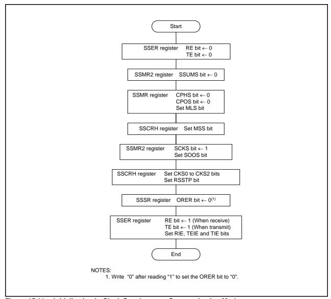
Figure 15.11 Initialization in Clock Synchronous Communication Mode
