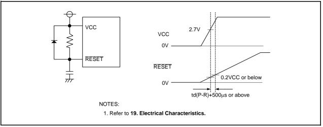
Figure 5.4 Example of Hardware Reset Circuit and Operation
