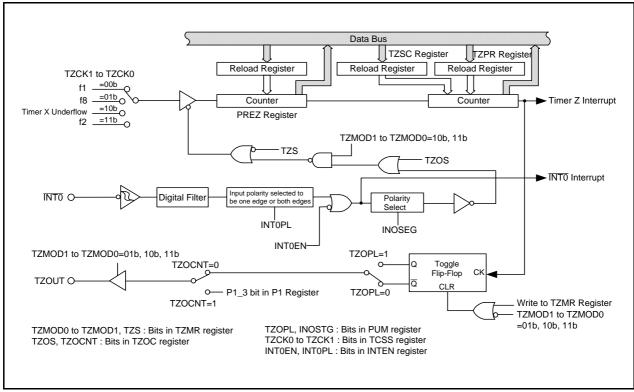
Figure 13.11 Block Diagram of Timer Z
