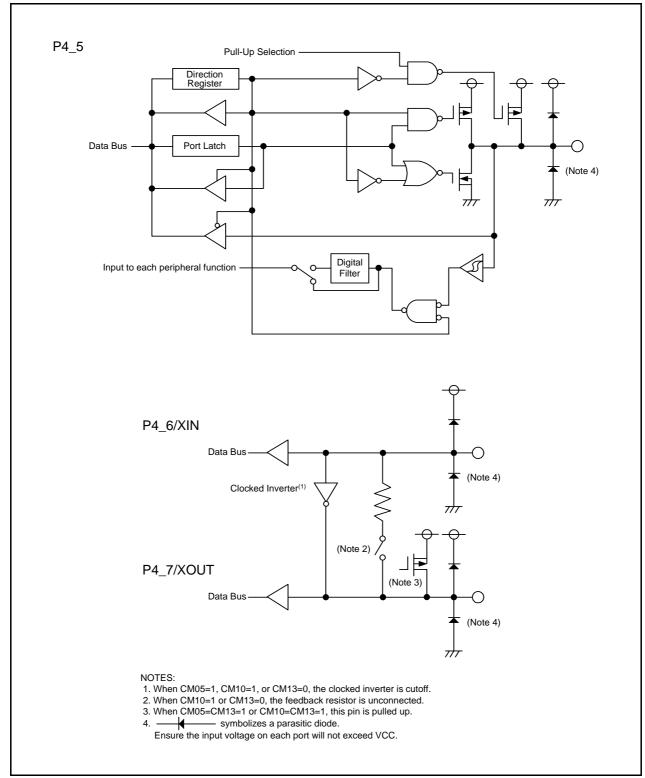
Figure 17.3 Configuration of Programmable I/O Ports (3)
