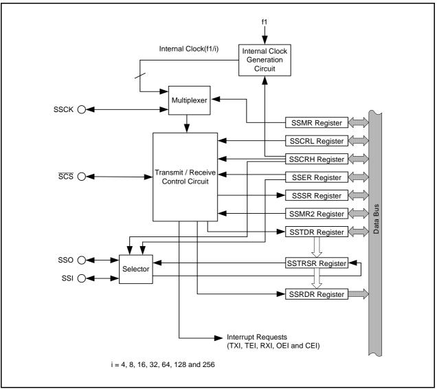
Figure 15.1 **Block Diagram of SSU**
