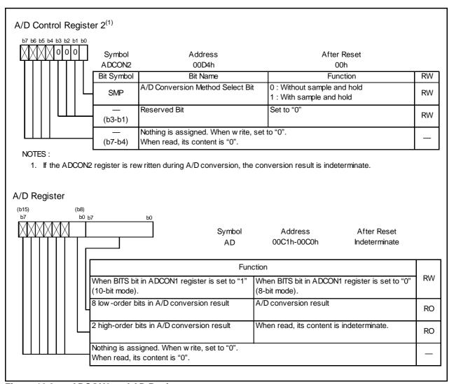
Figure 16.3 **ADCON2 and AD Registers**
