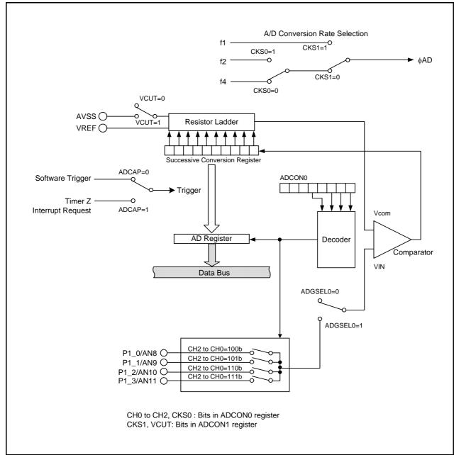
Figure 16.1 Block Diagram of A/D Converter
