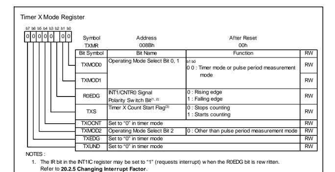
Figure 13.4 TXMR Register in Timer Mode
