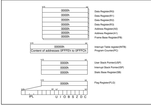
Figure 5.2 CPU Register Status after Reset
