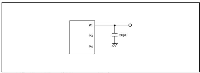
Figure 19.1 Port P1, P3 and P4 Measurement Circuit
