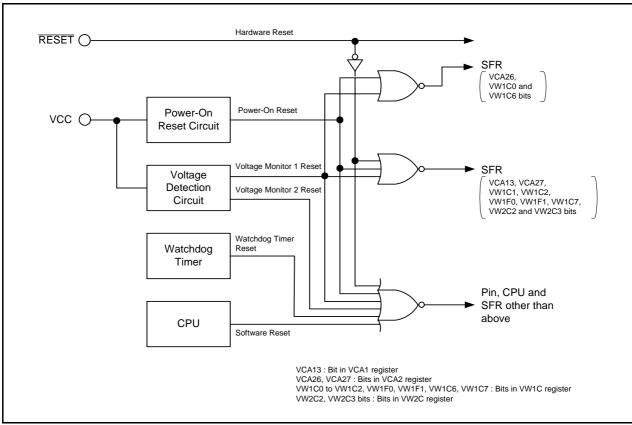
Figure 5.1 Block Diagram of Reset Circuit
