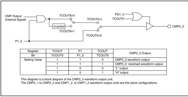
Figure 13.25 Block Diagram of CMP Waveform Output Unit
