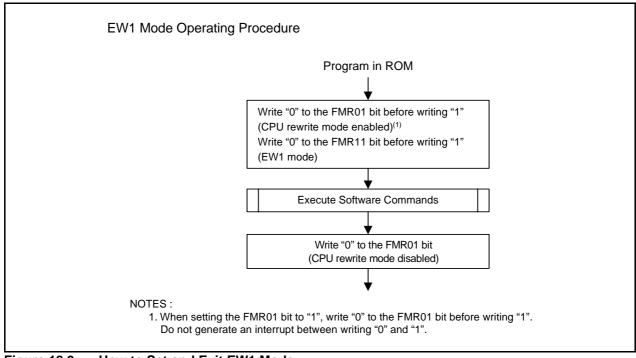
Figure 18.9 How to Set and Exit EW1 Mode
