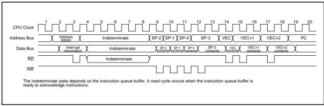
Figure 11.5 Time Required for Executing Interrupt Sequence
