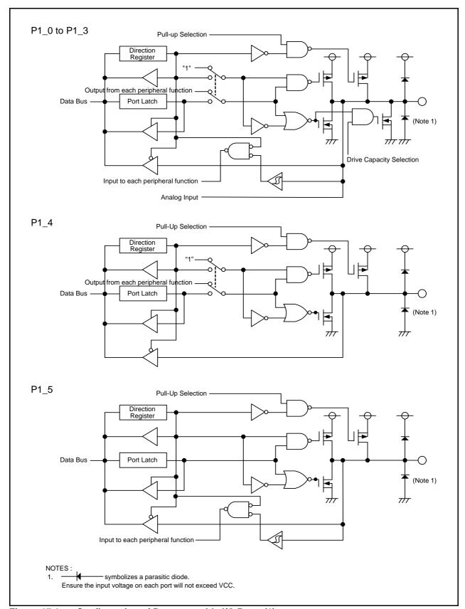
Figure 17.1 Configuration of Programmable I/O Ports (1)
