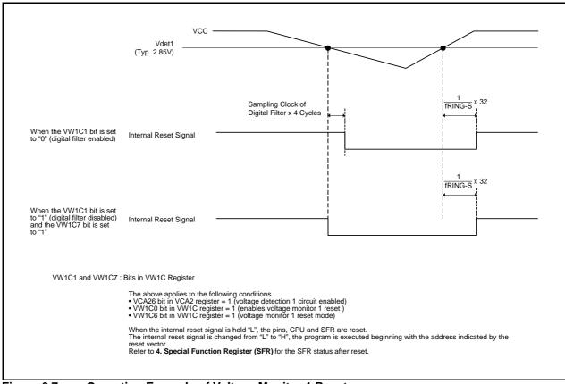
Figure 6.7 Operating Example of Voltage Monitor 1 Reset
