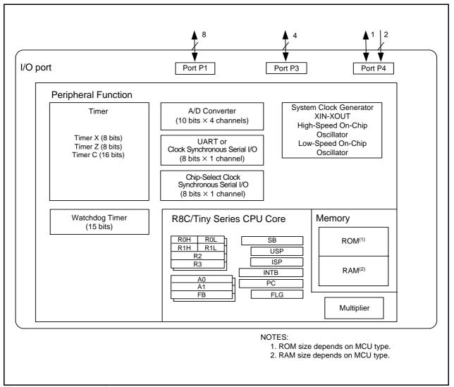
Figure 1.1 Block Diagram
