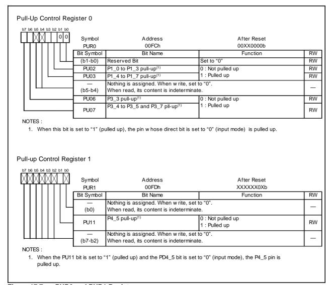
Figure 17.7 PUR0 and PUR1 Registers
