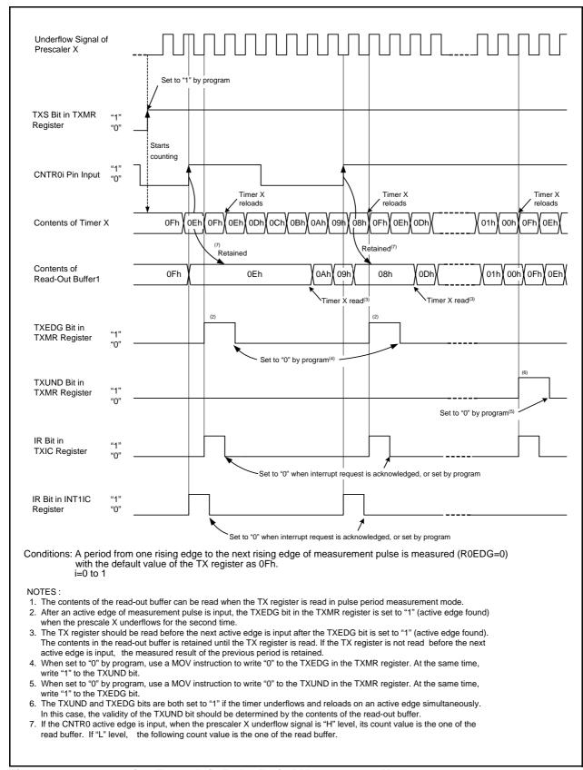
Figure 13.10 Operating Example in Pulse Period Measurement Mode
