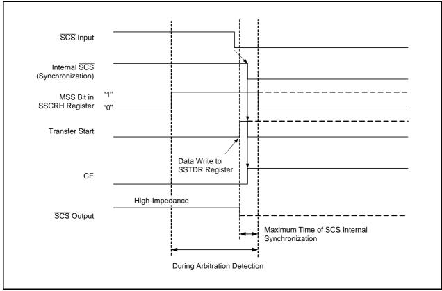
Figure 15.20 Arbitration Check Timing
