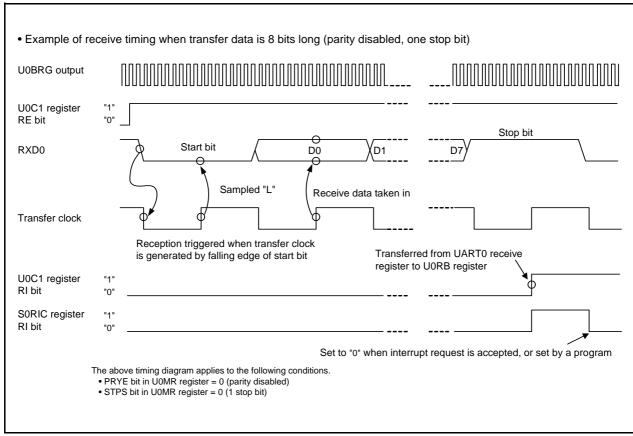
Figure 14.10 Receive Timing in UART Mode
