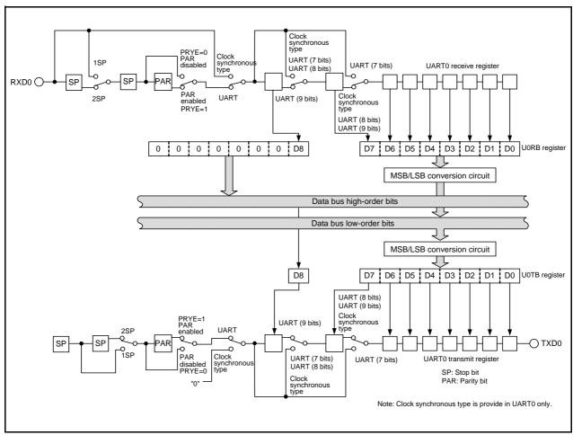
Figure 14.2 UART0 Transmit/Receive Unit
