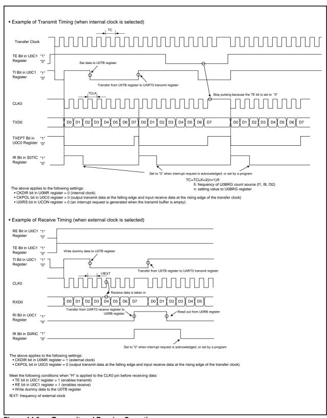
Figure 14.6 Transmit and Receive Operation
