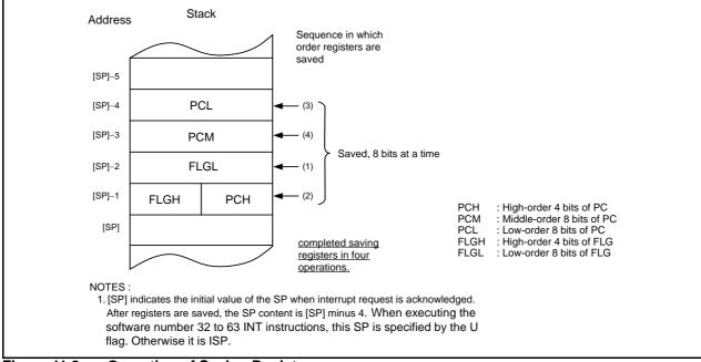
Figure 11.8 Operation of Saving Register
