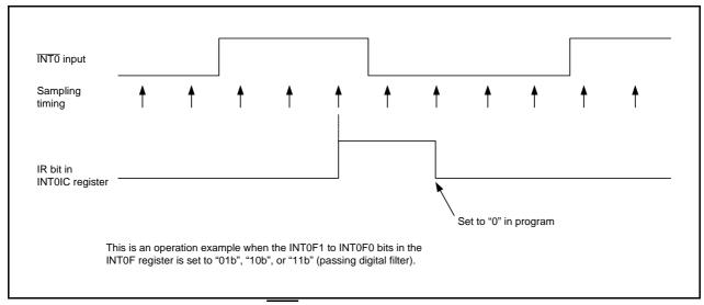
**Figure 11.13 Operating Example of INTO Input Filter**
