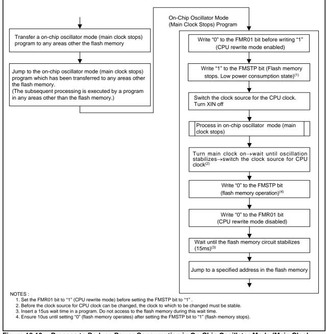
**Figure 18.10** Process to Reduce Power Consumption in On-Chip Oscillator Mode (Main Clock Stops)
