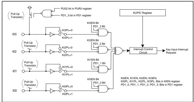
Figure 11.17 Block Diagram of Key Input Interrupt
