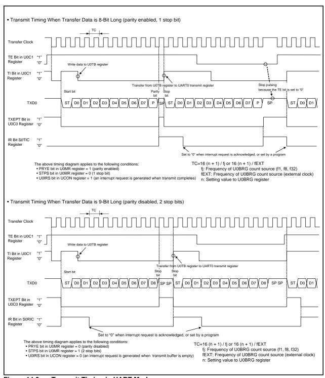
Figure 14.9 Transmit Timing in UART Mode
