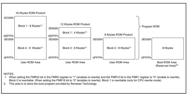
Figure 18.1 Flash Memory Block Diagram for R8C/14 Group
