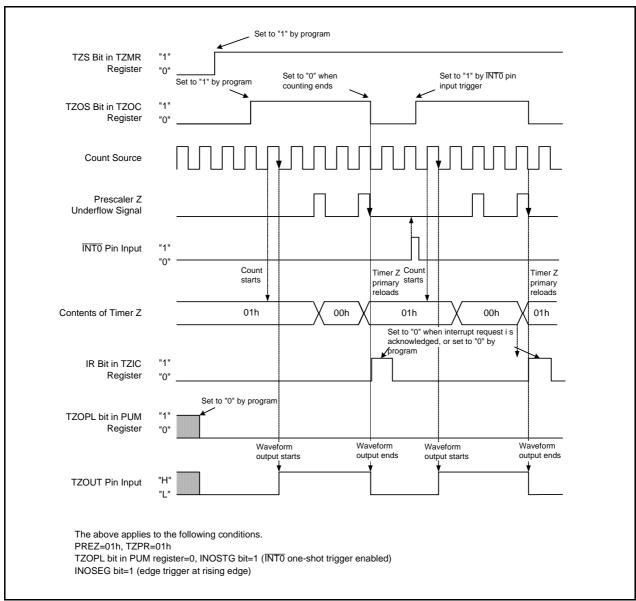
Figure 13.20 Operating Example in Programmable One-Shot Generation Mode
