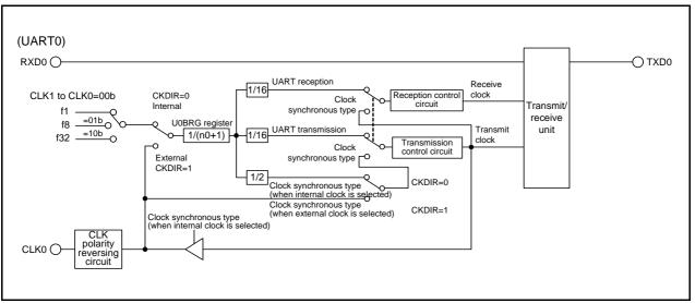
Figure 14.1 UART0 Block Diagram
