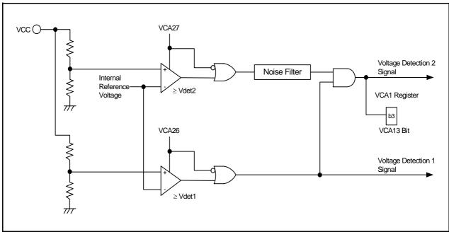
Figure 6.1 Block Diagram of Voltage Detection Circuit
