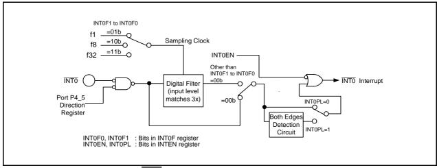
**Figure 11.12 Configuration of INTO Input Filter**
