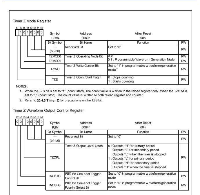
Figure 13.17 TZMR and PUM Registers in Programmable Waveform Generation Mode
