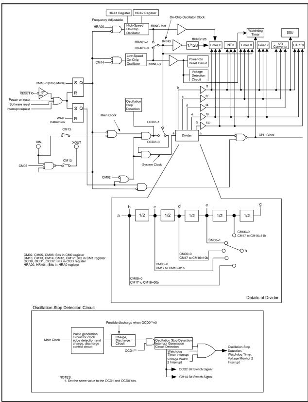
Figure 9.1 **Clock Generation Circuit**
