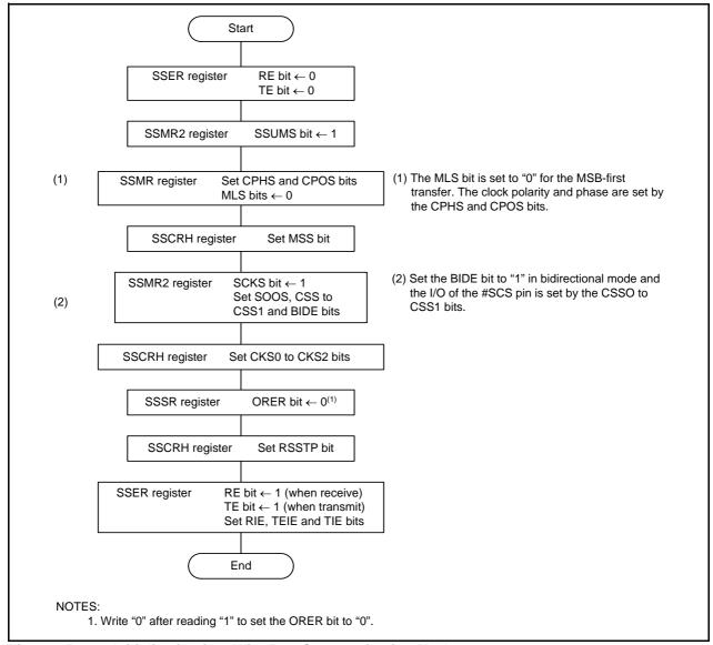
Figure 15.17 Initialization in 4-Wire Bus Communication Mode
