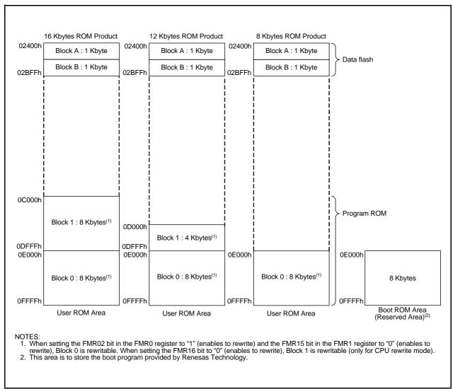
Figure 18.2 Flash Memory Block Diagram for R8C/15 Group
