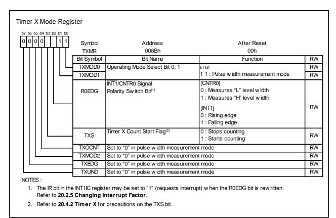
Figure 13.7 TXMR Register in Pulse Width Measurement Mode
