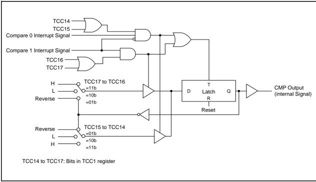
Figure 13.24 Block Diagram of CMP Waveform Generation Unit
