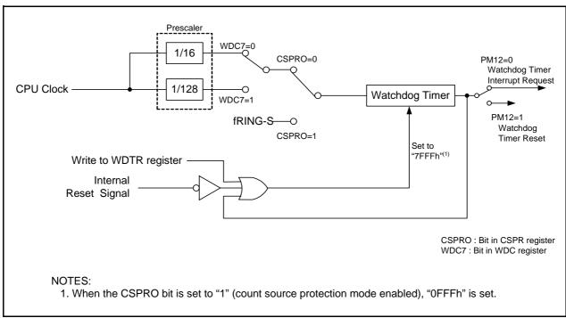
Figure 12.1 Block Diagram of Watchdog Timer
