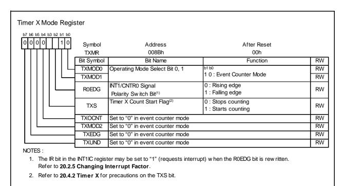
Figure 13.6 **TXMR Register in Event Counter Mode**
