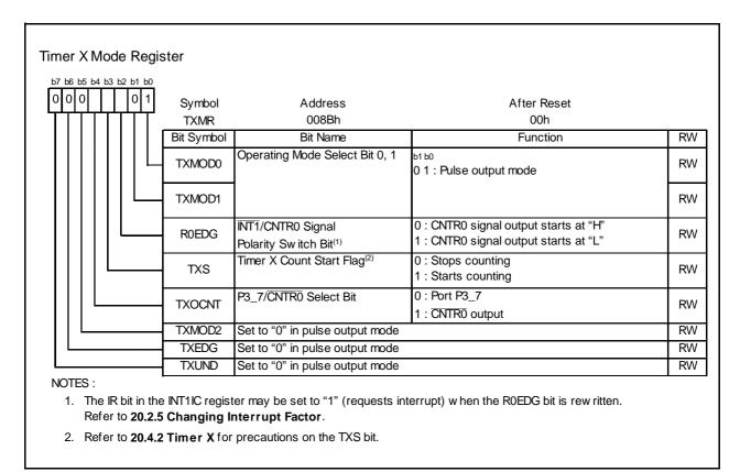
Figure 13.5 **TXMR Register in Pulse Output Mode**
