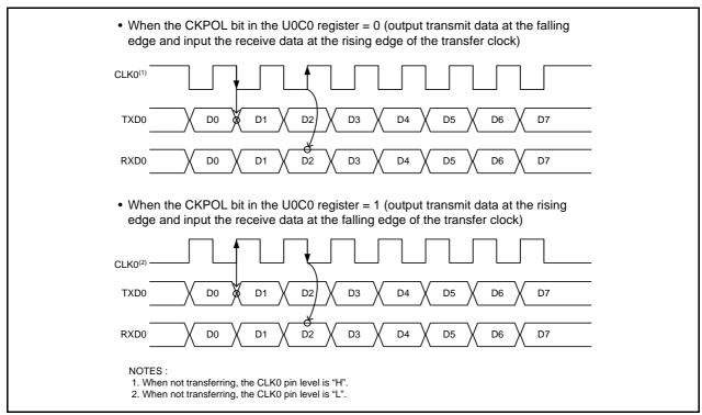
Figure 14.7 Transfer Clock Polarity
