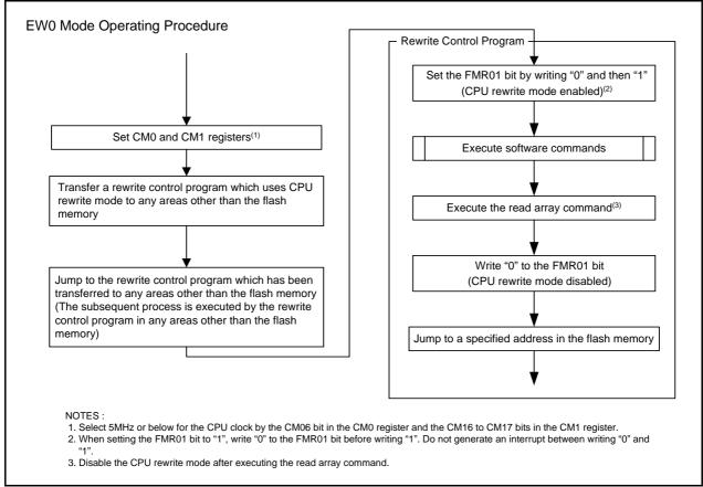
Figure 18.8 How to Set and Exit EW0 Mode
