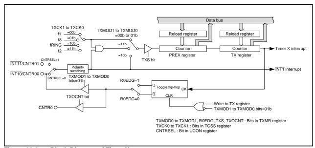
Figure 13.1 Block Diagram of Timer X
