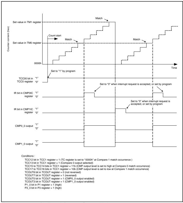
Figure 13.31 Operating Example in Output Compare Mode
