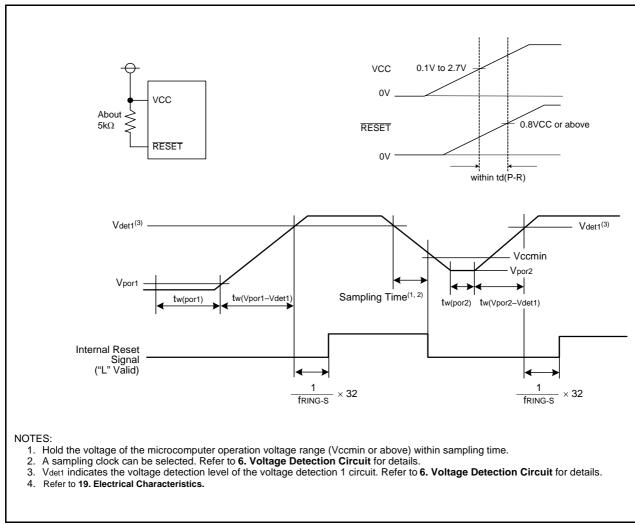
Figure 5.6 Example of Power-On Reset Circuit and Operation
