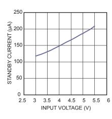
Disabled Supply Current vs. Input Voltage
