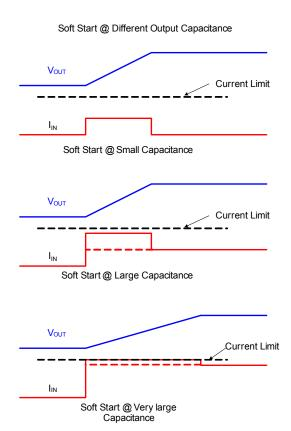
Figure 3: Soft Start Periods at Different Output Capacitance
