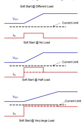
Figure 2: Soft Start Periods at Different Load
