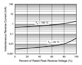
Fig. 4 - Typical Reverse Characteristics
