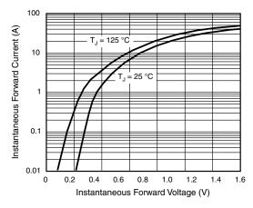
Fig. 3 - Typical Instantaneous Forward Characteristics
