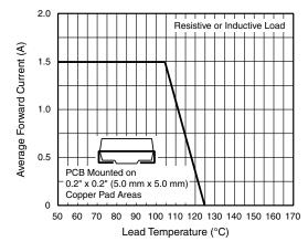
Fig. 1 - Forward Current Derating Curve
