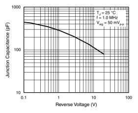
Fig. 5 - Typical Junction Capacitance
