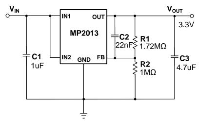
Figure 8: 3.3V Output with Feedforward Capacitor
