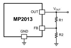
Figure 2: FB Resistor Divider to Set Vout
