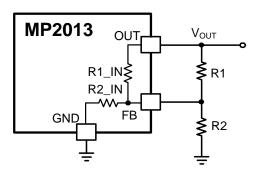
Figure 3: FB Divider of Fixed Output Version
