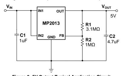
Figure 9: 5V Output Typical Application Circuit
