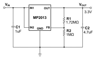
Figure 7: 3.3V Output Typical Application Circuit
