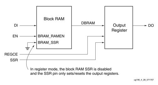
Figure 4-11: Block RAM SSR in Register Mode
