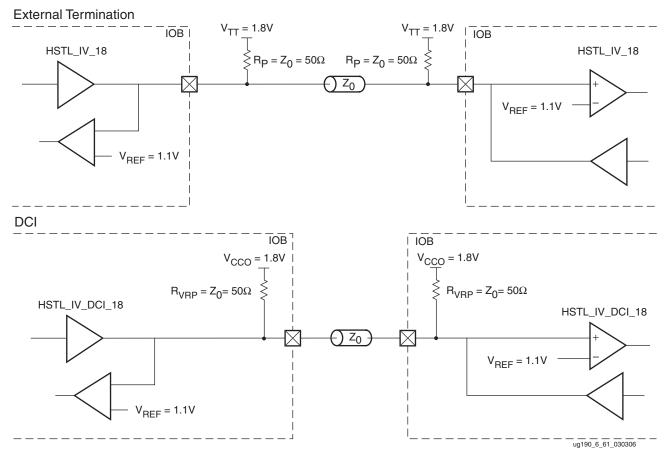
Figure 6-64: HSTL Class IV (1.8V) with Bidirectional Termination
