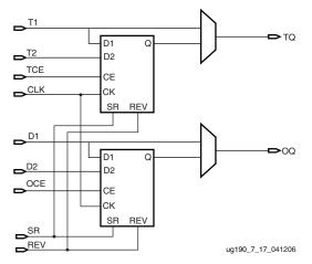
Figure 7-22: OLOGIC Block Diagram
