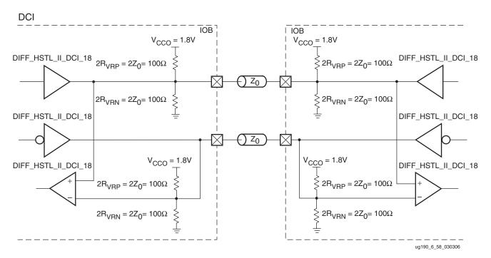
Figure 6-61 shows a sample circuit illustrating a valid termination technique for differential HSTL Class II (1.8V) with bidirectional DCI termination.
