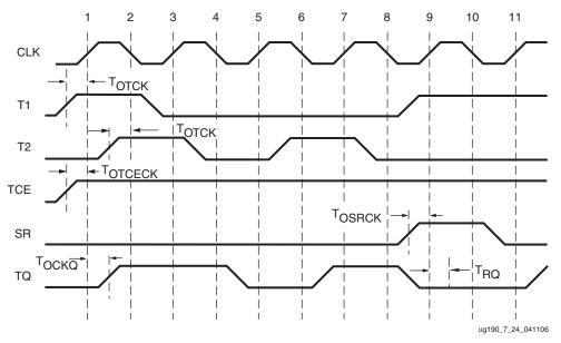
Figure 7-29: OLOGIC ODDR 3-State Register Timing Characteristics
