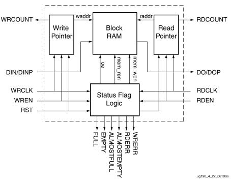
Figure 4-17: Top-Level View of FIFO in Block RAM
