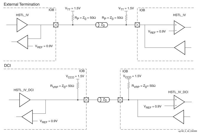
Figure 6-51 shows a sample circuit illustrating a valid bidirectional termination technique for HSTL Class IV.
