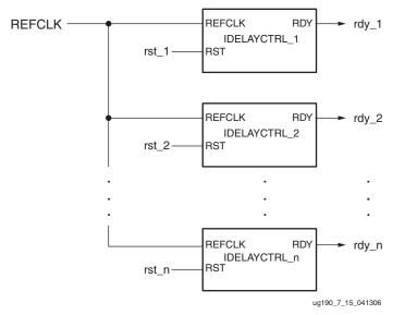
Figure 7-20: Instantiate IDELAYCTRL with LOC Constraint
