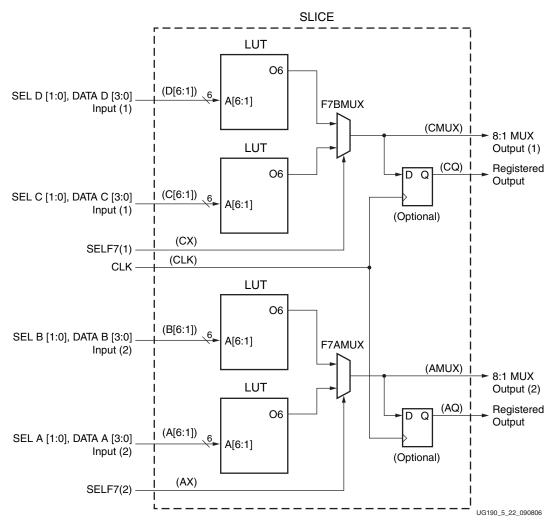
Figure 5-22: Two 8:1 Multiplexers in a Slice
