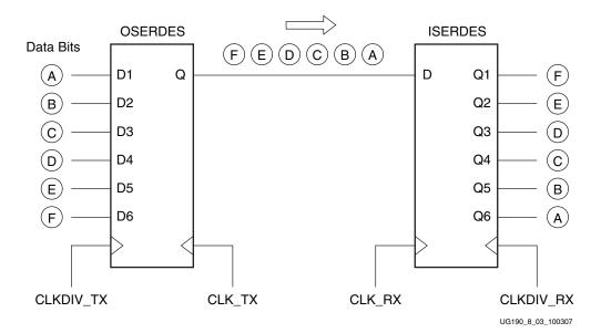
Figure 8-3: Bit Ordering on Q1–Q6 Outputs of ISERDES\_NODELAY Ports
