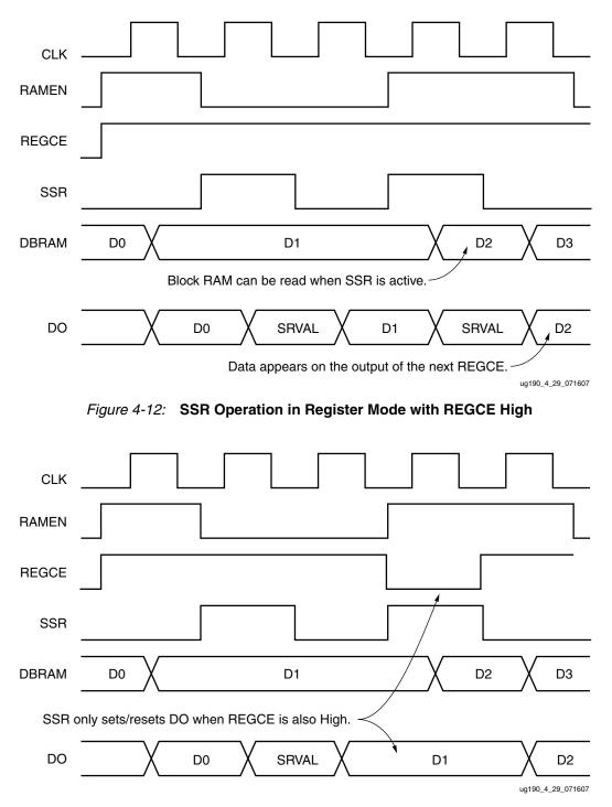
Figure 4-13: SSR Operation in Register Mode with Variable REGCE
