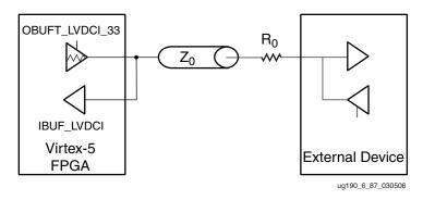
Figure 6-93: 3.3V I/O Configuration
