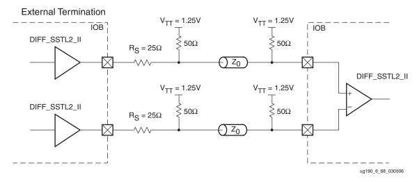
Figure 6-72: Differential SSTL2 Class II Unidirectional Termination
