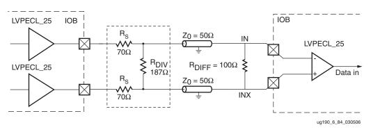
Figure 6-90: LVPECL Transmitter Termination
