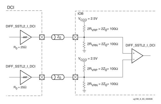
Figure 6-69 shows a sample circuit illustrating a valid termination technique for differential SSTL2 Class I (2.5V) with unidirectional DCI termination.
