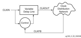
Figure 2-3: Simplified DLL Circuit
