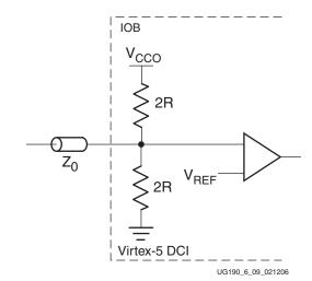
Figure 6-11 illustrates split termination inside a Virtex-5 device.
