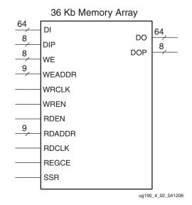
Figure 4-6: Simple Dual-Port Data Flow
