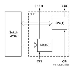
Figure 5-1: Arrangement of Slices within the CLB
