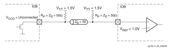
Figure 6-38: GTL+ with External Parallel Termination and Unconnected V<sub>CCO</sub>
