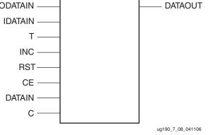
Figure 7-8: IODELAY Primitive
