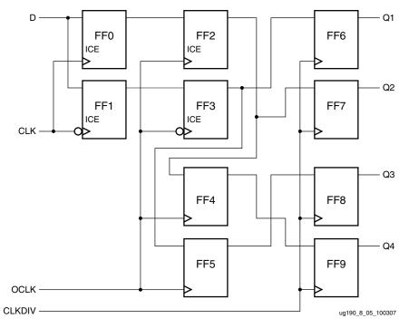
Figure 8-5: Internal Connections of ISERDES\_NODELAY When in Memory Mode
