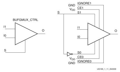
Figure 1-11: BUFGMUX\_CTRL as BUFGCTRL
