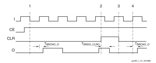
*Figure 1-21:* **BUFR Timing Diagrams with BUFR\_DIVIDE Values**
