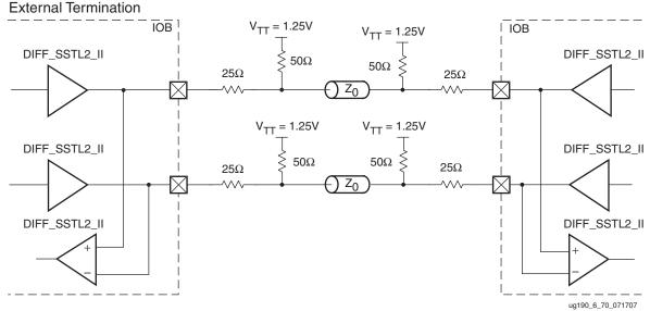
Figure 6-74: Differential SSTL2 (2.5V) Class II with Bidirectional Termination
