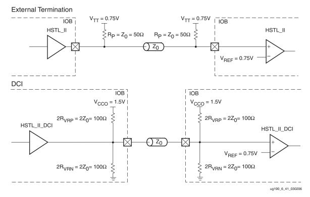
Figure 6-43: HSTL (1.5V) Class II Unidirectional Termination
