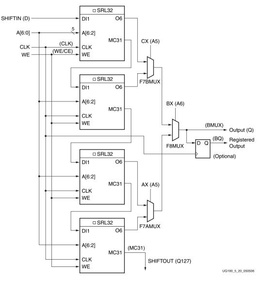
Figure 5-20: 128-bit Shift Register Configuration
