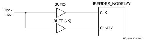
Figure 8-6: Clocking Arrangement Using BUFIO and BUFR
