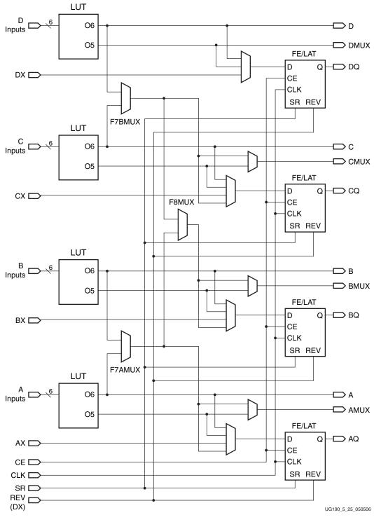
Figure 5-25: Simplified Virtex-5 FPGA Slice
