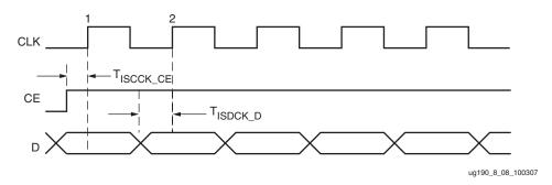
Figure 8-8: ISERDES Input Data Timing Diagram
