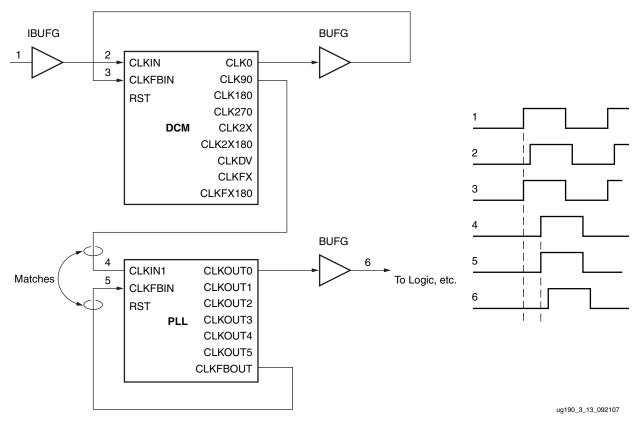
Figure 3-13: DCM Driving a PLL
