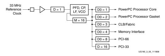
Figure 3-5: PLL as a Frequency Synthesizer
