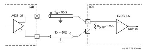
*Figure 6-88:* LVDS\_25 With DIFF\_TERM Receiver Termination
