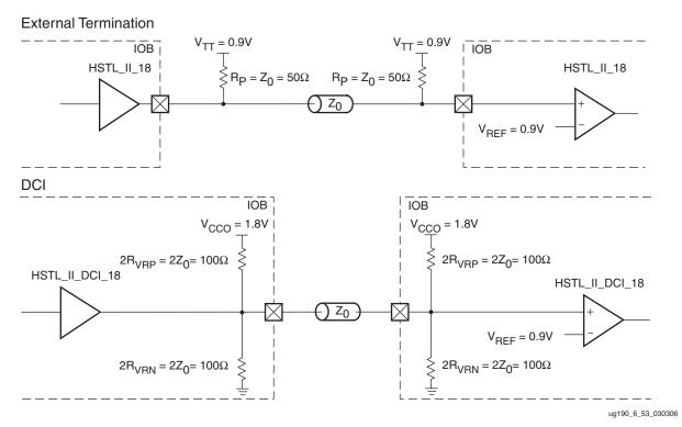
Figure 6-56: HSTL Class II (1.8V) with Unidirectional Termination
