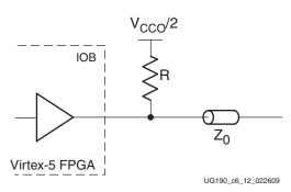
Figure 6-14: Driver with Termination to V<sub>CCO</sub>/2 without DCI
