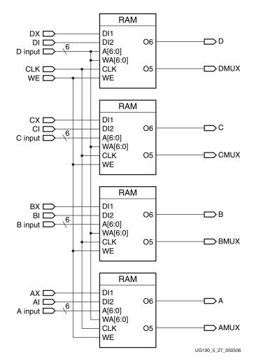
Figure 5-27: Simplified Virtex-5 FPGA SLICEM Distributed RAM
