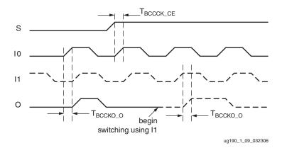
Figure 1-9: BUFGMUX Timing Diagram
