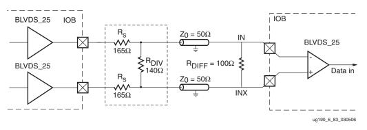
Figure 6-89: BLVDS Transmitter Termination
