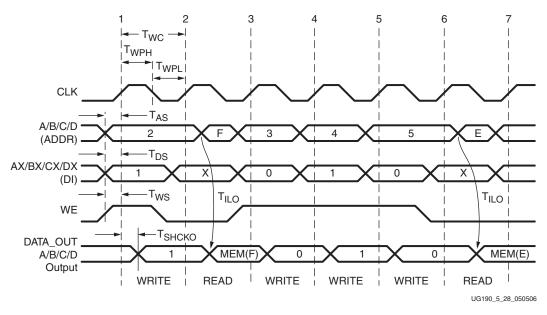
Figure 5-28: Slice Distributed RAM Timing Characteristics
