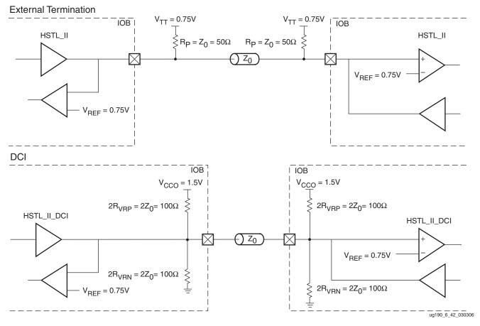
Figure 6-44: HSTL (1.5V) Class II Bidirectional Termination
