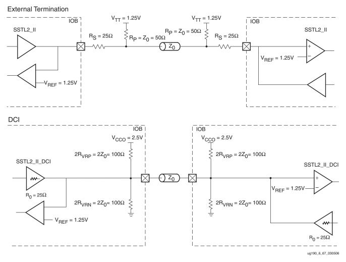
Figure 6-71: SSTL2 Class II with Bidirectional Termination
