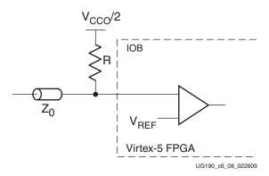
Figure 6-10: Input Termination to V<sub>CCO</sub>/2 without DCI
