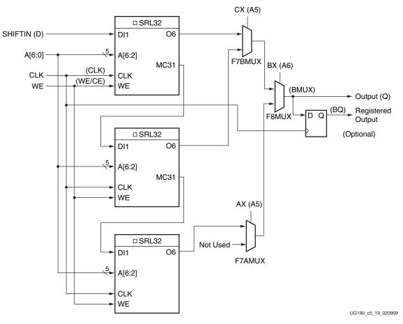
Figure 5-19: 96-bit Shift Register Configuration
