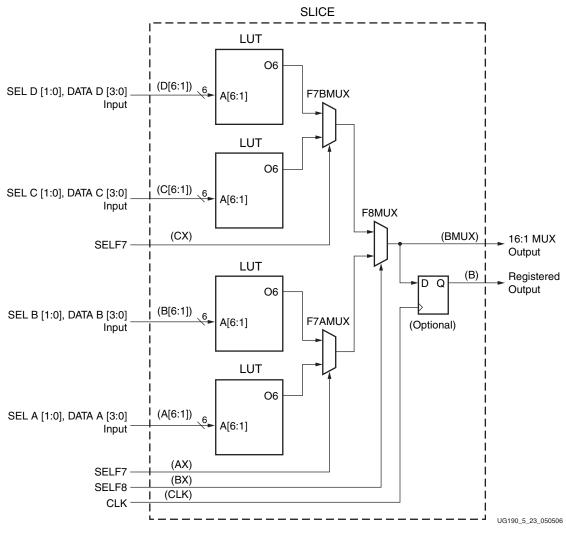
Figure 5-23: 16:1 Multiplexer in a Slice
