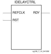
Figure 7-15: IDELAYCTRL Primitive
