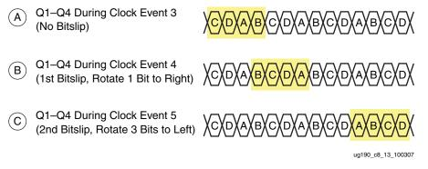
*Figure 8-13:* Bits from Data Input Stream (D) of Figure 8-12
