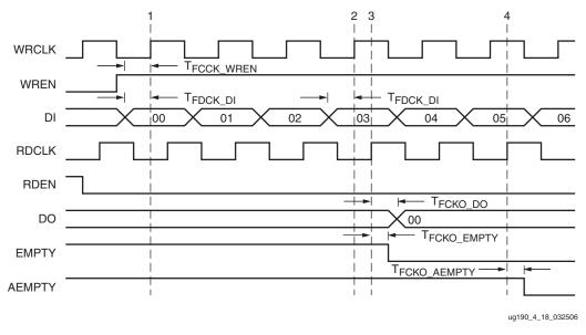
Figure 4-21: Writing to an Empty FIFO in FWFT Mode
