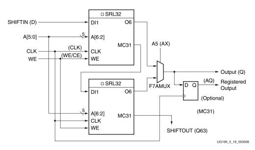
Figure 5-18: 64-bit Shift Register Configuration
