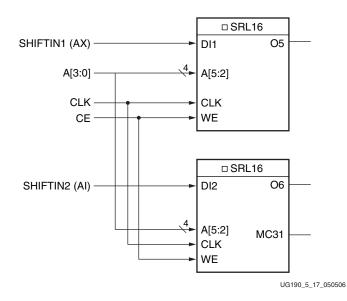
Figure 5-17 shows two 16-bit shift registers. The example shown can be implemented in a single LUT.
