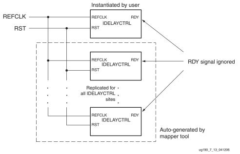
Figure 7-18: Instantiate IDELAYCTRL Without LOC Constraints - RDY Unconnected
