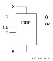
Figure 7-5: IDDR Primitive Block Diagram
