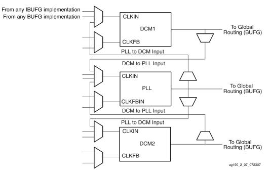
Figure 2-7: DCM and PLL Connection in Same CMT Block
