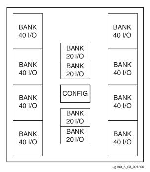
Figure 6-3: Virtex-5 FPGA XC5VLX30 I/O Banks
