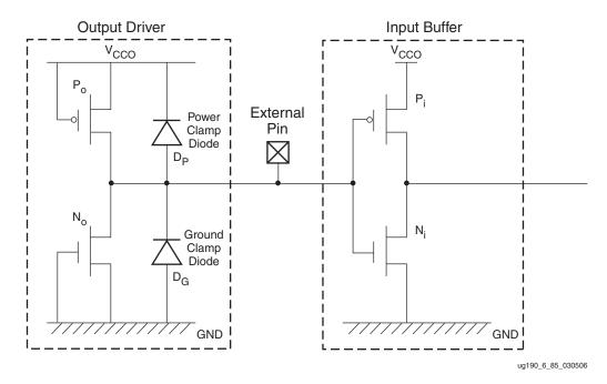
Figure 6-91: Virtex-5 FPGA I/O: 3-State Output Driver
