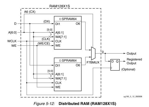
If two single-port 128 x 1-bit modules are built, the two RAM128X1S primitives can occupy a SLICEM, as long as they share the same clock, write enable, and shared read and write port address inputs. This configuration equates to 128 x 2-bit single-port distributed RAM.
