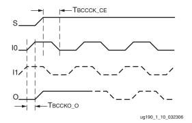
Figure 1-10: BUFGMUX\_1 Timing Diagram
