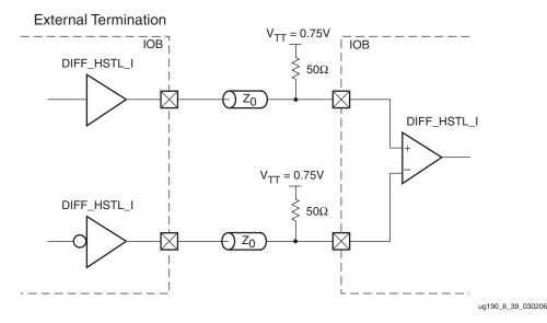
*Figure 6-41:* Differential HSTL (1.5V) Class I Unidirectional Termination
