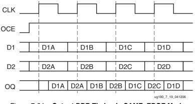
Figure 7-24: Output DDR Timing in SAME\_EDGE Mode
