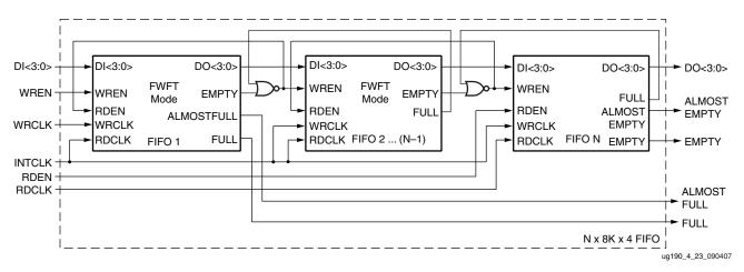
Figure 4-26: Example: Cascading Multiple FIFOs by Depth
