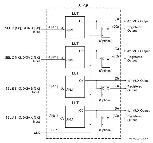
Figure 5-21: Four 4:1 Multiplexers in a Slice
