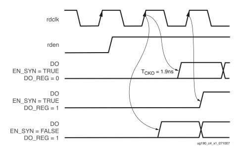
Figure 4-16: Synchronous FIFO Data Timing Diagram
