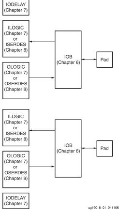
Figure 6-1: Virtex-5 FPGA I/O Tile
