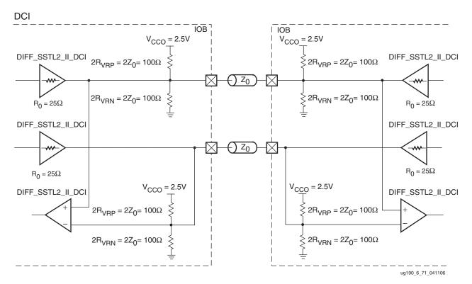
Figure 6-75 shows a sample circuit illustrating a valid termination technique for differential SSTL2 Class II (2.5V) with bidirectional DCI termination.
