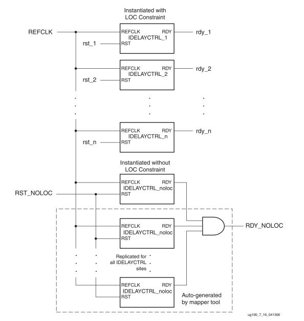
*Figure 7-21:* Mixed Instantiation of IDELAYCTRL Elements
