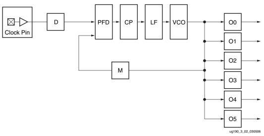
Figure 3-2: Block Diagram of the Virtex-5 FPGA PLL
