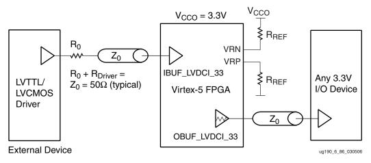
Figure 6-92: Connecting LVTTL or LVCMOS Using the LVDCI\_33 Standard
