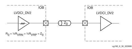
Figure 6-33: Controlled Impedance Driver with Half Impedance Unidirectional Termination
