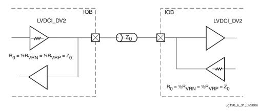
Figure 6-34: Controlled Impedance Driver with Half Impedance Bidirectional Termination
