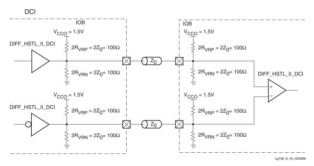
Figure 6-46 shows a sample circuit illustrating a valid termination technique for differential HSTL Class II (1.5V) with unidirectional DCI termination.
