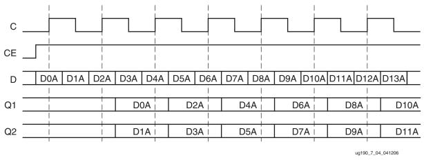
Figure 7-4: Input DDR Timing in SAME\_EDGE\_PIPELINED Mode
