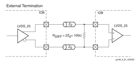
Figure 6-87: LVDS\_25 Receiver Termination
