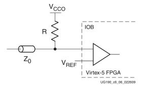
Figure 6-8: Input Termination to V<sub>CCO</sub> without DCI
