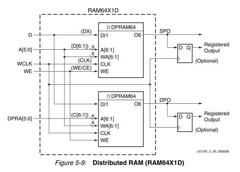
If two dual-port 64 x 1-bit modules are built, the two RAM64X1D primitives can occupy a SLICEM, as long as they share the same clock, write enable, and shared read and write port address inputs. This configuration equates to 64 x 2-bit dual-port distributed RAM.
