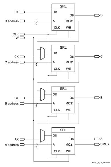
Figure 5-29: Simplified Virtex-5 FPGA Slice SRL
