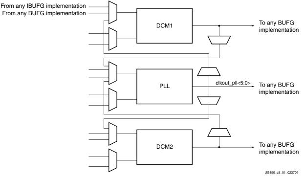
Figure 3-1: Block Diagram of the Virtex-5 FPGA CMT
