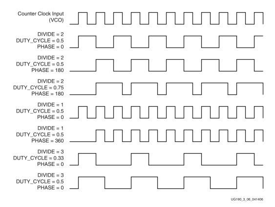
Figure 3-6: Output Counter Clock Synthesis Examples
