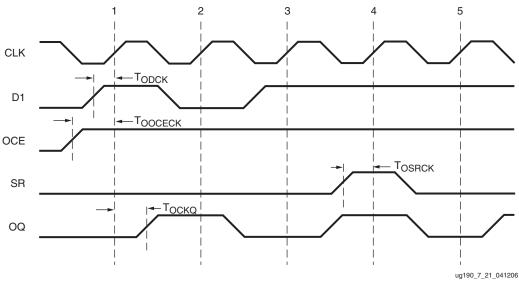
Figure 7-26: OLOGIC Output Register Timing Characteristics
