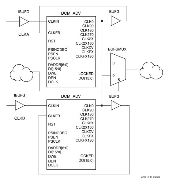
Figure 2-13: Clock Switching Between Two DCMs
