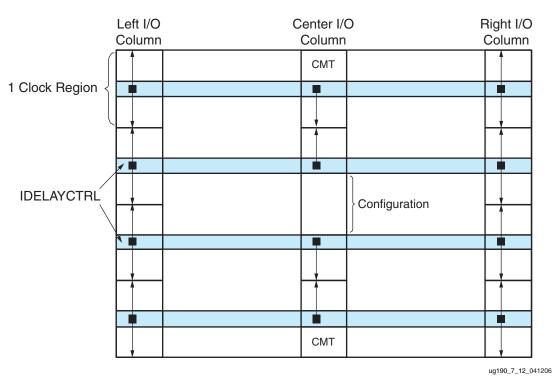
Figure 7-17: Relative Locations of IDELAYCTRL Modules
