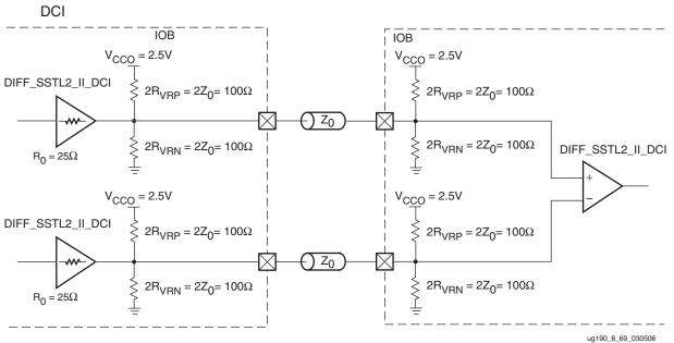
Figure 6-73 shows a sample circuit illustrating a valid termination technique for differential SSTL2 Class II (2.5V) with unidirectional DCI termination.
