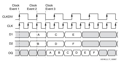
Figure 8-17: OSERDES Data Flow and Latency in 2:1 SDR Mode
