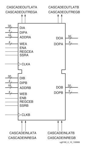
Figure 4-9 illustrates all the I/O ports of the 36 Kb true dual-port block RAM primitive (RAMB36). Table 4-5 lists these primitives.
