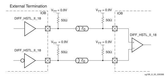
Figure 6-58: Differential HSTL (1.8V) Class II Unidirectional Termination
