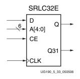
Figure 5-33: 32-bit Shift Register
