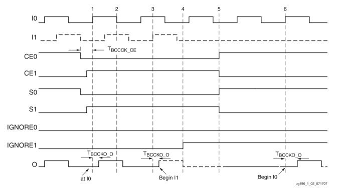
The timing diagram in Figure 1-2 illustrates various clock switching conditions using the BUFGCTRL primitives. Exact timing numbers are best found using the speed specification.
