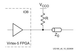
Figure 6-12: Driver with Termination to V<sub>CCO</sub> without DCI
