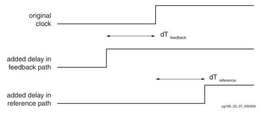
Figure 3-7: Basic Output Clock Shifting
