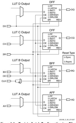
Figure 5-5: Register/Latch Configuration in a Slice
