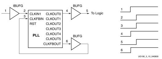
Figure 3-10: Clock Deskew Using Two BUFGs
