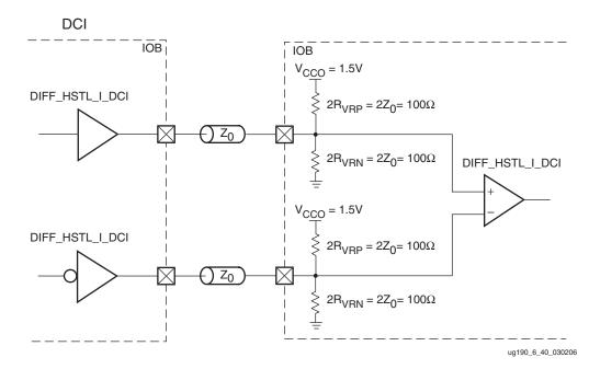
Figure 6-42: Differential HSTL (1.5V) Class I DCI Unidirectional Termination
