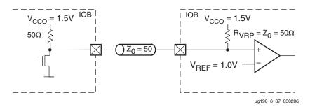
Figure 6-39: GTLP\_DCI Internal Parallel Driver and Receiver Termination
