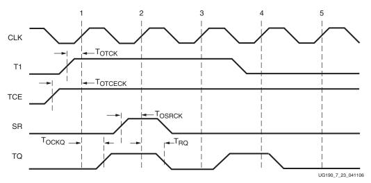
Figure 7-28: OLOGIC 3-State Register Timing Characteristics
