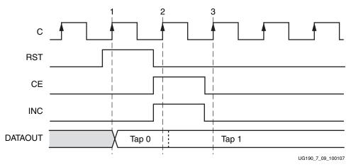
Figure 7-9: IDELAY Timing Diagram
