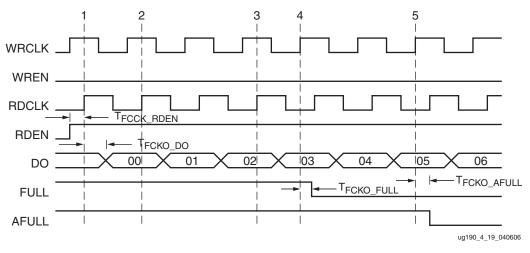
Figure 4-23: Reading From a Full FIFO
