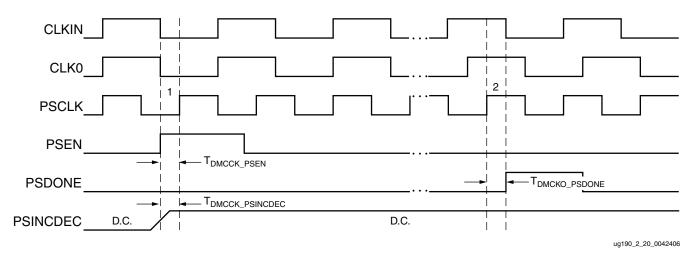
*Figure 2-19:* **Phase Shift Example: Variable**
