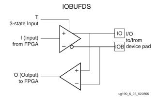
Figure 6-26 shows the differential input/output buffer primitive.
