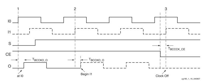
*Figure 1-16:* **BUFGMUX\_CTRL with a CE Timing Diagram**
