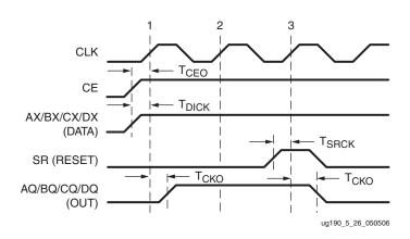
Figure 5-26: General Slice Timing Characteristics
