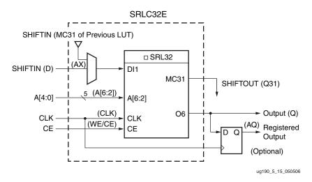
Figure 5-15: 32-bit Shift Register Configuration
