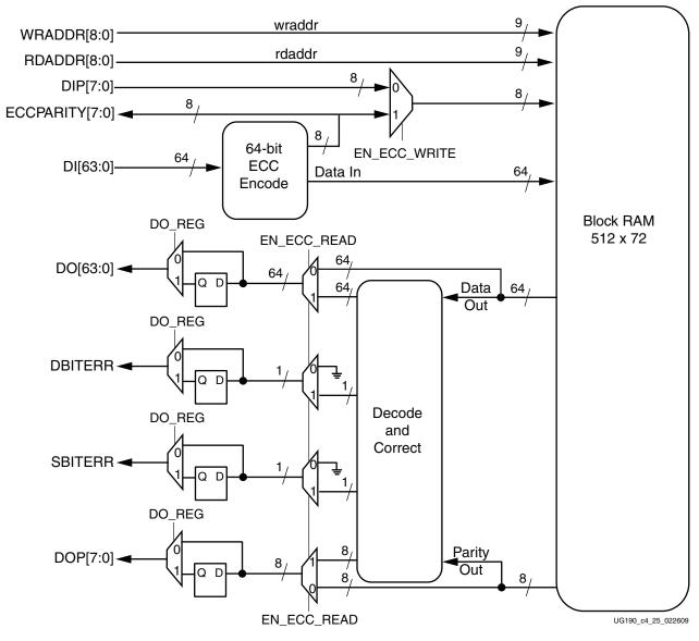
Figure 4-28: Top-Level View of Block RAM ECC
