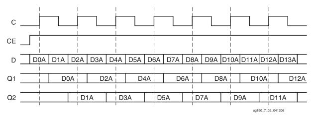
Figure 7-2: Input DDR Timing in OPPOSITE\_EDGE Mode
