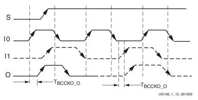
Figure 1-12: BUFGMUX\_CTRL Timing Diagram
