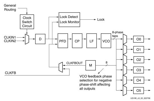
Figure 3-3: Detailed PLL Block Diagram
