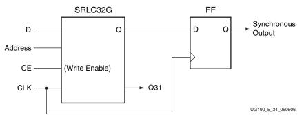
Figure 5-34: Synchronous Shift Register
