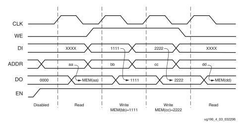
Figure 4-2: WRITE\_FIRST Mode Waveforms
