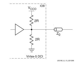
Figure 6-15 illustrates a driver with split termination inside a Virtex-5 device.
