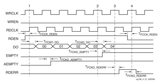
Figure 4-24: Reading From an Empty / Almost Empty FIFO (Standard Mode)
