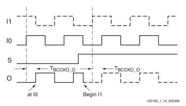
*Figure 1-14:* Asynchronous Mux Timing Diagram
