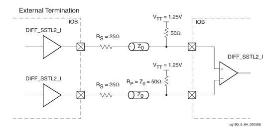
Figure 6-68: Differential SSTL2 Class I Unidirectional Termination
