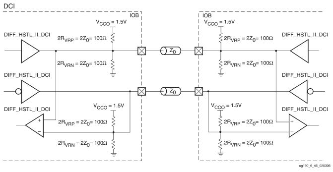
Figure 6-48 shows a sample circuit illustrating a valid termination technique for differential HSTL Class II (1.5V) with bidirectional DCI termination.
