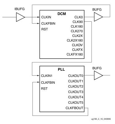
Figure 2-15: Direct Connection between DCM and PLL
