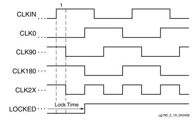
Figure 2-18: Phase Shift Example: Fixed
