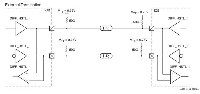
Figure 6-47: Differential HSTL (1.5V) Class II Bidirectional Termination
