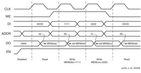
Figure 4-3: READ\_FIRST Mode Waveforms
