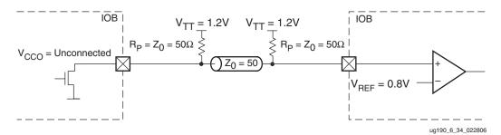
Figure 6-36: GTL with External Parallel Termination and Unconnected V<sub>CCO</sub>
