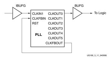
Figure 3-11: PLL with Internal Feedback
