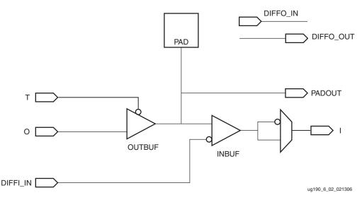
Figure 6-2: Basic IOB Diagram
