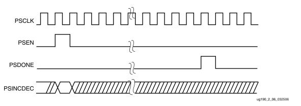
Figure 2-6: Phase-Shift Timing Diagram
