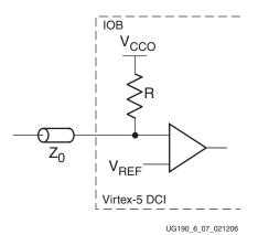
Figure 6-9: Input Termination Using DCI Single Termination
