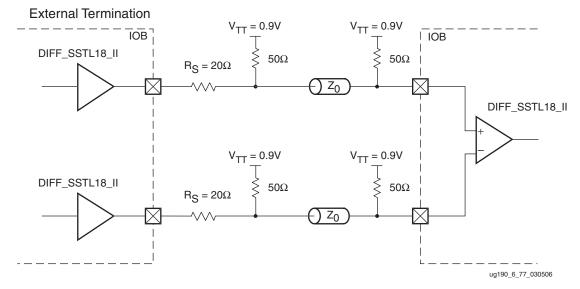
Figure 6-82: Differential SSTL (1.8V) Class II Unidirectional Termination
