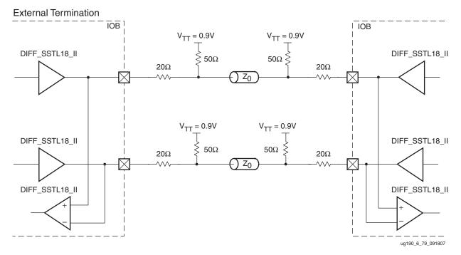
Figure 6-84 shows a sample circuit illustrating a valid termination technique for differential SSTL Class II (1.8V) with bidirectional termination.
