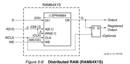
If four single-port 64 x 1-bit modules are built, the four RAM64X1S primitives can occupy a SLICEM, as long as they share the same clock, write enable, and shared read and write port address inputs. This configuration equates to 64 x 4-bit single-port distributed RAM.
