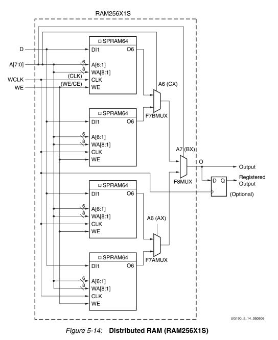
Distributed RAM configurations greater than the provided examples require more than one SLICEM. There are no direct connections between slices to form larger distributed RAM configurations within a CLB or between slices.
