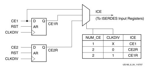
Figure 8-4: Input Clock Enable Module
