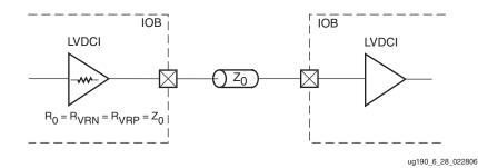
Figure 6-31: Controlled Impedance Driver with Unidirectional Termination
