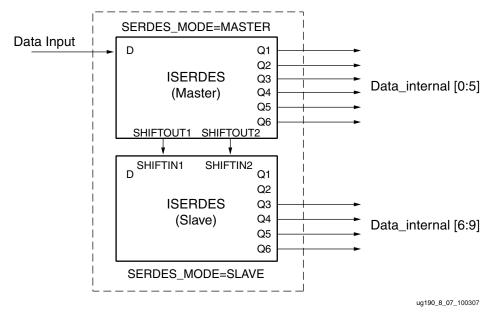
Figure 8-7: Block Diagram of ISERDES Width Expansion
