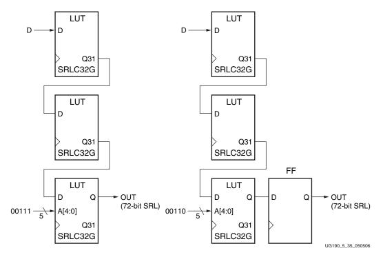
Figure 5-35: Example Static-Length Shift Register
