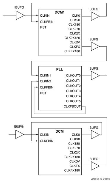
*Figure 2-16:* **Two DCMs Driving a PLL**
