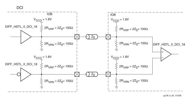
Figure 6-59 shows a sample circuit illustrating a valid termination technique for differential HSTL Class II (1.8V) with unidirectional DCI termination.
