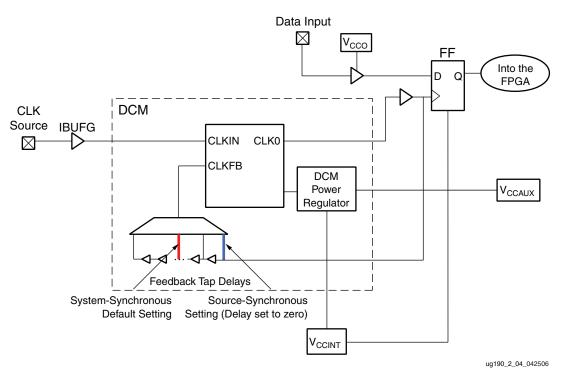
Figure 2-4: DCM and Feedback Tap-Delay Elements
