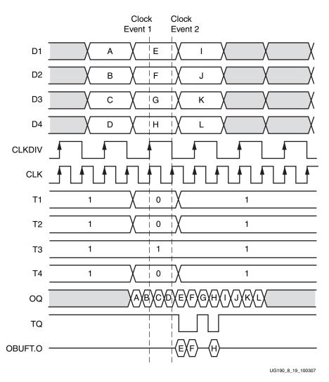
Figure 8-19: OSERDES Data Flow and Latency in 4:1 DDR Mode
