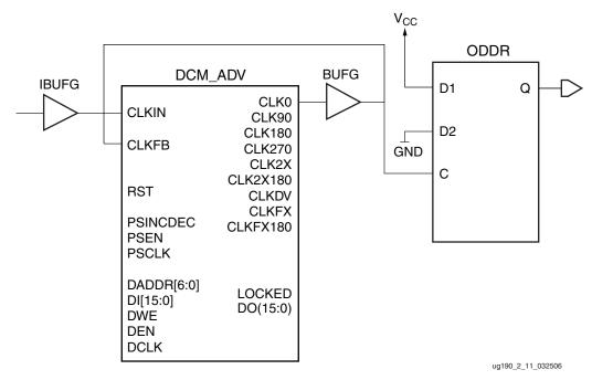
*Figure 2-10:* **Board-Level Clock with Internal Feedback**
