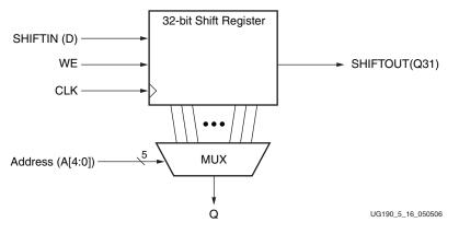
Figure 5-16: Representation of a Shift Register
