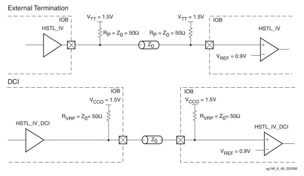
Figure 6-50: HSTL Class IV Unidirectional Termination
