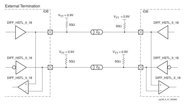
Figure 6-60: Differential HSTL (1.8V) Class II Bidirectional Termination
