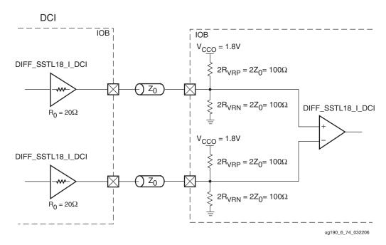
*Figure 6-79:* Differential SSTL (1.8V) Class I Unidirectional DCI Termination
