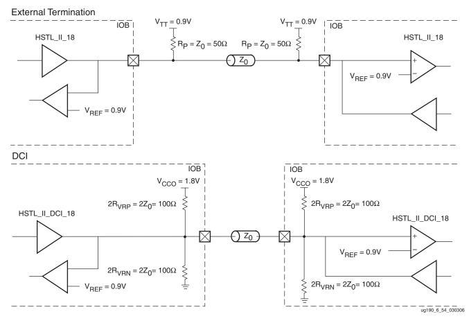
Figure 6-57: HSTL Class II (1.8V) with Bidirectional Termination
