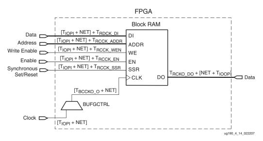
Figure 4-15: Block RAM Timing Model
