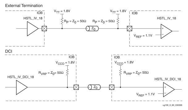
Figure 6-63: HSTL Class IV (1.8V) with Unidirectional Termination
