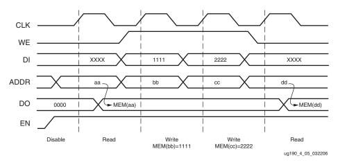
Figure 4-4: NO\_CHANGE Mode Waveforms
