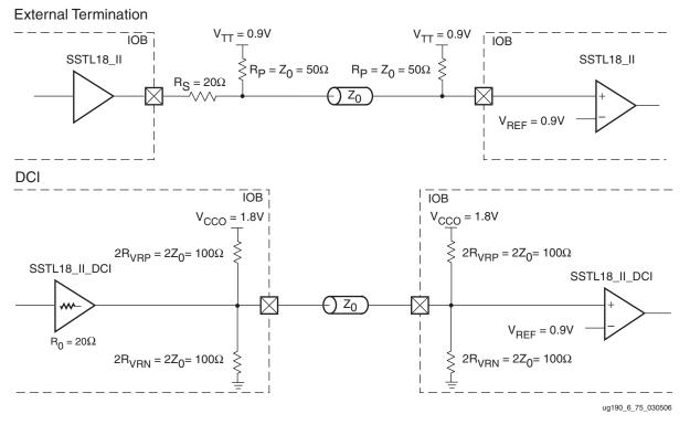
Figure 6-80: SSTL18 (1.8V) Class II Unidirectional Termination
