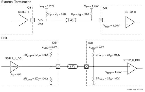
Figure 6-70: SSTL2 Class II with Unidirectional Termination
