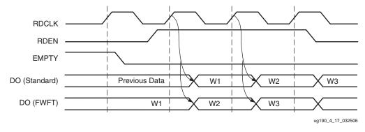
Figure 4-20: Read Cycle Timing (Standard and FWFT Modes)
