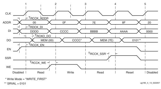
Figure 4-14: Block RAM Timing Diagram
