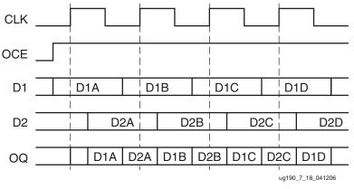
Figure 7-23: Output DDR Timing in OPPOSITE\_EDGE Mode
