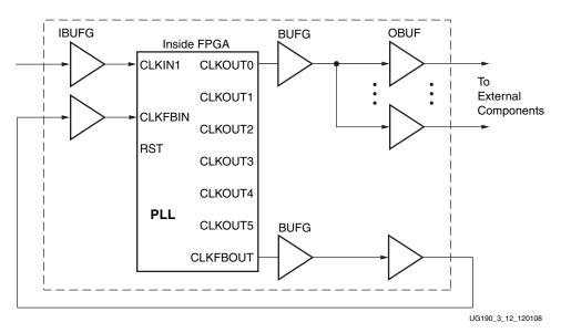
Figure 3-12: Zero Delay Buffer
