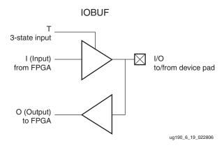
Figure 6-21: Input/Output Buffer (IOBUF) Primitive
