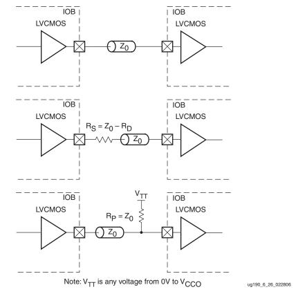
Figure 6-29: LVCMOS Unidirectional Termination
