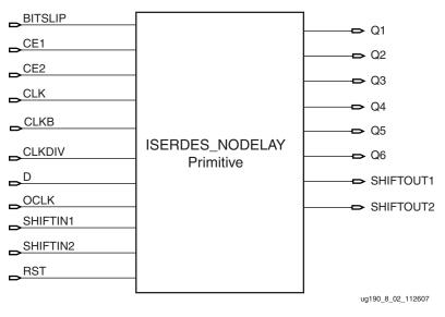
Figure 8-2: ISERDES\_NODELAY Primitive
