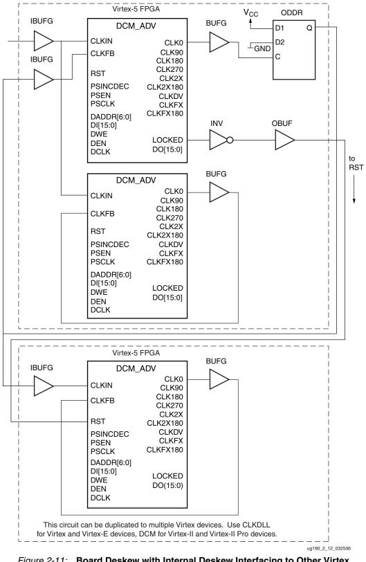
Figure 2-11: Board Deskew with Internal Deskew Interfacing to Other Virtex Devices
