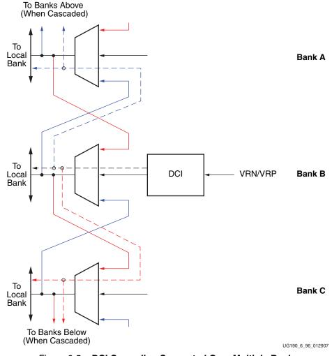
Figure 6-5: DCI Cascading Supported Over Multiple Banks
