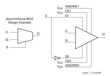
Figure 1-13: Asynchronous Mux with BUFGCTRL Design Example
